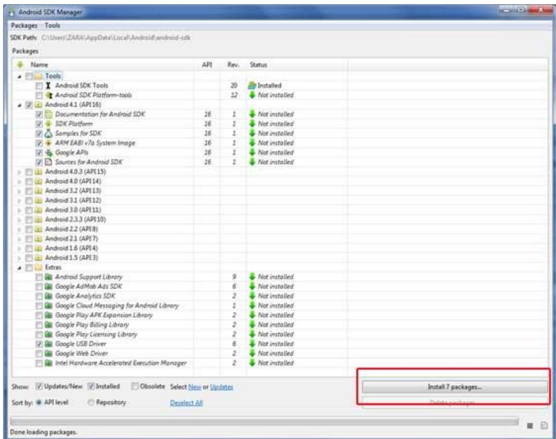
Once you launched SDK manager, its time to install other required packages. By default it will list down total 7 packages to be installed, but I will suggest to de-select *Documentation for Android SDK* and *Samples for*
