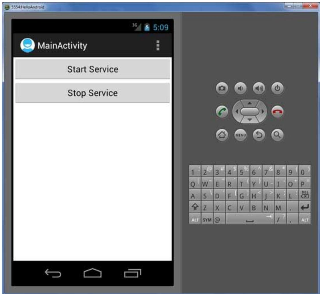
Now to start your service, let's click on **Start Service** button, this will start the service and as per our programming in `onStartCommand()` method, a message *Service Started* will appear on the bottom of the the simulator as follows:
