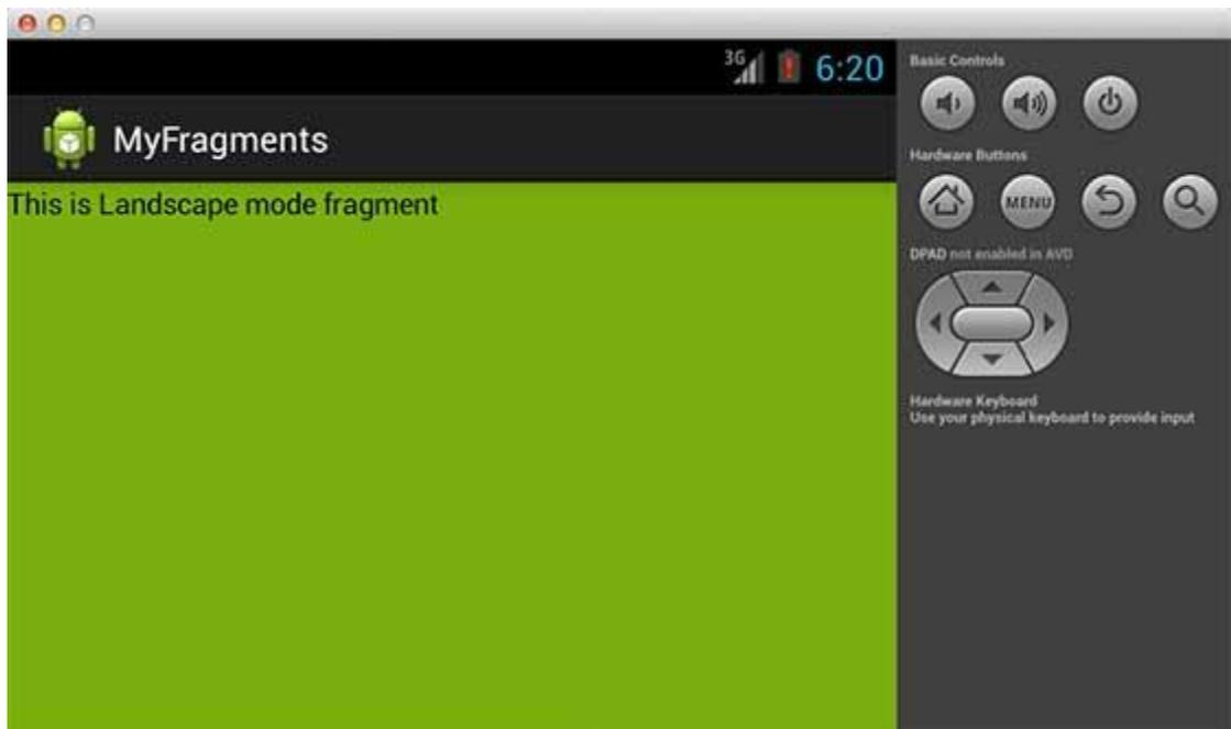
This way you can use same activity but different GUIs through different fragments. You can use different type of GUI components for different GUIs based on your requirements.
