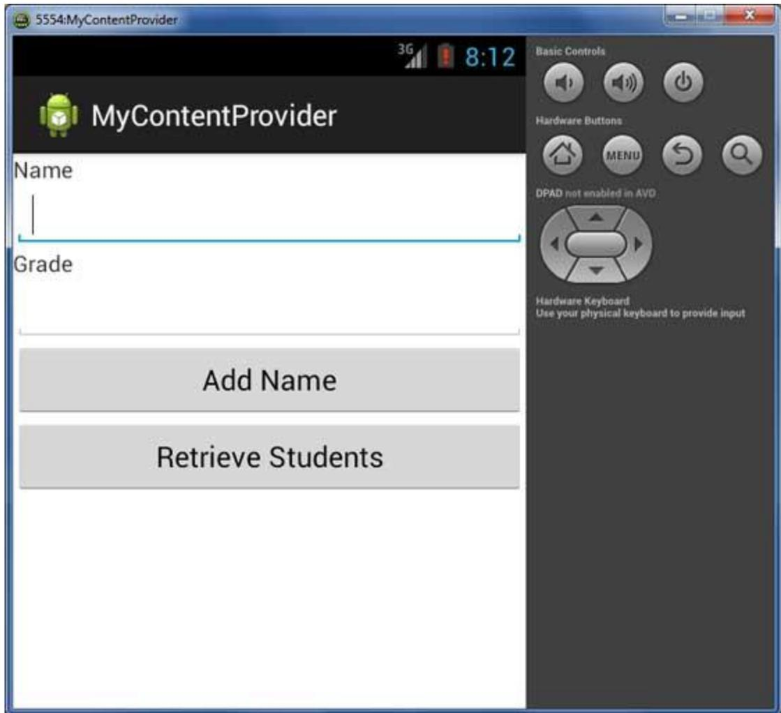
Now let's enter student **Name** and **Grade** and finally click on **Add Name** button, this will add student record in the database and will flash a message at the bottom showing ContentProvider URI along with record number added in the database. This operation makes use of our **insert()** method. Let's repeat this process to add few more students in the database of our content provider.
