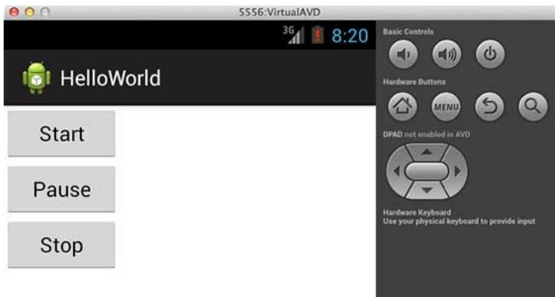
Now let's change the orientation of Layout as **android:orientation="horizontal"** and try to run the same application, it will give following screen:
