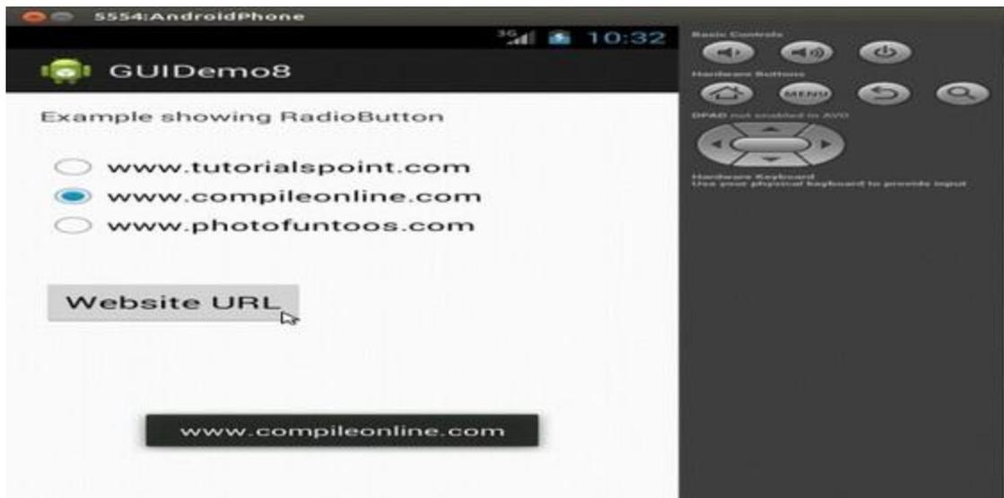
The following screen will appear when 3rd radiobutton is checked and text "www.photofuntoos.com" is shown when Button is clicked:
