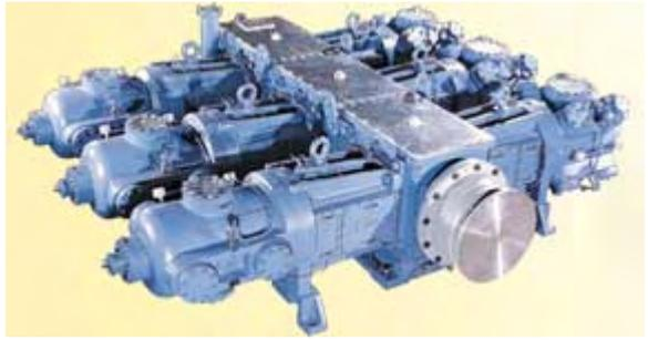
power) with pressure up to 5MPa (500 bars). Used for lower capacity gas compression and high reservoir pressure gas injection. *Photo: Ariel corp.*
