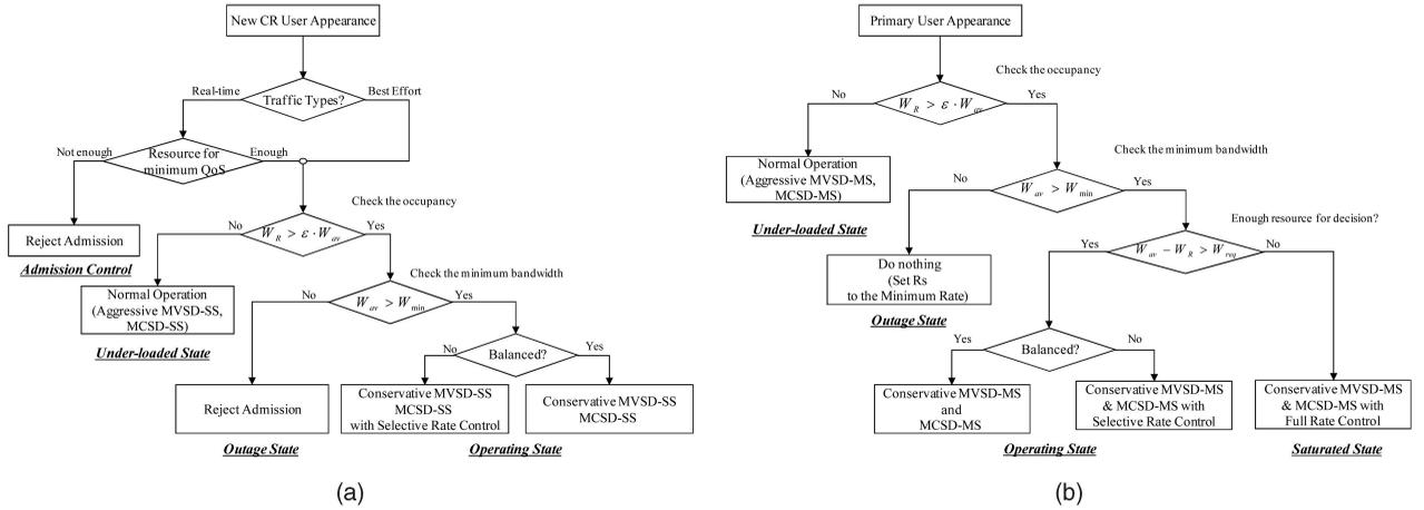
Fig. 6. The flowchart for the proposed decision control: (a) CR user appearance, and (b) primary user appearance.
