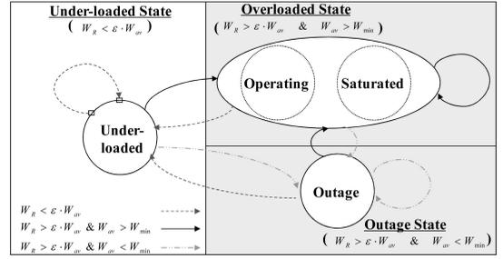
Fig. 5. The state diagram for resource management.
