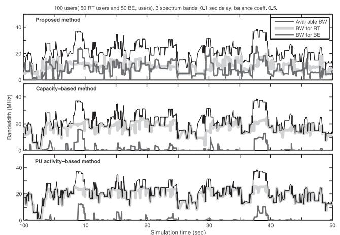
Fig. 10. Bandwidth utilization in the hybrid scenario.
