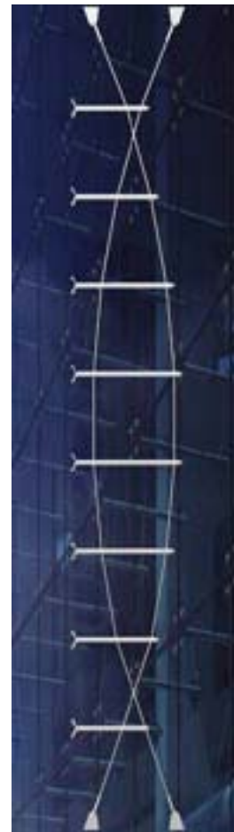
Figure 6.6 Typical cable truss design.
