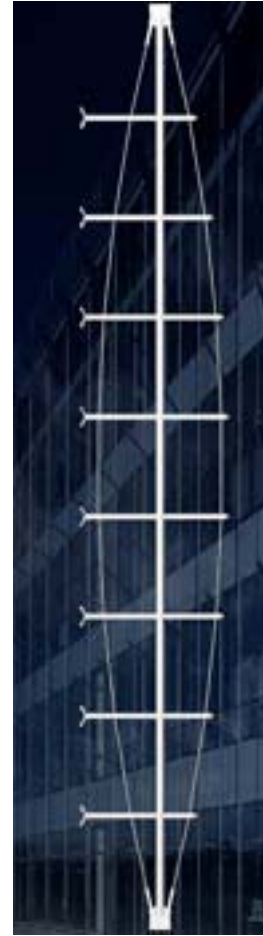
Figure 6.5 Mast truss cable-braced on two sides.
