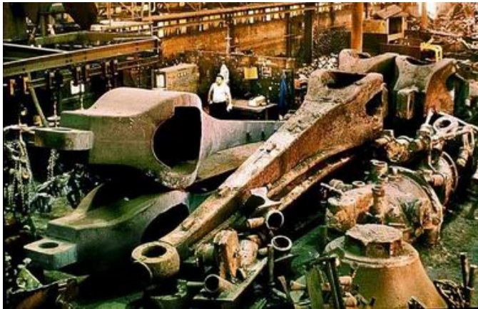
Figure 2.22 Center Pompidou, Paris; Rodgers and Piano architects, cast gerberettes on the production floor (Vincent n.d.).
