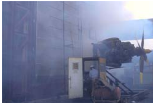
Figure 1.23 UBS Tower cable net facade; testing underway (ASIDI).
