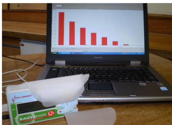
Above: Easysense Q datalogger and model clouds. The results show a gradual decrease in light intensity as each cloud layer is added.
