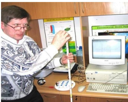
Fig. 15. Tadeusz Kubiak presents checking the dependence of magnetic induction on intensity of current flowing in the coil.
