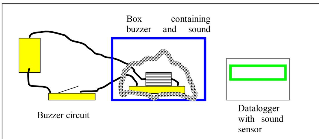
You can also set up the datalogger so that it takes a reading each time you tell it to. It will display the sound loudness on a computer screen as a bar chart.
