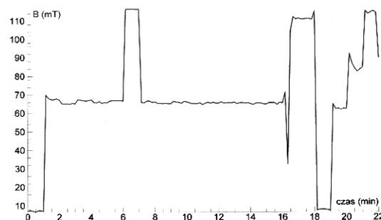
Fig. 18. The experimental results related to measurement of  $\mu$  for diamagnetic and ferromagnetic – cast iron and steel (7 and 18 min).
