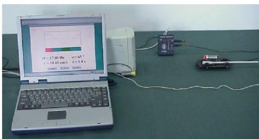
Fig. 9. A car with microphone and ultrasound receiver is moving with a speed  $v_o$  towards the loudspeaker and ultrasound transmitter, which are at rest on the table.
