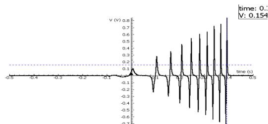
Fig. 16. On-line data and graphs illustrate change of induced potential in the plastic tube.
