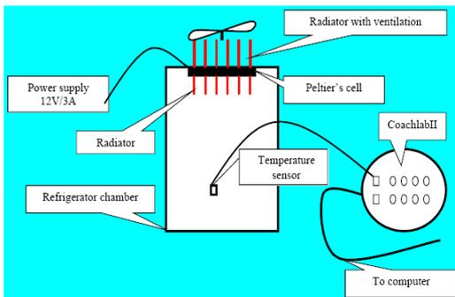
Fig. 13. The scheme of the Peltier's device.
