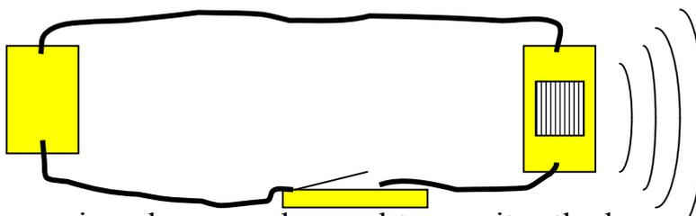
The datalogger microphone can be used to monitor the buzzer loudness in dB (decibels). The investigation invites learners to explore sound insulation by placing the buzzer in a box and investigating different types of sound insulation.
