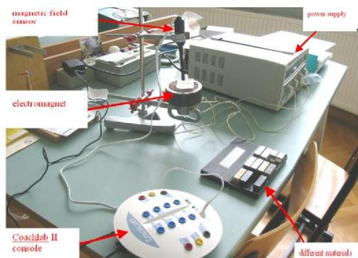
Fig. 17. The experimental set (designed by M. Kamiński) for measurement the permeability of different materials.
