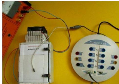
Fig. 14. The use of Peltier's cell for cooling.
