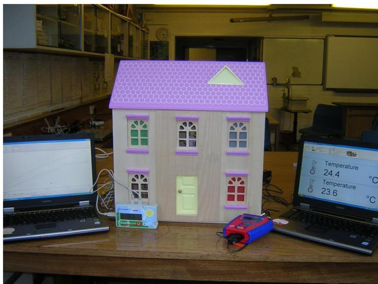
In the first experiment a night light candle is used as an energy source. [Warning: candles should not be left unattended or placed near flammable materials]. Temperature probes from the dataloggers are inserted through holes drilled in the back of the dolls house. The windows were sealed and the internal conditions were monitored over a period of ten minutes.
