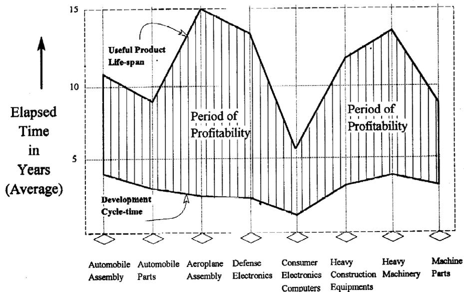
Fig. 2. Analysis of the average product development time (which indicates the start of the pay-off period) and of the product useful time (period of profitability) for various industrial products.
