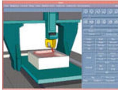
(H) Graphical simulation including the machine tool
