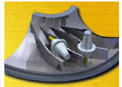
(F) Multi axis and multi spindle milling
