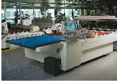
(G) An automatic machine for cutting the fabric
