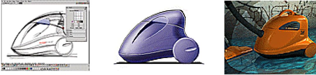
Fig. 7. (a) Sketch the product, (b) Colour and texture mapping, (c) Rendering of the 3D Model.
