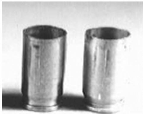
Figure 4.20 Scoop chamber marks on fired cartridge case.
