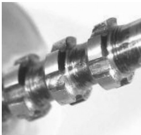
Figure 4.6 Broach rifling cutter.
