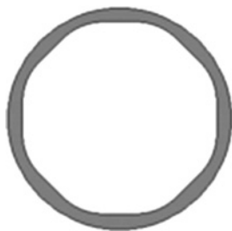
Figure 4.10 Conventional eight-groove rifling.
