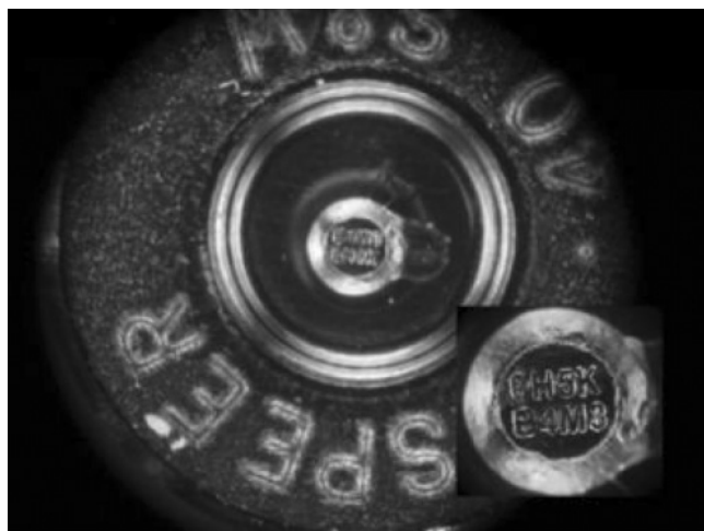
Figure 8.3 Firing pin impression with laser-etched serial number.
