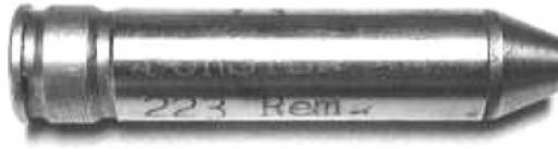
Figure 1.21 Rimless cartridge headspace gauge.
