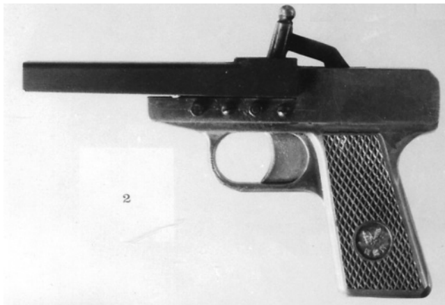
Figure 5.13 Converted, 0.22" calibre, muzzle-loading blank pistol.
