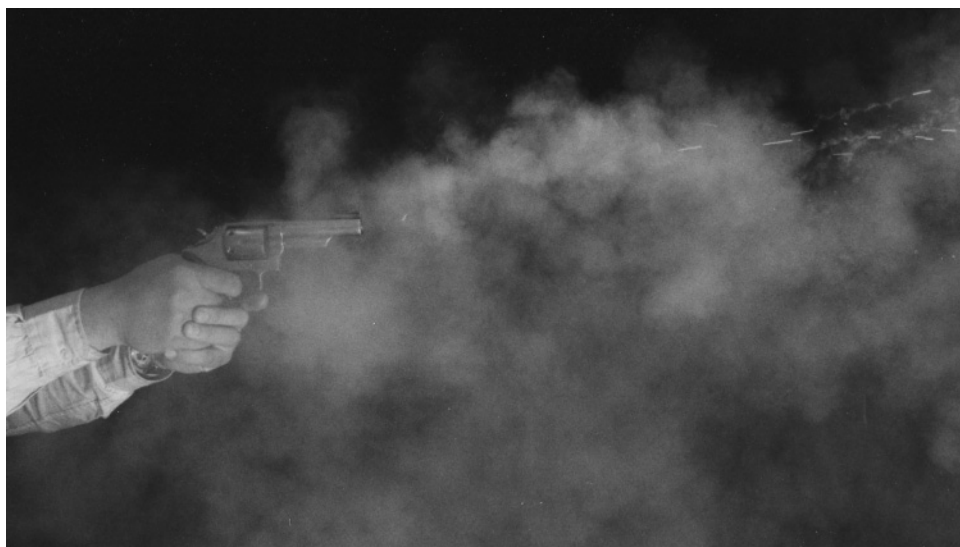
Figure 6.2 Photograph of discharge residue surrounding the hand during firing.
