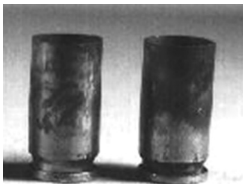
Figure 4.21 Helical chamber marks on fired cartridge case.
