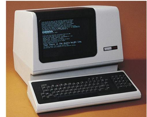
The VT100 was the first video terminal with microprocessor, and the first to implement the ANSI X3.64 (= ECMA-48) control functions. For instance, “`Esc[7m`” activates **inverse mode** and “`Esc[0m`” returns to normal, where `Esc` is the ASCII control character encoded by byte 27.
