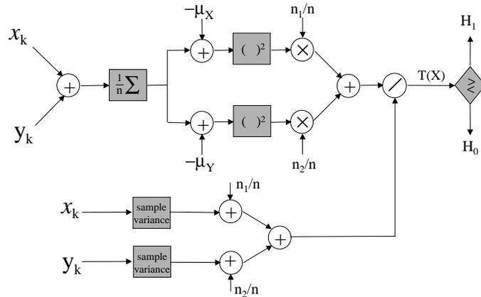
Figure 133: Block diagram of test of equality of means of two populations.
