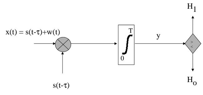
Figure 66: *SNR optimal receiver implemented as a correlator receiver for delayed signal in noise.*
