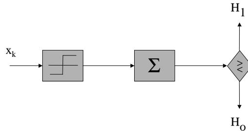
Figure 117: *LMP detector for testing positive mean  $\theta > 0$  for a Laplace r.v. is composed of a summer and memoryless non-linearity.*
