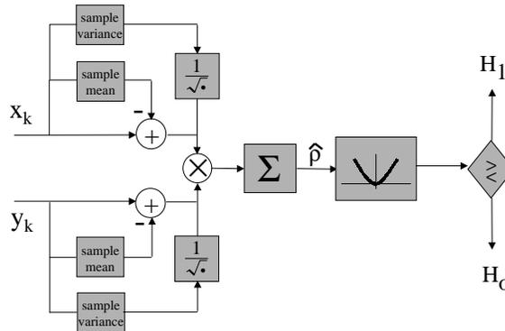
Figure 136: Block diagram of double sided test of nonzero correlation between two populations.
