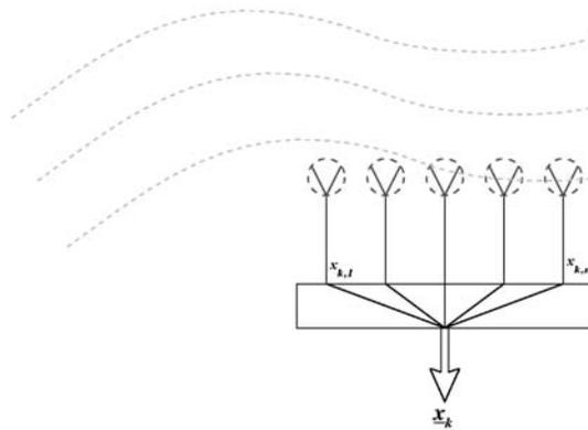
Figure 187: *Sensor array generates spatio-temporal measurement.*
