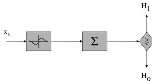
Figure 115: *Optimal detector for positive Cauchy median is a memoryless non-linearity followed by a summer and decision mechanism.*
