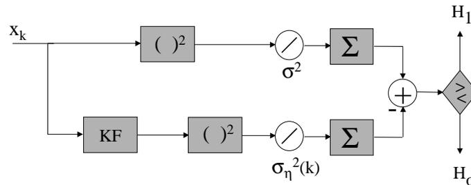
Figure 178: *The optimal detector of a single state space signal in noise.*
