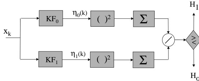
Figure 181: *GLRT signal selector for unknown measurement noise*
