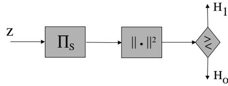
Figure 161: *GLRT detector block diagram implemented via signal subspace projection.*
