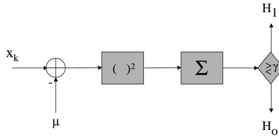
Figure 104: *Optimal detector for increase in Gaussian variance is a memoryless non-linear device (squarer) followed by a summer and decision mechanism. This detector has been called the square law detector and the energy detector.*
