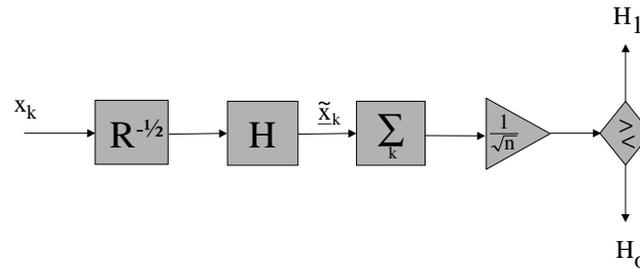
Figure 158: LRT for detecting presence of a spatio-temporal signal implemented with whitening and coordinate rotation preprocessing.
