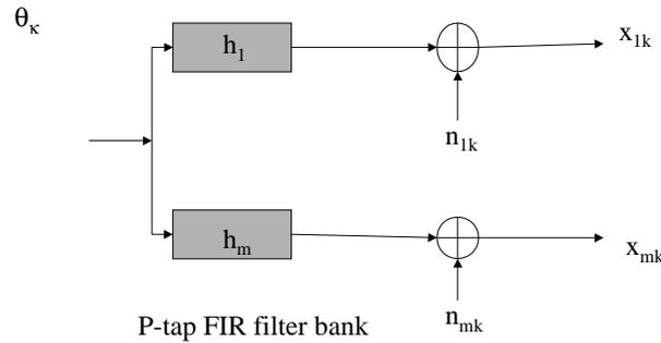
Figure 33: Block diagram for inverse problem
