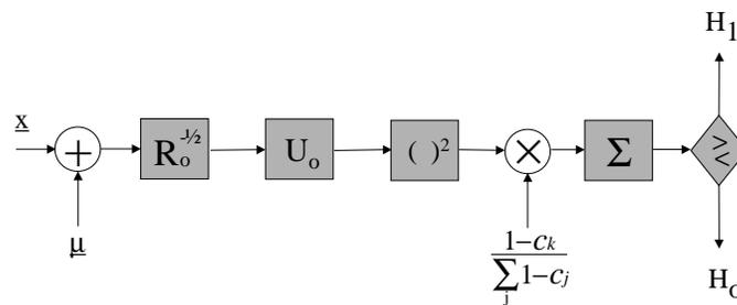
Figure 165: An implementation of the MP-LRT for equal means unequal covariances using orthogonal prefilter  $\mathbf{U}_0$  obtained from eigendecomposition:  $\mathbf{R}_0^{\frac{1}{2}}\mathbf{R}_1^{-1}\mathbf{R}_0^{\frac{1}{2}} = \mathbf{U}_0^T\mathbf{C}\mathbf{U}_0$ , where  $\mathbf{C}$  is diagonal.
