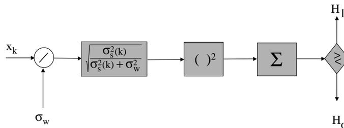
Figure 170: *Memoryless filter squarer implementation of LRT for non-stationary uncorrelated signal in white noise.*
