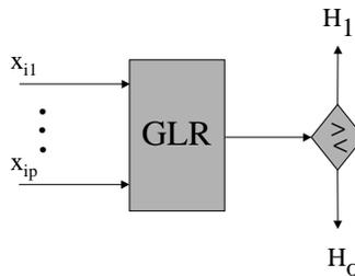
Figure 182: *GLR detector from multi-channel Gaussian measurements.*
