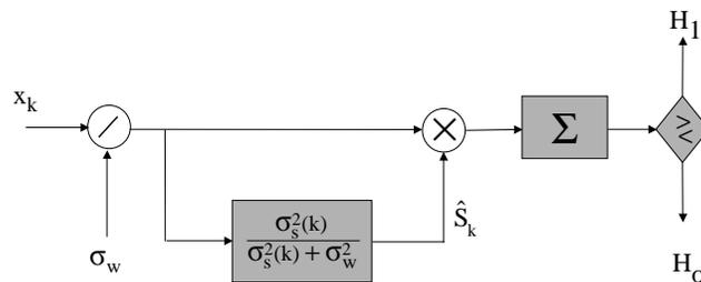
Figure 169: *Memoryless estimator correlator implementation of LRT for non-stationary uncorrelated signal in white noise. Note prewhitening operation  $1/\sigma_w^2$  precedes the estimator correlator.*
