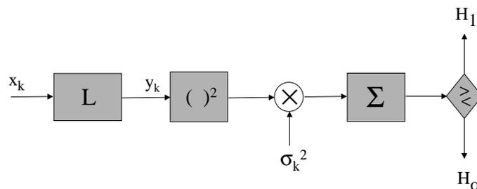
Figure 179: *On-line implementation of non-stationary signal detector via using Cholesky factor  $\mathbf{L}$ .*
