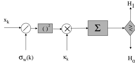
Figure 168: *LRT for detecting independent zero mean non-stationary Gaussian signal in non-stationary Gaussian noise.*
