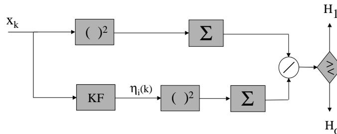
Figure 180: *Approximate steady-state GLRT signal detector for unknown measurement noise*
