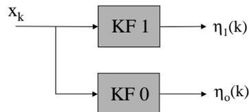
Figure 175: Dual Kalman filters generate innovations processes  $\eta_1$  and  $\eta_0$
