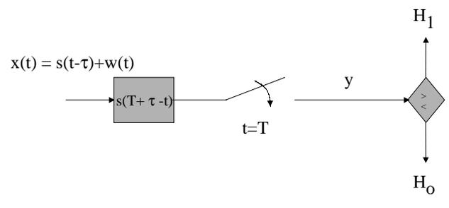
Figure 65: *SNR optimal receiver implemented as a matched filter receiver for delayed signal in noise.*
