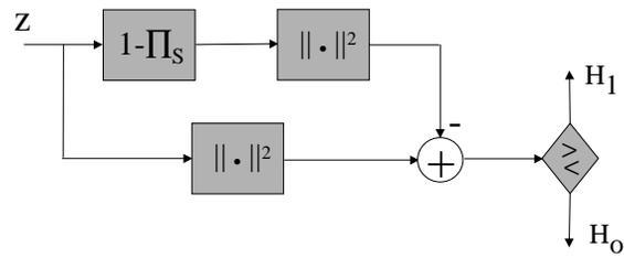
Figure 162: *GLRT detector block diagram implemented via noise subspace projection.*
