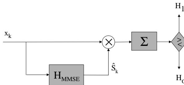
Figure 171: *Estimator correlator implementation of LRT for w.s.s. signal in white noise.*
