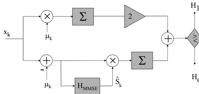
Figure 173: *Estimator correlator plus matched filter implementation of LRT for non-zero mean w.s.s. signal in white noise.*
