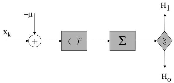
Figure 129: *GLRT for one sided test of positive shift in variance is an energy detector.*
