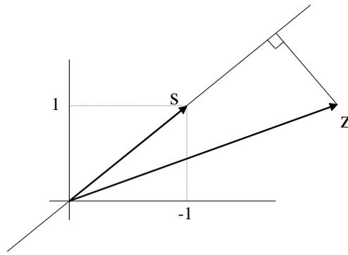
Figure 160: *GLRT detector thresholds length of orthogonal projection of  $\underline{z}$  onto  $\underline{s}$ , shown here for the case of  $n = 2$ .*
