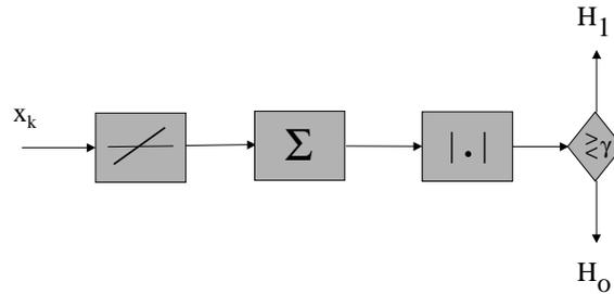
Figure 122: *Locally best unbiased double-sided test for non-zero Gaussian mean is a memoryless non-linearity followed by a summer and decision device.*
