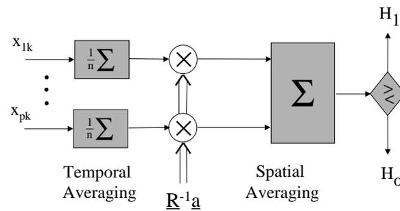
Figure 159: *LRT for detecting presence of a spatio-temporal signal implemented without coordinate transformation preprocessing.*
