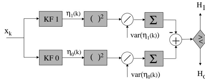
Figure 176: *Dual Kalman filter implementation of state space signal selector.*
