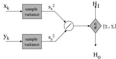
Figure 135: Block diagram of test of equality of two variances.
