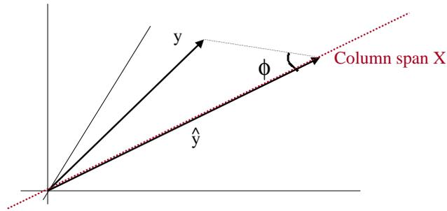
Figure 38: *Oblique projection interpretation of WLS estimator*
