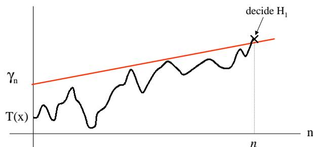
Figure 177: *Trajectory of dual Kalman filter implementation of state space signal selector. Note that the threshold is a function of time. If the number of samples  $n$  is random then the threshold of the test must be set by the method of repeated tests of significance.*
