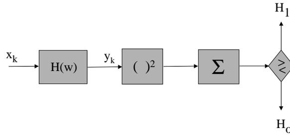
Figure 172: Filter squarer implementation of LRT for *w.s.s.* signal in white noise.
