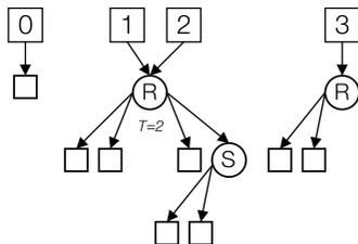
**Fig. 2.** Four snapshots in a Sarnak-Tarjan versioned-node tree, starting with an empty tree, then inserting  $R$ , then inserting  $S$ , then deleting  $S$ . We show the archived children to the left of a node and the current children to the right. Note that  $R$  is modified in-place for snapshot 2, but cloned for snapshot 3.
