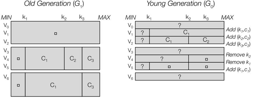
**Fig. 6.** Example of a PAD using speculation with an epoch of 3 snapshots. Lookups examine the young generation first. Because we did not use a circular ID-space the sentinel tuple in the young generation uses a key of ? to indicate that the older generation must be examined for  $k_q = k_{MIN}$ .
