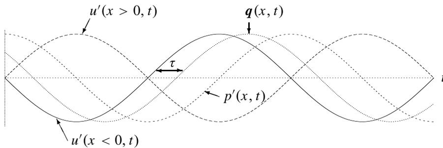
Figure 5.22 Sketch of time dependence of  $p'$  and  $u'$  in the upper ( $x > 0$ ) and lower ( $x < 0$ ) part of the tube. A memory effect of  $\frac{1}{2}\pi$  will shift the phase of the heat transfer  $\mathbf{q}$  from that of  $u'$  (the quasi-steady approximation) toward that of  $p'$ . It is the part of  $\mathbf{q}$  which is in phase with  $p'$  that produces the sound in a Rijke tube.
