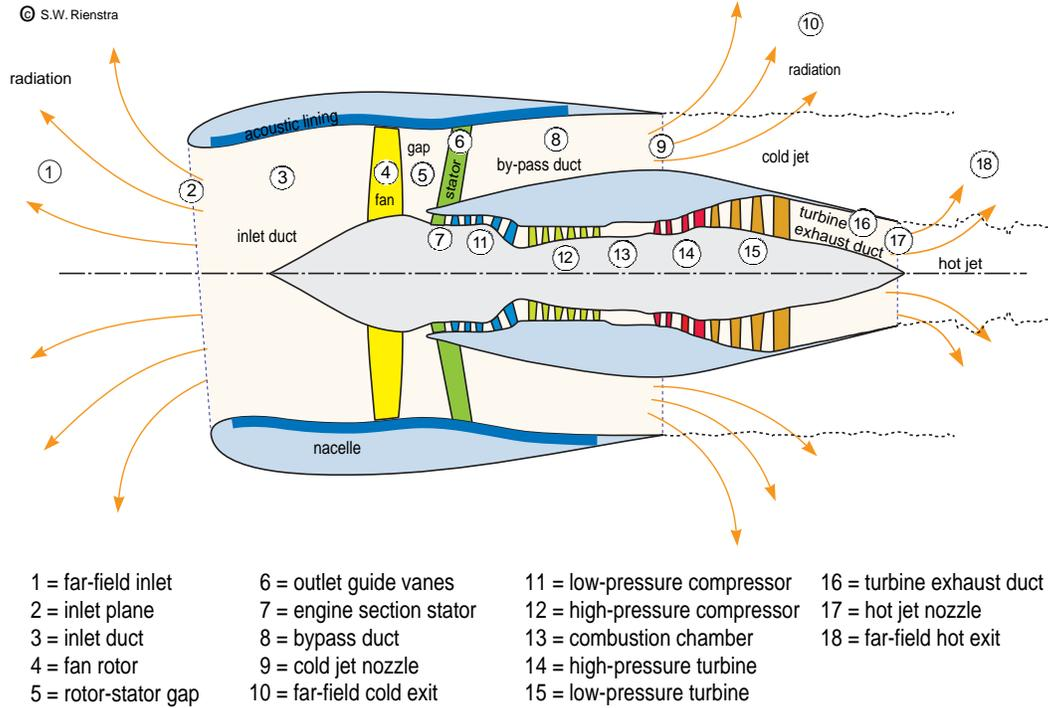
Figure 7.9 Sketch of high by-pass turbo fan engine. Note the fan (or inlet rotor), which produces with the stator (or outlet guide vanes) the important *rotor-stator interaction* noise. This is to be attenuated by the acoustically lined walls of the inlet and bypass duct.
