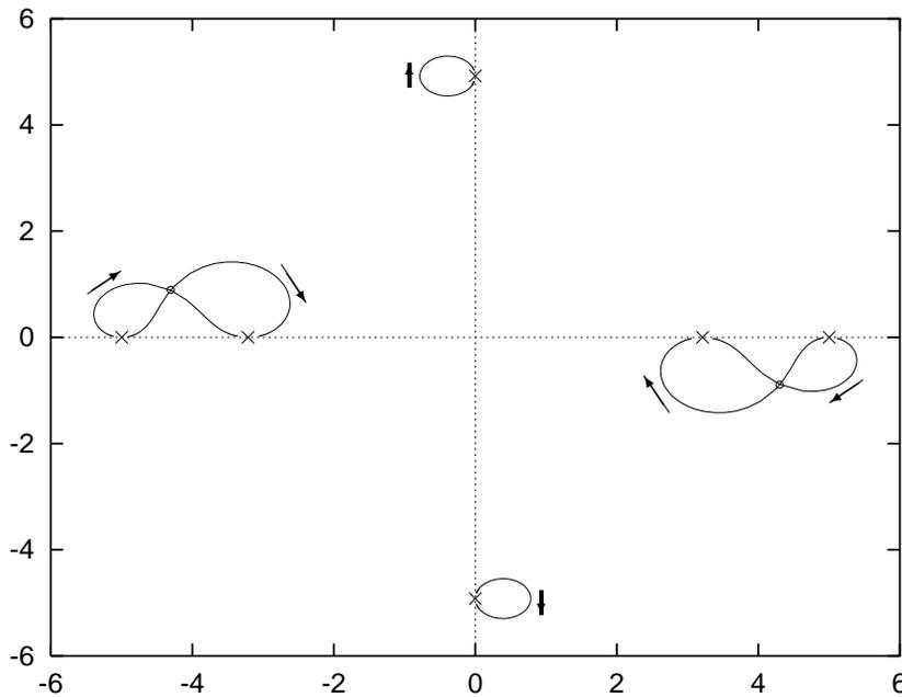
Figure 7.7 Trajectories of  $k_{m\mu}$  ( $m = 0, \omega = 5$ ) passing Cremer's optimum. At  $Z = (1.4165, -0.6082)$  the first two modes coalesce as  $k_{01}=k_{02}=(4.3057, -0.8857)$ .  $\text{Im}(Z)$  varies from  $-\infty$  to  $\infty$  and  $\text{Re}(Z)$  is fixed at 1.4165 .
