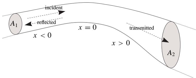
Figure 8.7 Duct junction.
