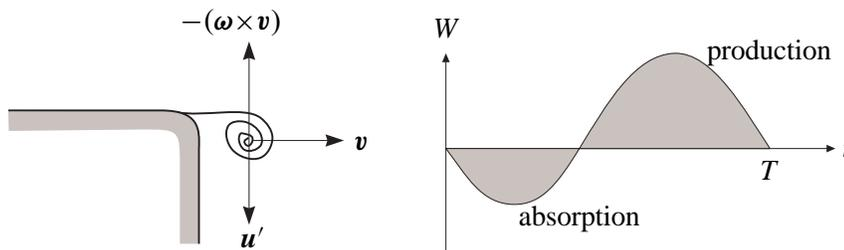
Figure 5.24 Absorption of acoustic energy by vortex shedding.
