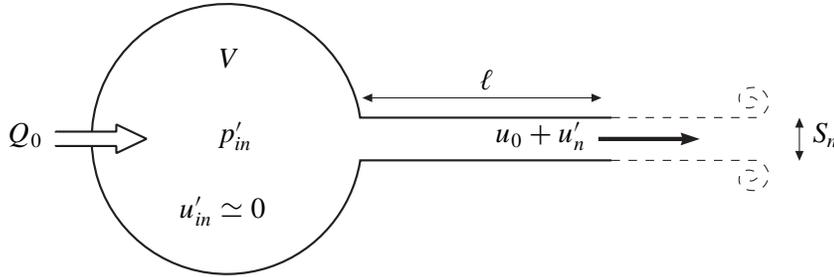
Figure 5.15 Helmholtz resonator with a mean flow.
