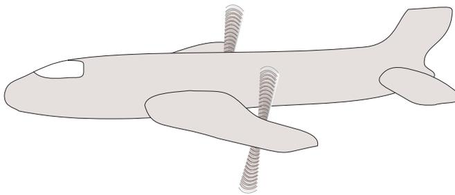
Figure 6.12 Propeller in pusher position (Exercise t)
