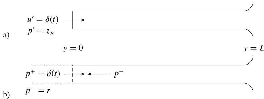
Figure 5.18 Difference between  $z_p$  and  $r$ .
