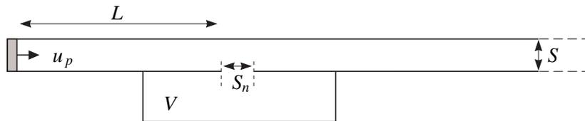
Figure 5.30 Helmholtz resonator driven by a piston.
