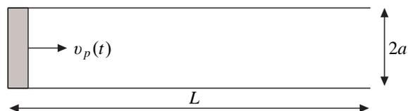
Figure 6.13 Piston in cylindrical pipe (Exercise x)
