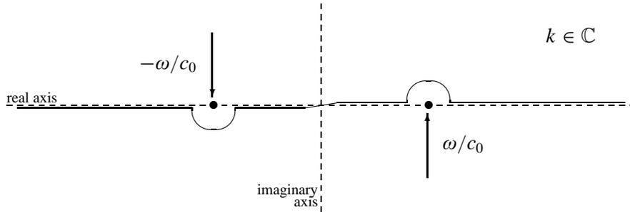
Figure C.2 Integration contour in complex  $k$ -plane. The arrows indicate the path of the poles  $\pm\omega/c_0$  in the  $k$ -plane, when  $\omega$  moves in its complex  $\omega$ -plane from the negative imaginary half onto the real axis, as  $\text{Im}(\omega) \uparrow 0$ .
