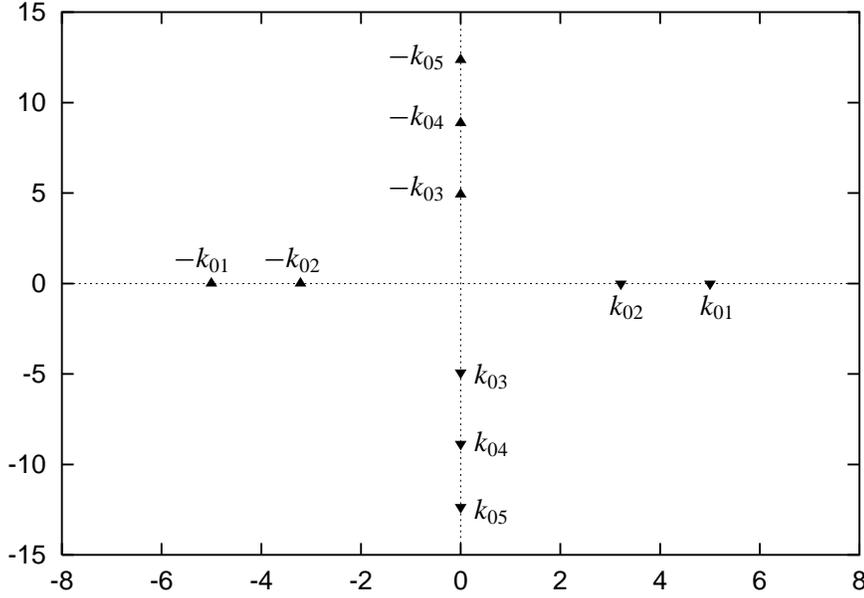
Figure 7.2 Complex axial wave numbers ( $m = 0$ ,  $\omega = 5$ ).
