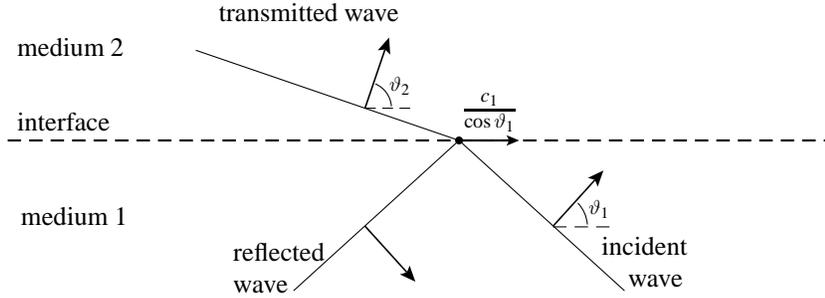
Figure 3.6 Reflection and transmission at a discontinuity.
