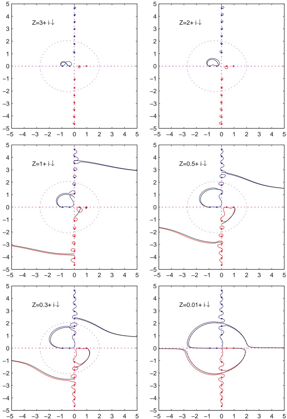
Figure 7.8 Trajectories of reduced wave number  $\sigma_{m\mu}$  ( $m = 1, \omega = 5$ ) where  $M = 0.5$ , for  $\text{Im}(Z)$  varying from  $-\infty$  to  $\infty$  and fixed  $\text{Re}(Z)$ . The 2D surface wave solutions of eqn. (3.47) are included as black lines.
