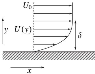
Figure 5.5 Boundary layer velocity profile.
