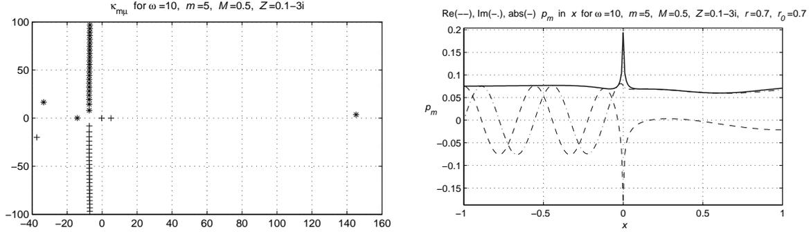
Figure 7.11 Eigenvalues  $\kappa_{m\mu}^{\pm}$  and  $\text{Re}(p_m)$ ,  $\text{Im}(p_m)$  and  $|p_m|$  is plotted of the  $m = 5$ -th component of the point source field in a lined flow duct with  $\omega = 10$ ,  $Z = 0.1 - 3i$ ,  $x_0 = 0$ ,  $r_0 = 0.7$ ,  $M = 0.5$  at  $r = 0.7$  and  $\theta = \theta_0$ . Note the presence of 3 surface waves.
