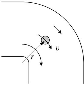
Figure 5.3 Frictionless flow in a bend.
