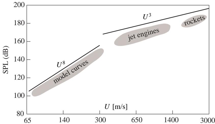
Figure 6.6 Sound power generated by a jet.
