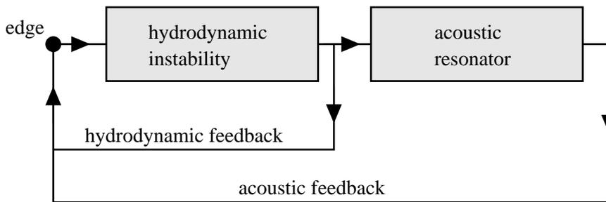
Figure 5.1 Flow-acoustic oscillator.
