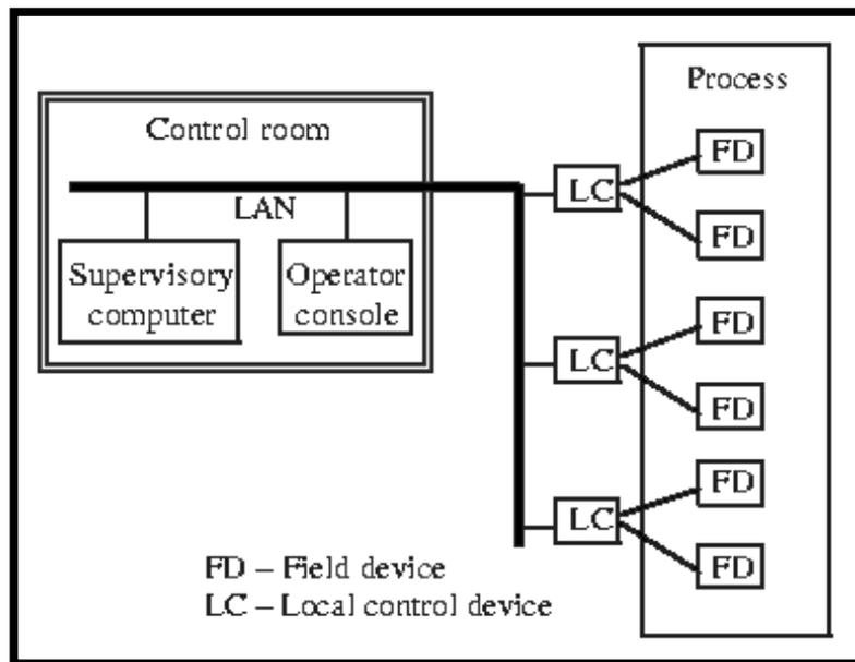
**Fig. 1.3.** A first approach towards a distributed architecture introduced in Process Control Systems after the mid 1970s.
