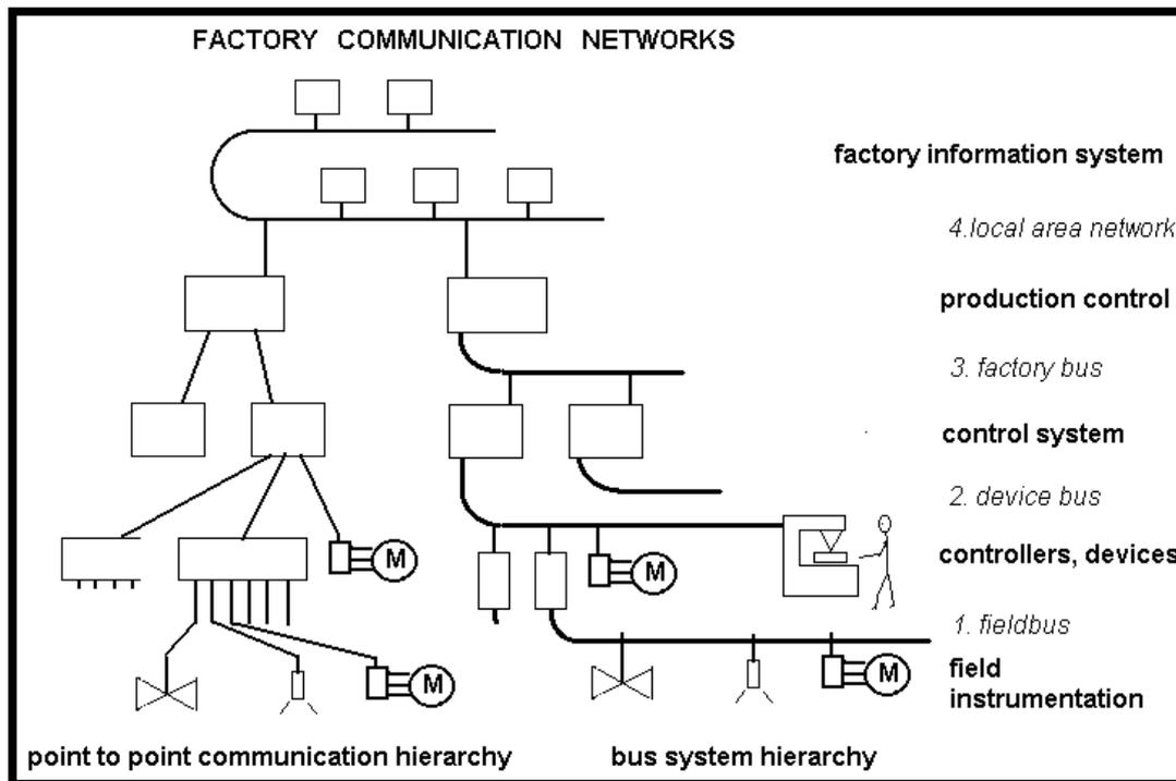
**Fig. 1.7.** Comparison between the point-to-point and the fieldbus Hierarchies.
