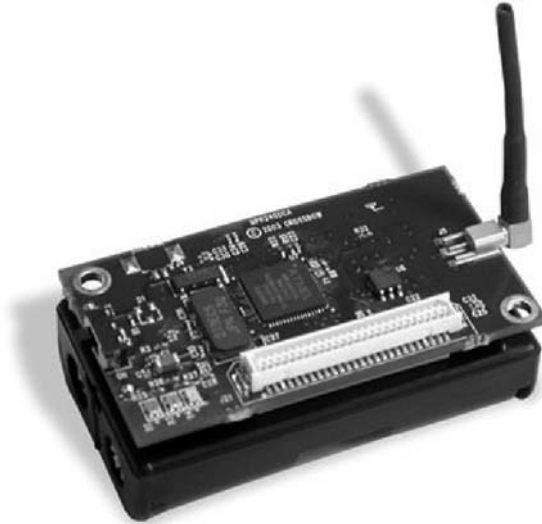
Figure 1.1 MICAz sensor mote hardware. (Image courtesy of Crossbow Technology [3].)
