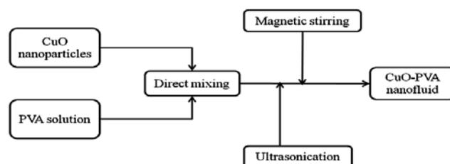
Figure 1. Preparation of CuO-PVA nanofluid
