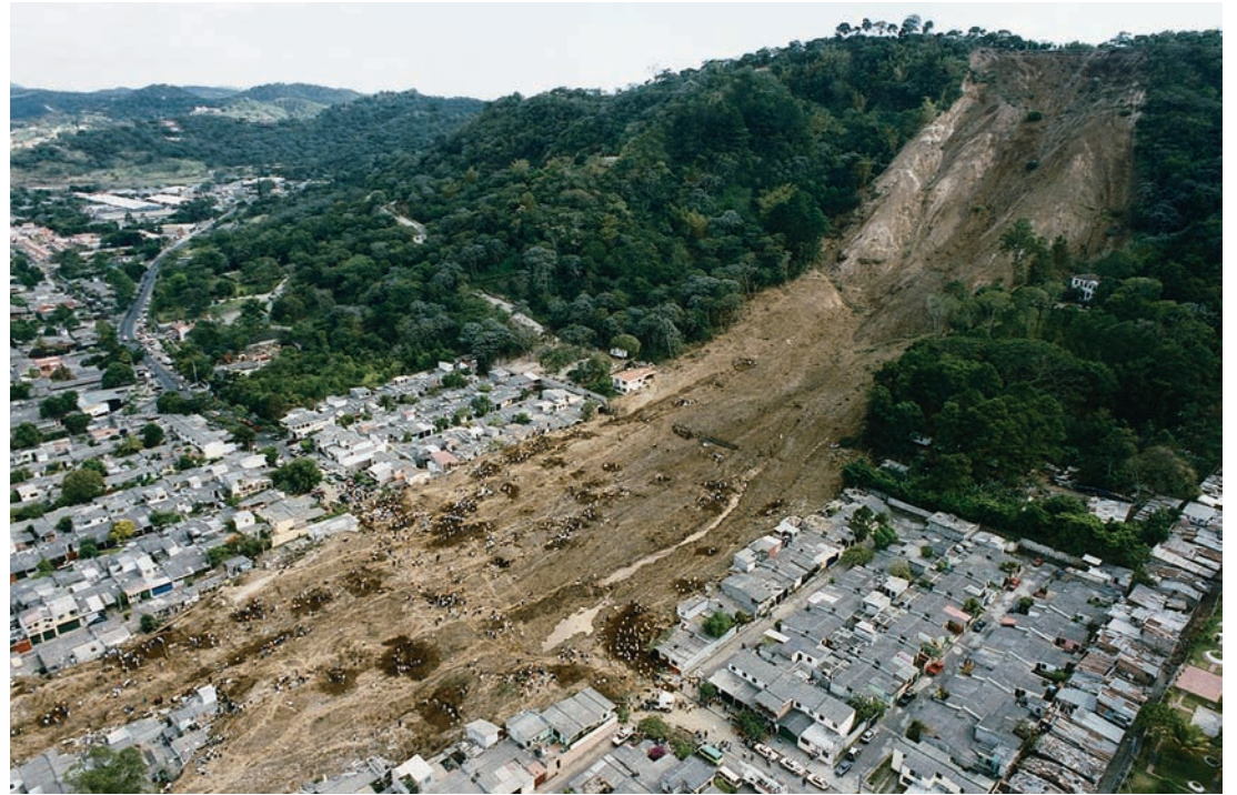
▲ Figure 1.2 On January 13, 2001, a magnitude 7.6 earthquake caused considerable damage in El Salvador. The damage pictured here was caused by a landslide that was triggered by the earthquake. As many as 1000 people were buried under 8 meters (26 feet) of landslide debris. Geologists seek to understand the processes that create such events. (Photo by Reuters/STR/Getty Images Inc.-Hulton Archive Photos)
