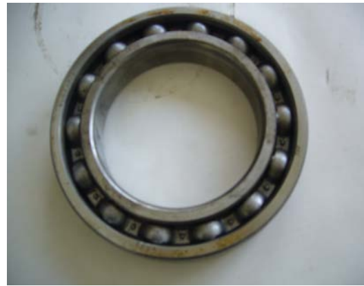
Figure 5. Main bearing in healthy condition
