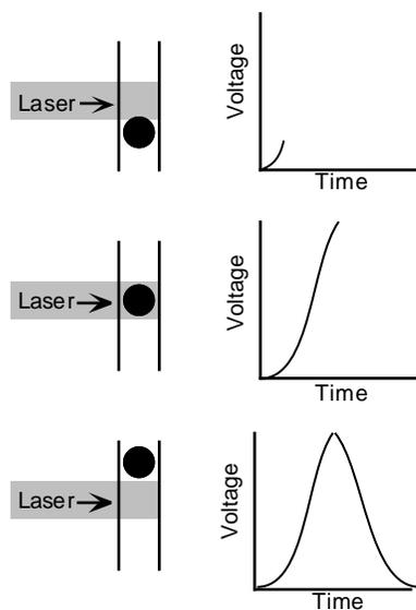
**Figure 4-5** Creation of a voltage pulse
