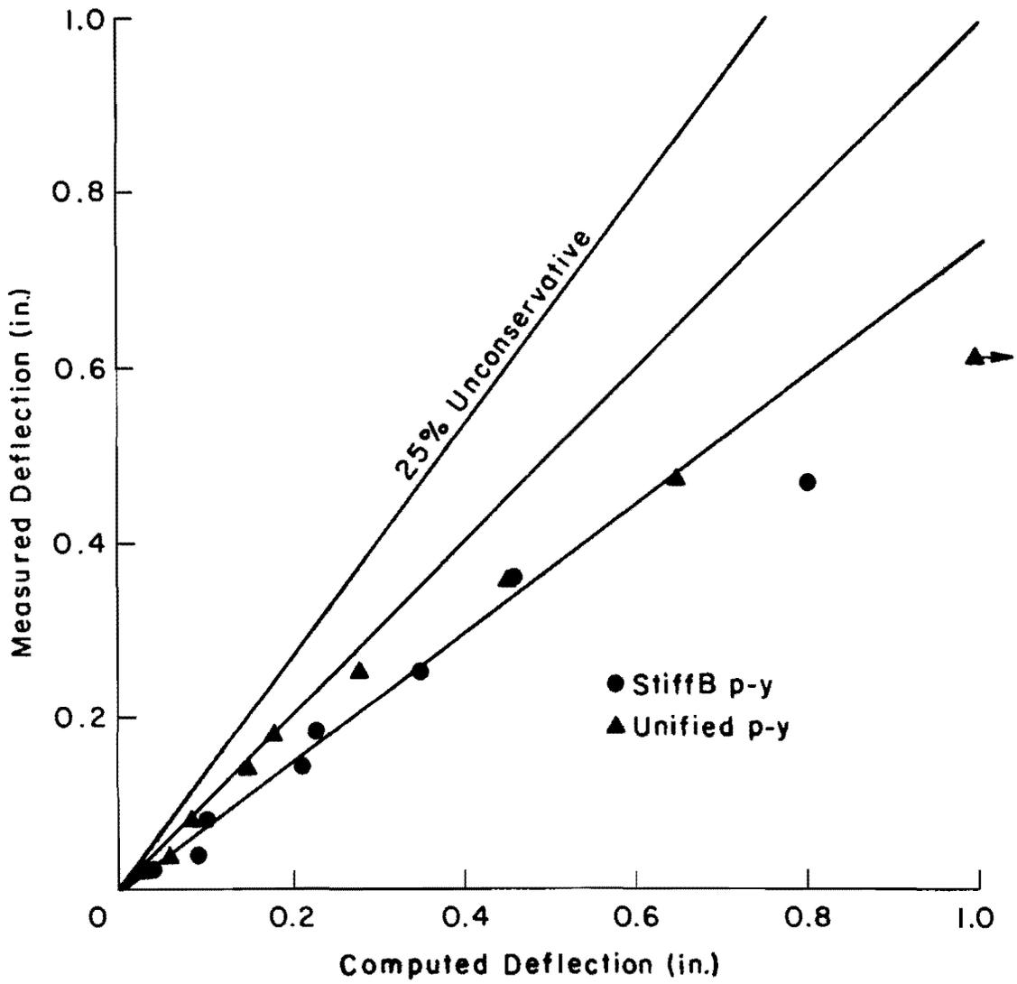
Fig. 4.30. Comparison between measured and computed deflections for tests using StiffA and Unified criteria.
