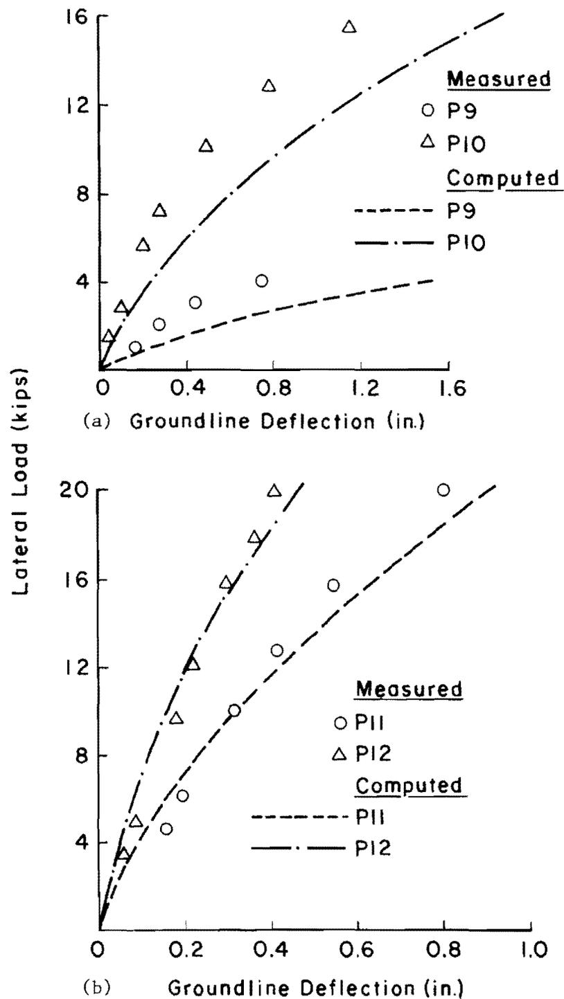
Fig. 5.24. Comparison of measured and computed deflections for tests in hydraulic fill. (a) test piles P9 and P10; (b) test piles P11 and P12.
