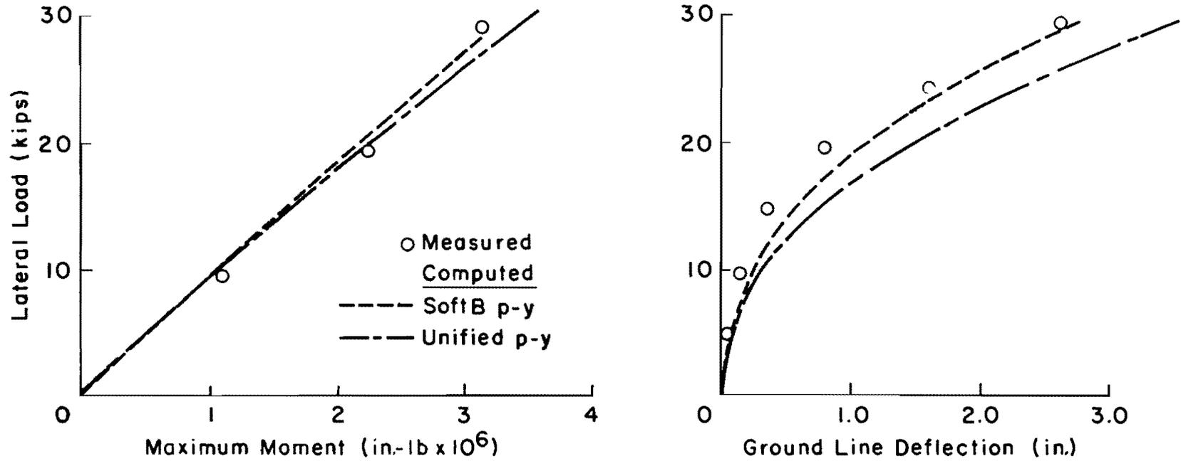
Fig. 4.18. Comparison between measured and computed results for test at Plancoet.
