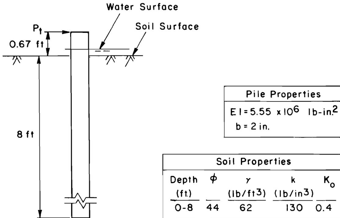
Fig. 5.27. Information for the analysis of model test at The University of Texas.
