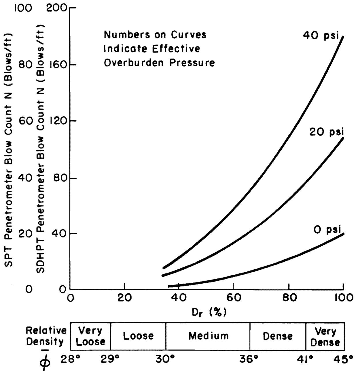
Fig. 5.2. Relation between SDHPT and SPT penetrometer blow count and the friction angle.
