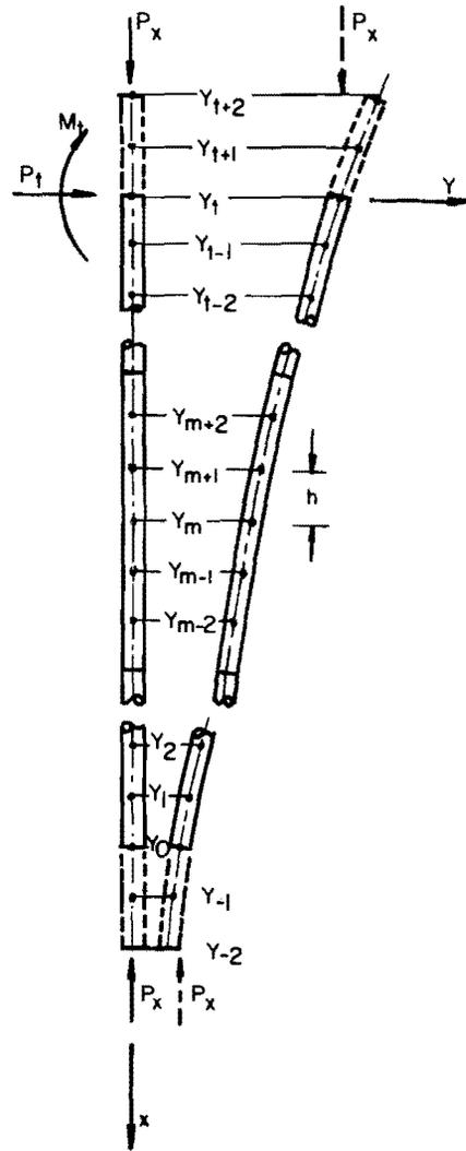
Fig. 1.6. Pile divided into increments.
