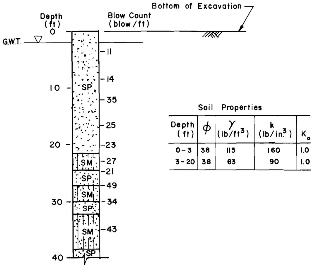
Fig. 5.5. Soils information for analysis of tests at Arkansas River.
