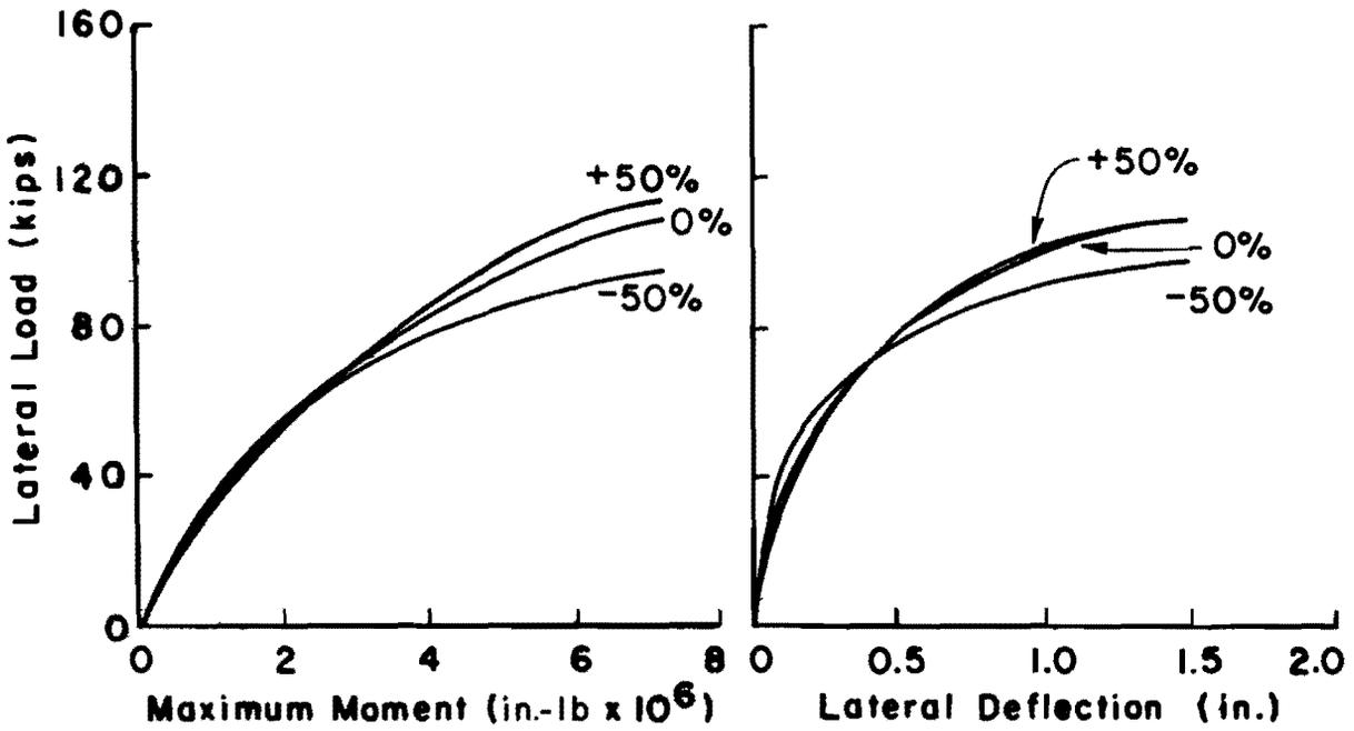
Fig. 3.7. Comparison between results for  $\pm 50\%$  variation in  $\epsilon_{50}$  using StiffB criteria for static loading.
