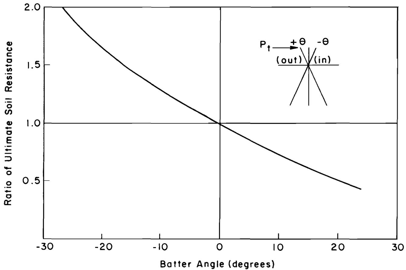
Fig. 5.15. Modification factors for sand p-y curves for battered piles (Kubo, 1962).
