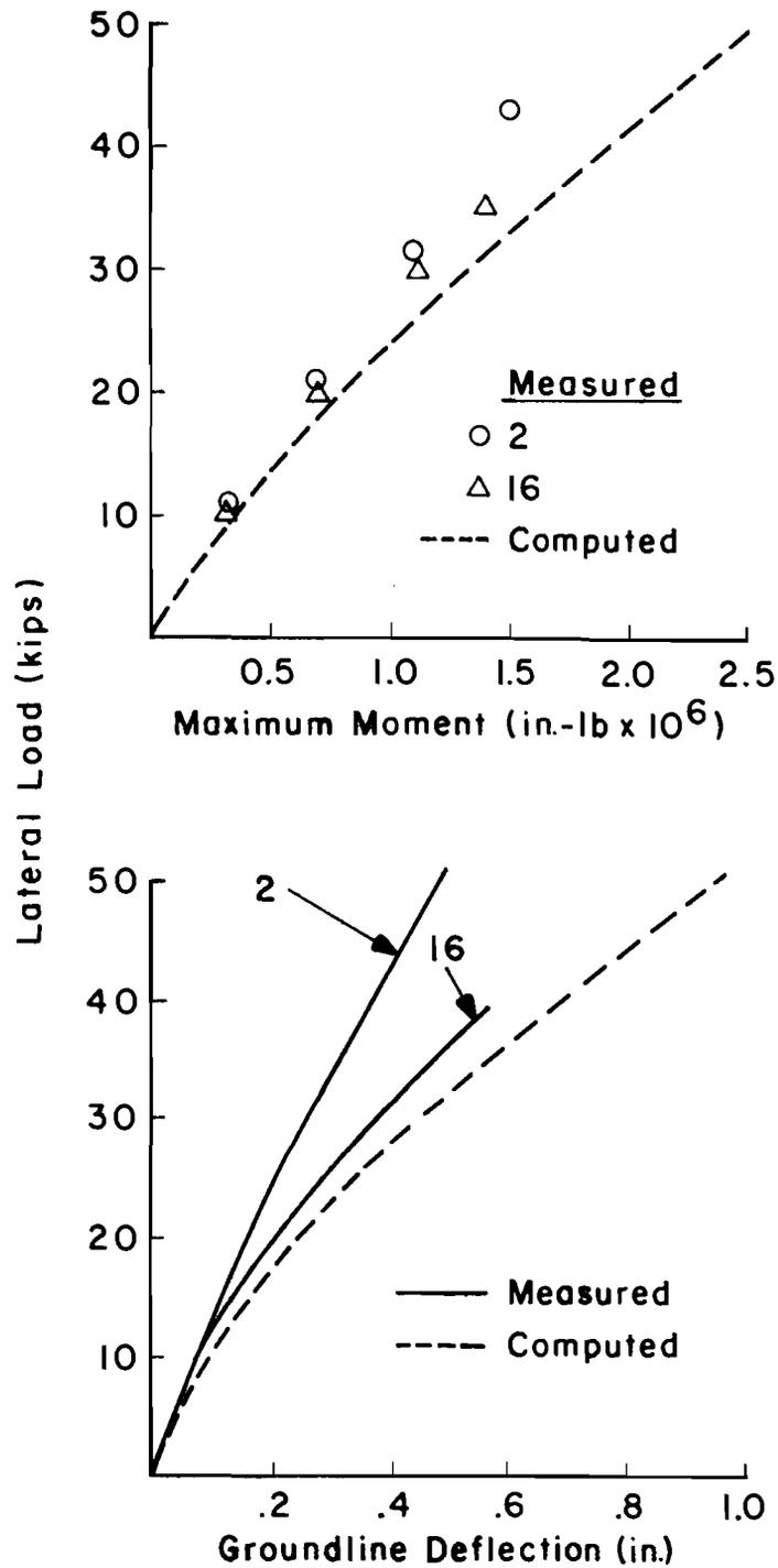
Fig. 5.7. Comparison between measured and computed results for test piles 2 and 16 at Arkansas River.
