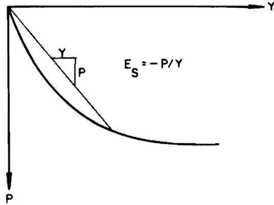
Fig. 1.5. Illustration of secant modulus.
