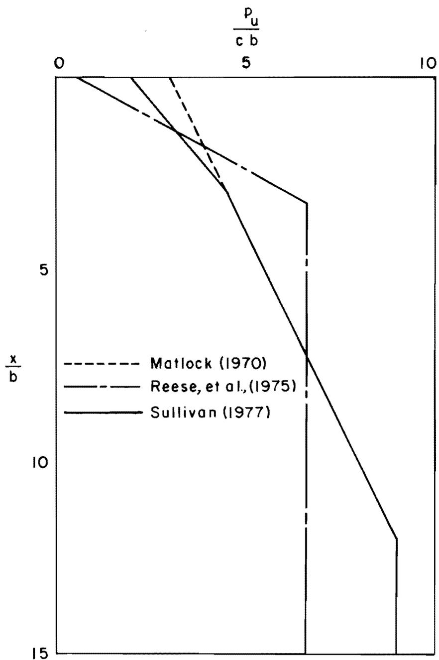
Fig. 2.5. Variation of  $N_p$  with depth for a soil deposit with a uniform shear strength.
