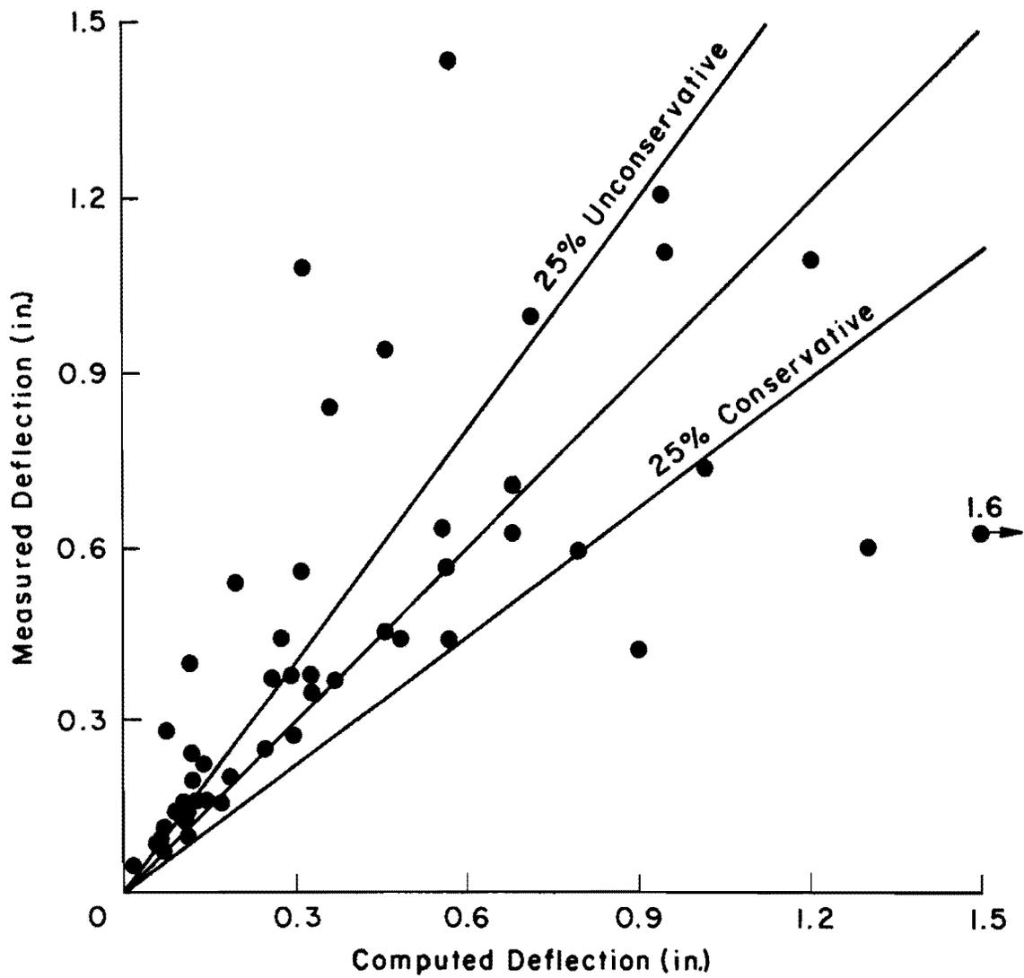
Fig. 4.28. Measured versus computed deflections for tests using StiffA criteria.
