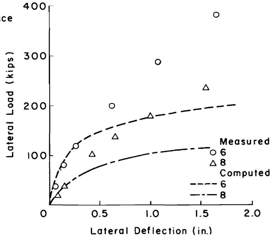
Fig. 4.24. Comparison between measured and computed deflections for test piles 6 and 8 for Southern California Edison.
