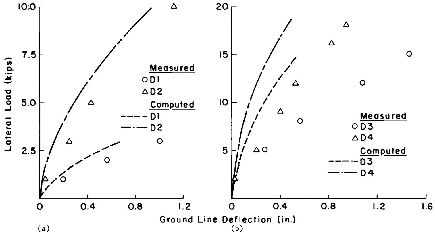
Fig. 4.6. Comparison between measured and computed deflections for tests at dry bay mud site. (a) test piles D1 and D2. (b) test piles D3 and D4.
