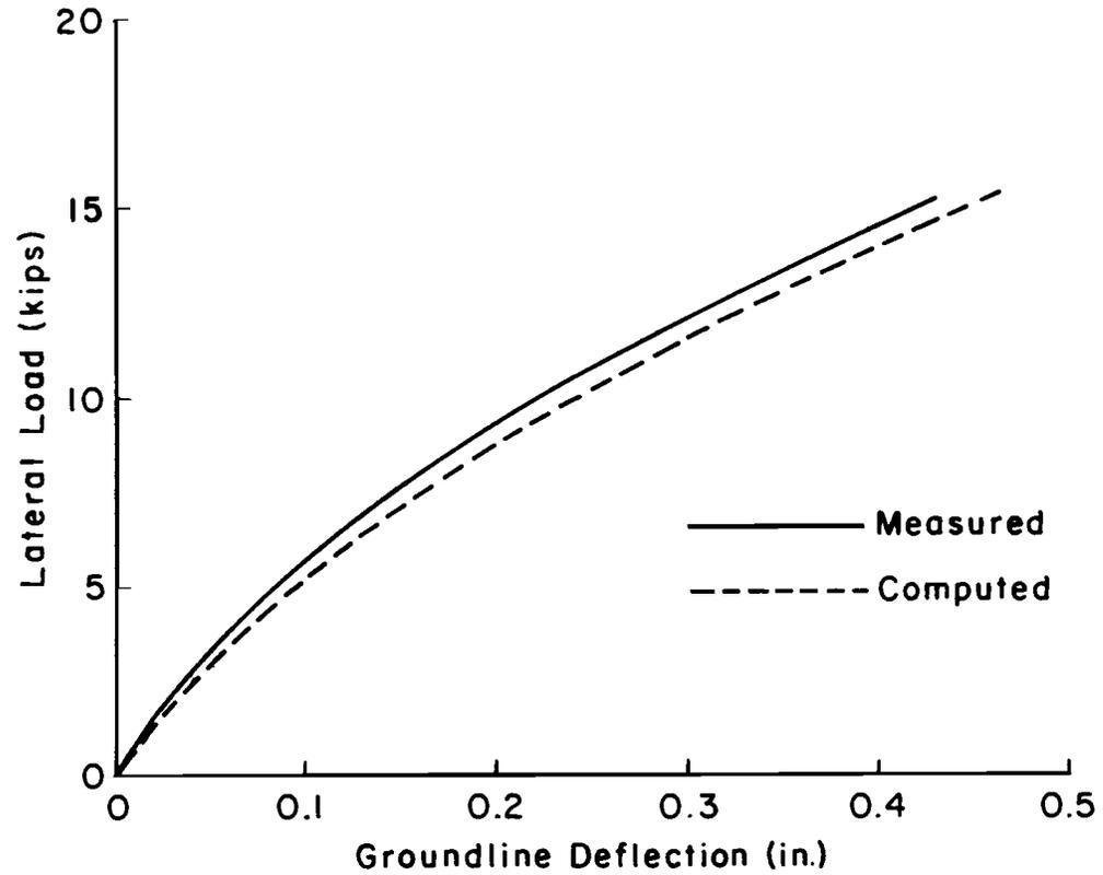
Fig. 5.13. Comparisons between measured and computed deflections for test pile 8 at Arkansas River.
