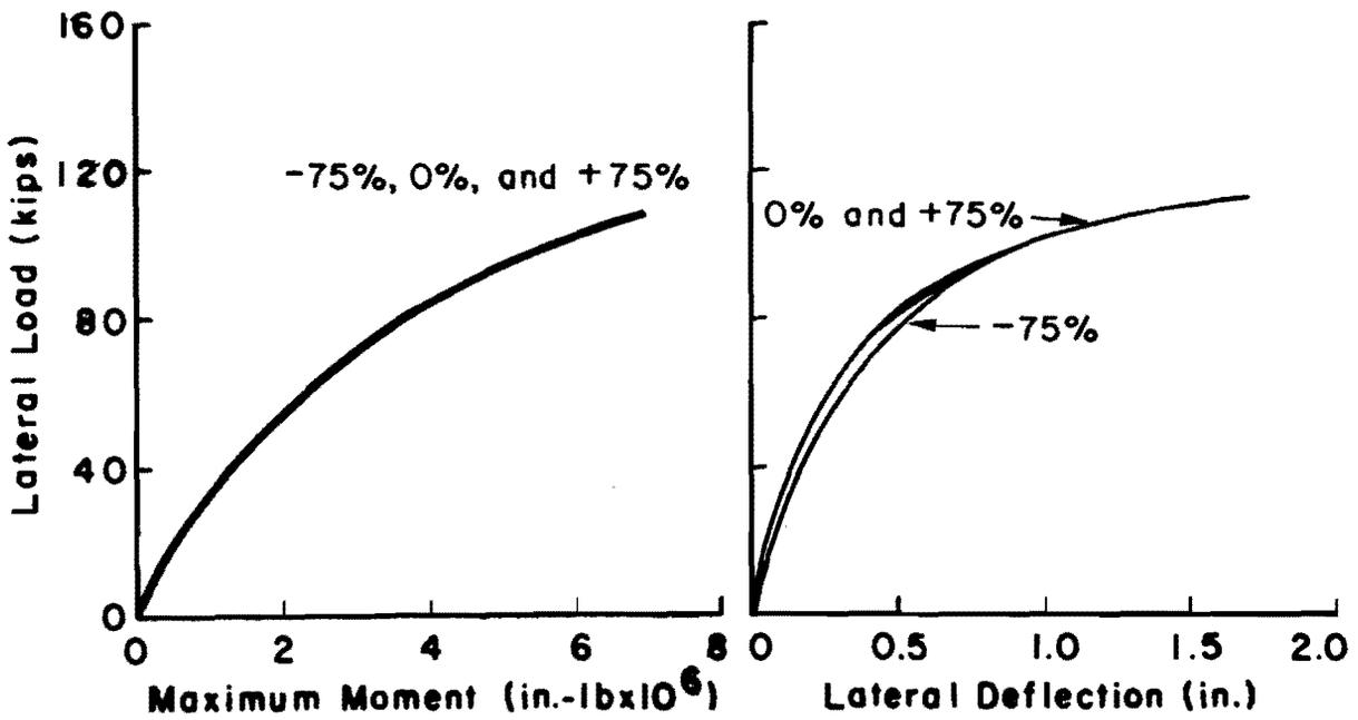
Fig. 3.8. Comparison between results for  $\pm 75\%$  variation in  $k_s$  using StiffB criteria for static loading.
