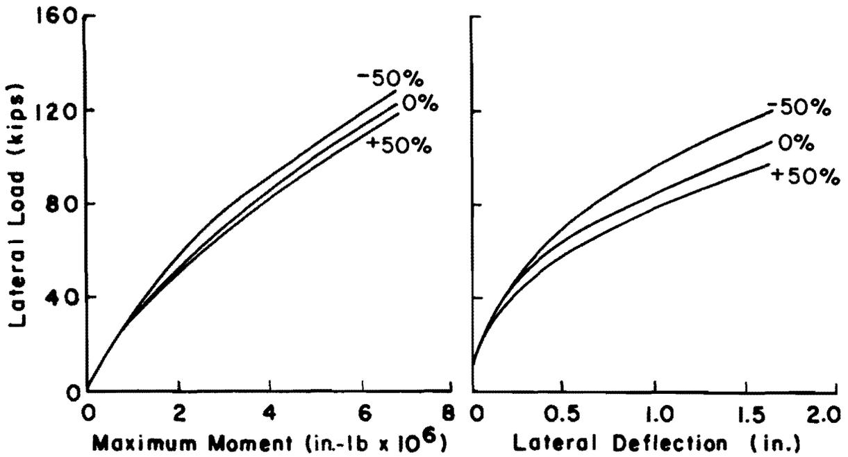
Fig. 3.5. Comparison between results for  $\pm 50\%$  variation in  $\epsilon_{50}$  using StiffA criteria for cyclic loading.
