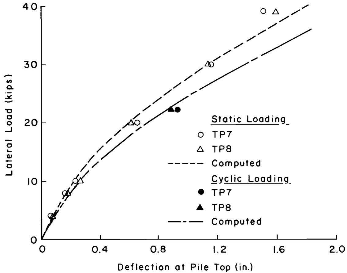
Fig. 5.20. Comparison between measured and computed deflections for test at Bailly.
