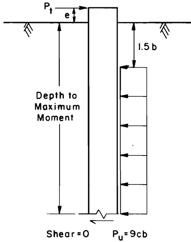
Fig. 1.1. Distribution of ultimate soil resistance for cohesive soils suggested by Broms.
