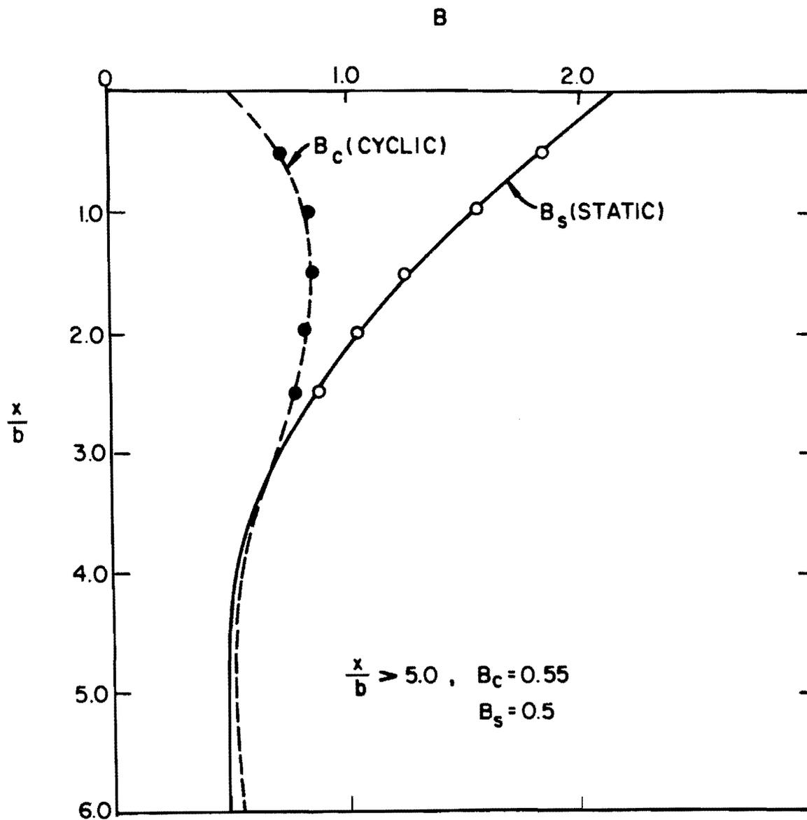
Fig. 2.9. Nondimensional coefficient  $B$  for soil resistance versus depth. (Reese et al., 1974).
