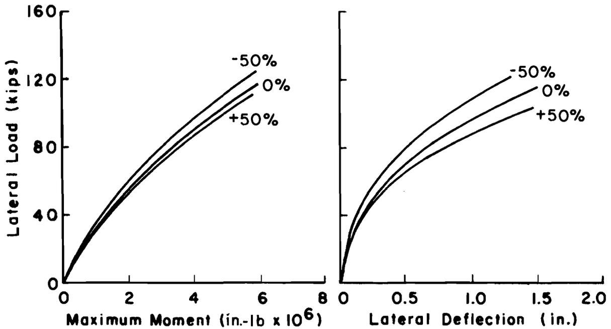
Fig. 3.17. Comparison between results for  $\pm 50\%$  variation in EI for a flexible pile using StiffA criteria for static loading.
