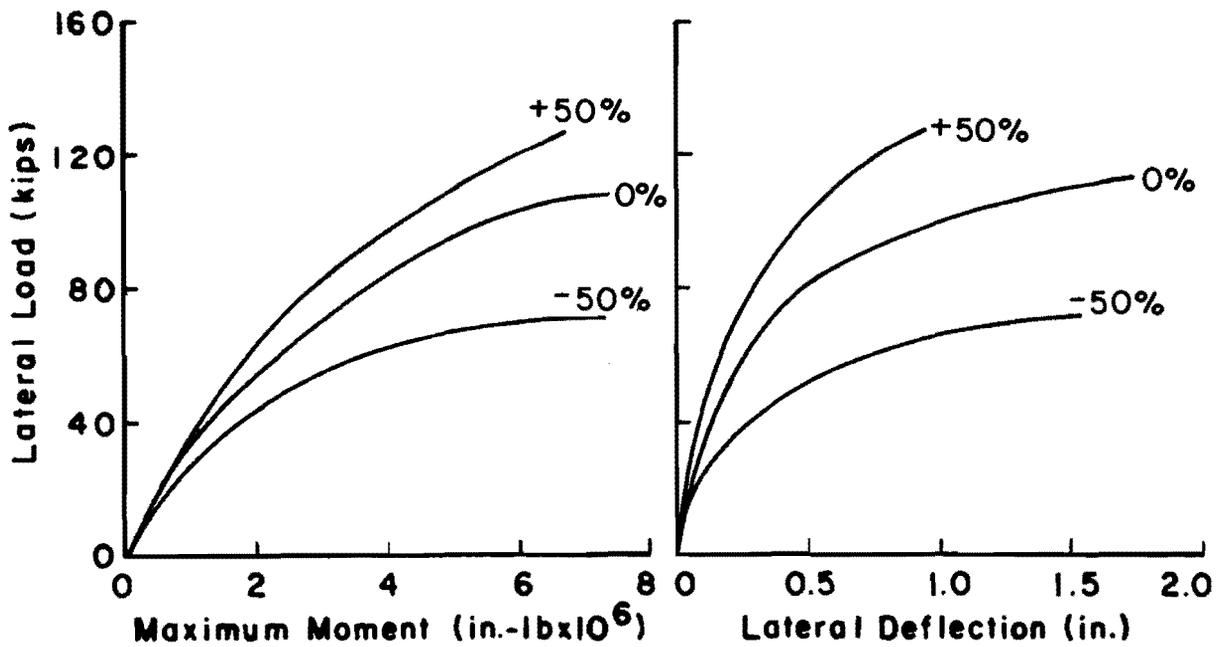
Fig. 3.6. Comparison between results for  $\pm 50\%$  variation in  $c$  using StiffB criteria for static loading.
