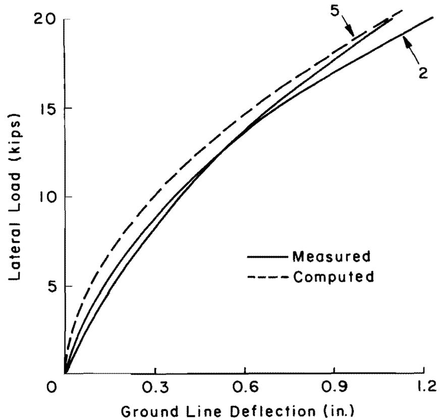
Fig. 4.20. Comparison between measured and computed deflections for tests at Savannah River.
