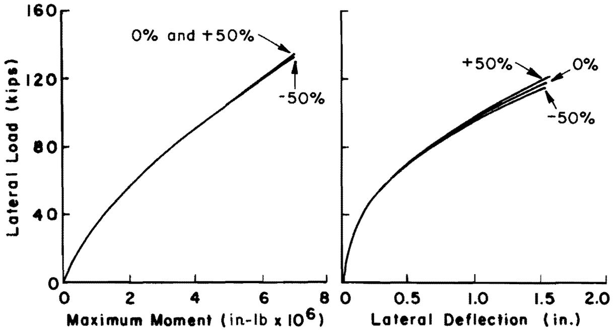
Fig. 3.3. Comparison between results for  $\pm 50$  variation in  $\gamma$  using StiffA criteria for static loading.
