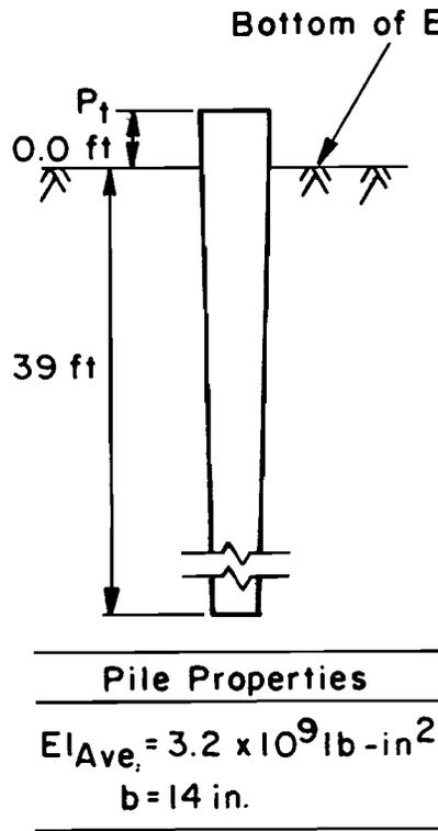
Fig. 5.12. Test setup and pile properties for test pile 8 at Arkansas River.
