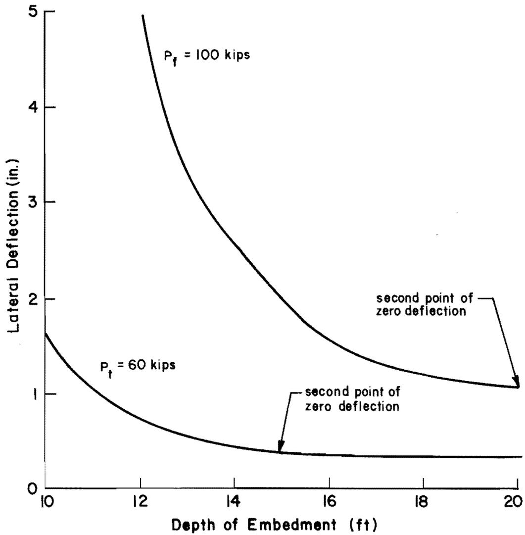
Fig. 3.19. Effect of depth of embedment on lateral deflection.
