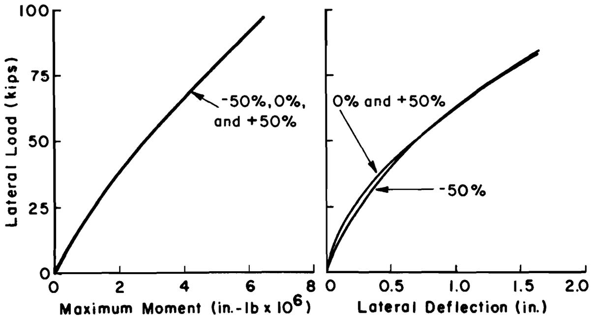
Fig. 3.14. Comparison between results for  $\pm 50\%$  variation in  $k$  using sand criteria for static loading.
