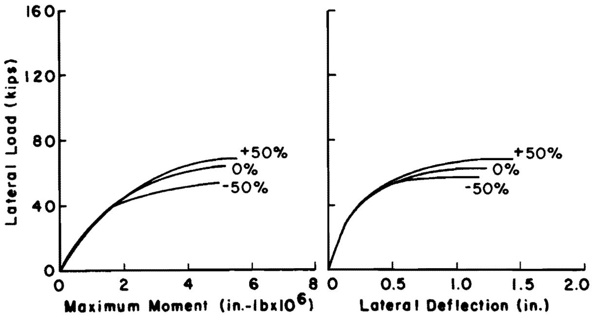
Fig. 3.10. Comparison between results for  $\pm 50\%$  variation in  $\epsilon_{50}$  using StiffB criteria for cyclic loading.
