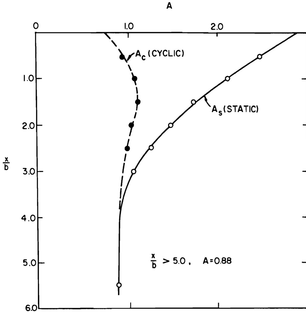
Fig. 2.7. Nondimensional coefficient  $A$  for ultimate soil resistance versus depth. (Reese et al., 1974).
