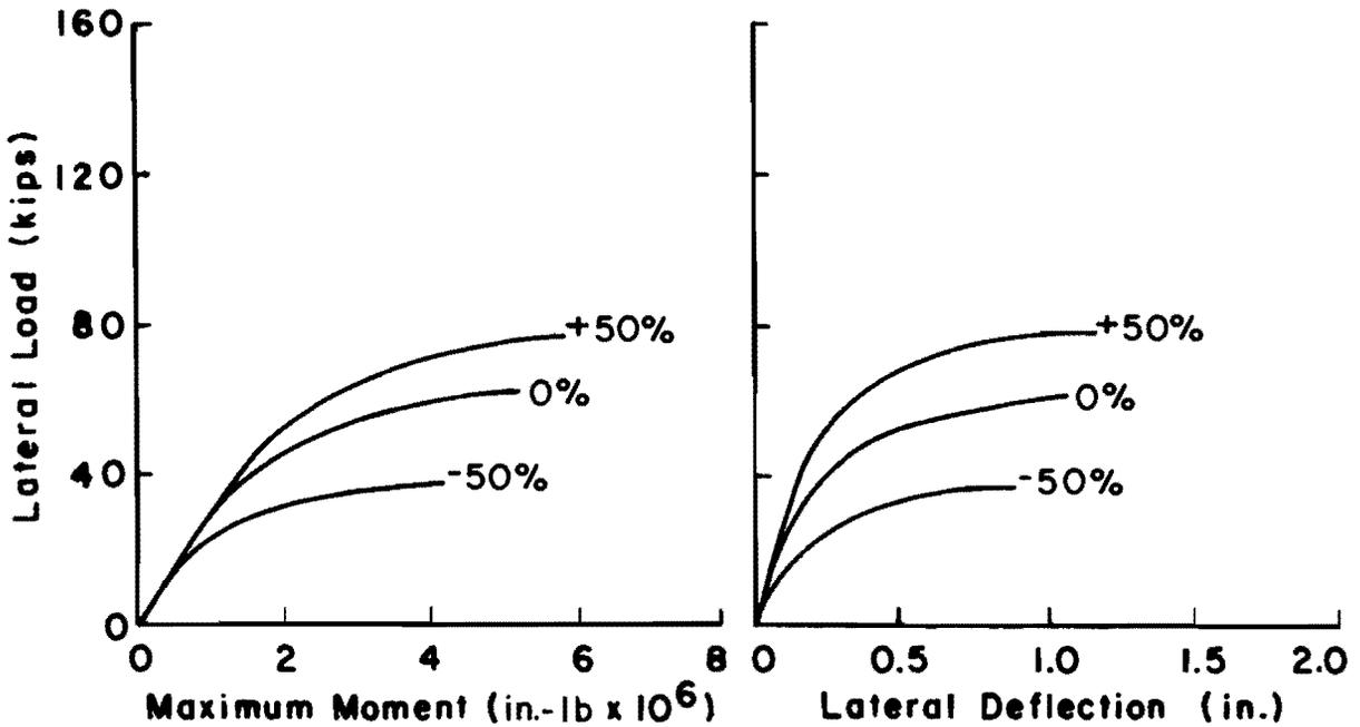
Fig. 3.9. Comparison between results for  $\pm 50\%$  variation in  $c$  using StiffB criteria for cyclic loading.
