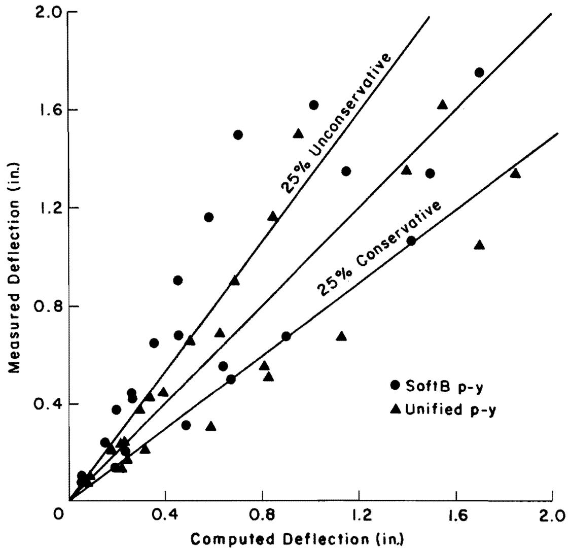
Fig. 4.27. Comparison between measured and computed deflections for tests using softB and unified criteria.
