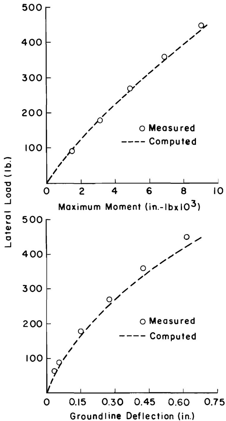
Fig. 5.28. Comparison between measured and computed results for model tests at The University of Texas.
