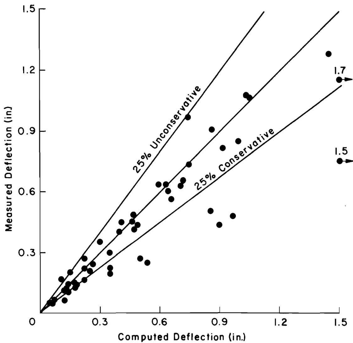
Fig. 5.29. Comparison between measured and computed deflections for tests using criteria for sand.
