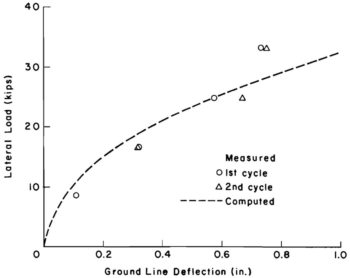
Fig. 4.14. Comparison between measured and computed deflections for test at Lewisburg.
