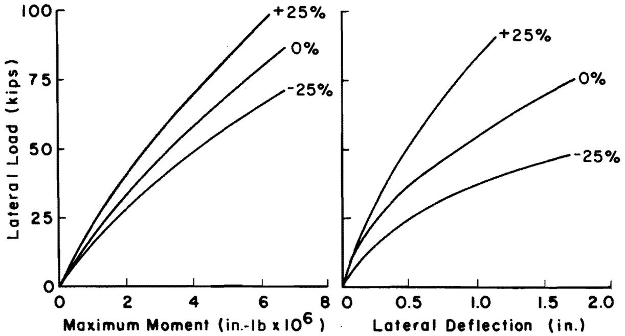
Fig. 3.15. Comparison between results for  $\pm 25\%$  variation in  $\phi$  using sand criteria for cyclic loading.
