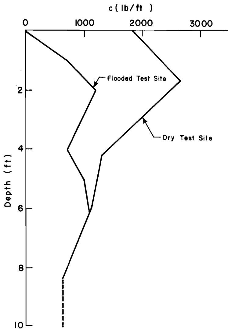
Fig. 4.5. Vane shear strength profiles for tests performed in bay mud.
