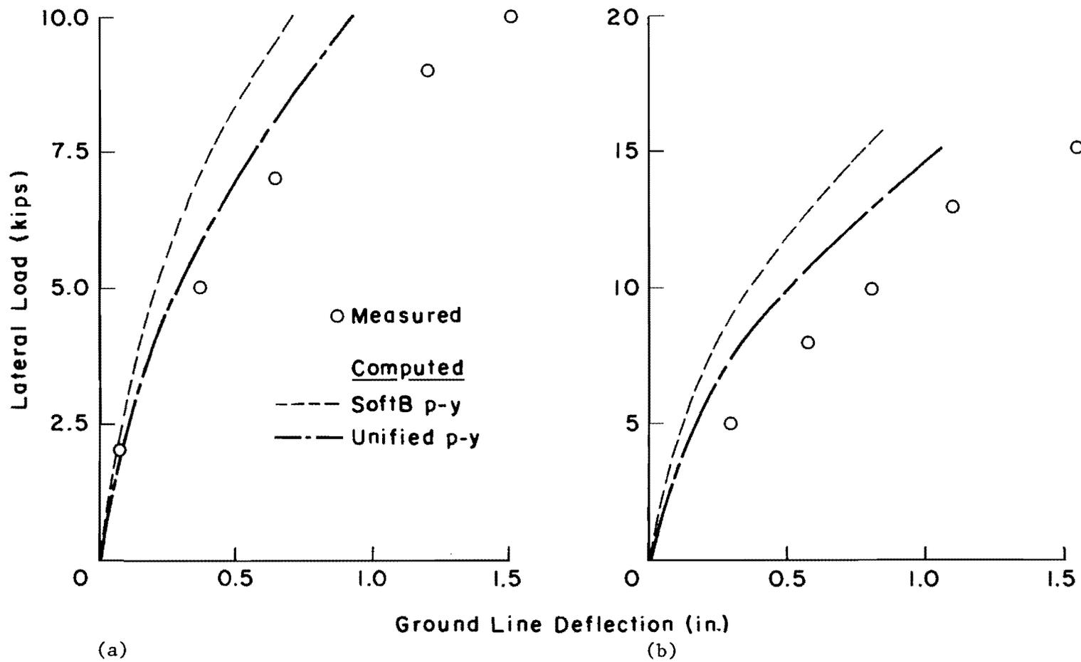
Fig. 4.8. Comparison between measured and computed deflections at flooded bay mud site. (a) test pile F3. (b) test pile F4.
