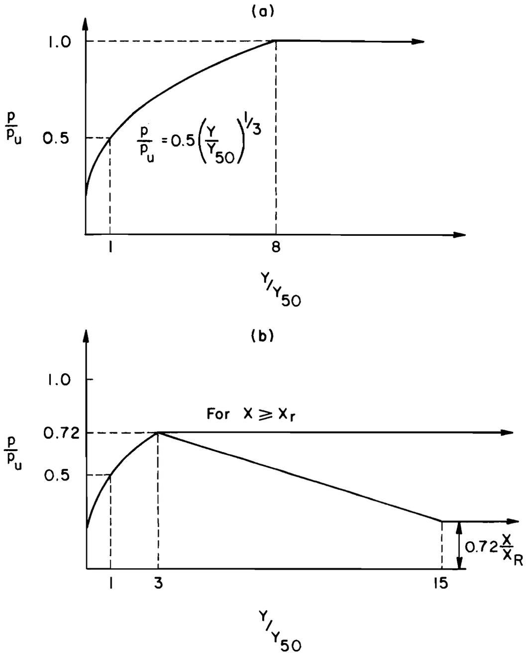
Fig. 2.1. Characteristic shape of the p-y curves for soft submerged clay (Matlock, 1970), (a) static loading. (b) cyclic loading.
