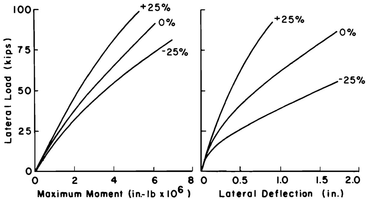
Fig. 3.11. Comparison between results for  $\pm 25\%$  variation in  $\phi$  using sand criteria for static loading.
