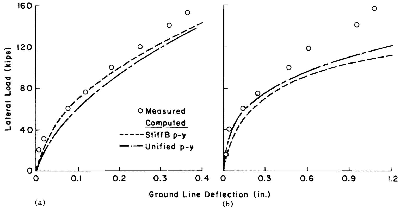
Fig. 4.16. Comparison between measured and computed deflections for tests at Ontario.
