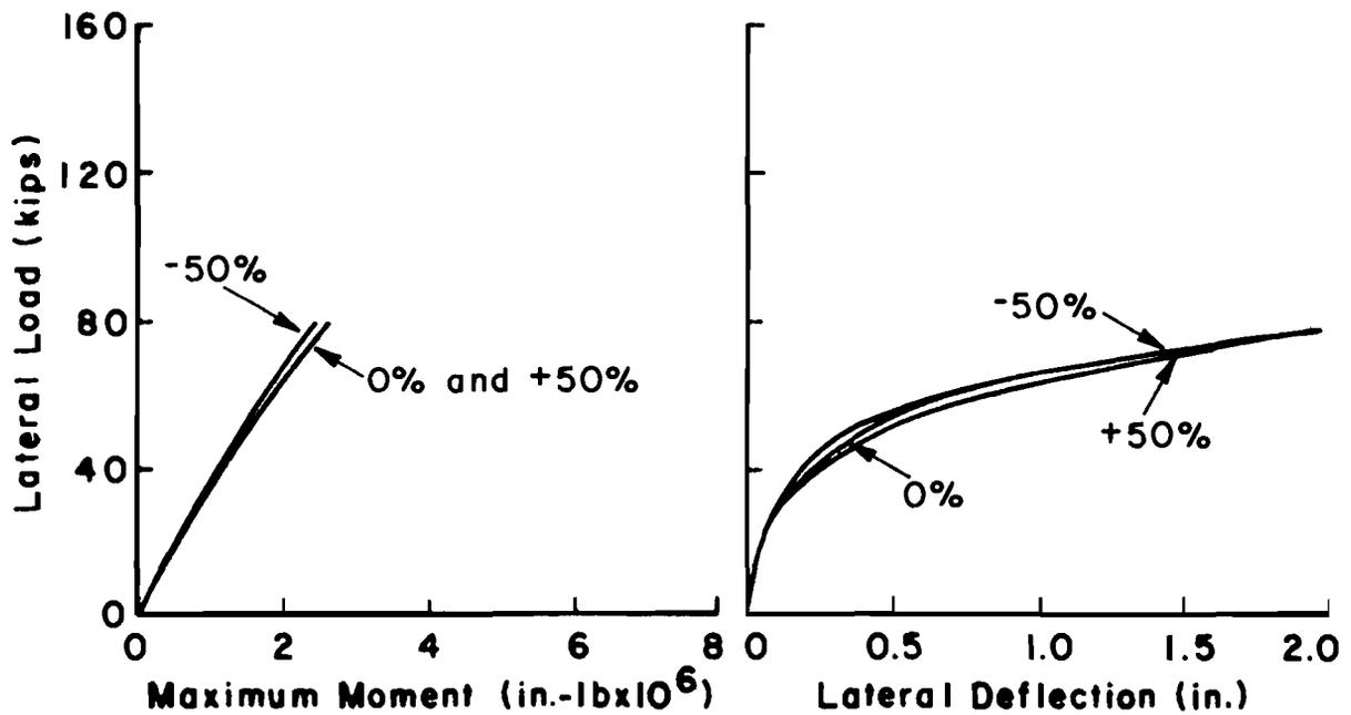
Fig. 3.18. Comparison between results for  $\pm 50\%$  variation in EI for a rigid pile using StiffA criteria for static loading.
