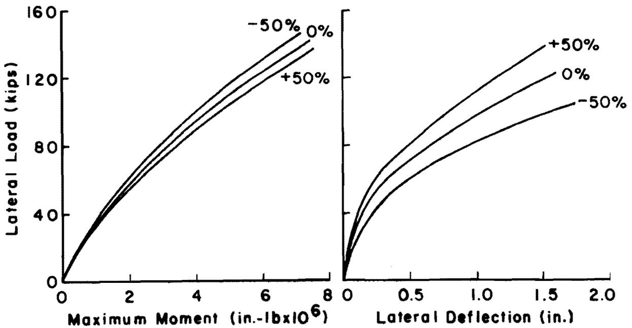
Fig. 3.2. Comparison between results for  $\pm 50\%$  variation in  $\epsilon_{50}$  using the StiffA criteria for static loading.
