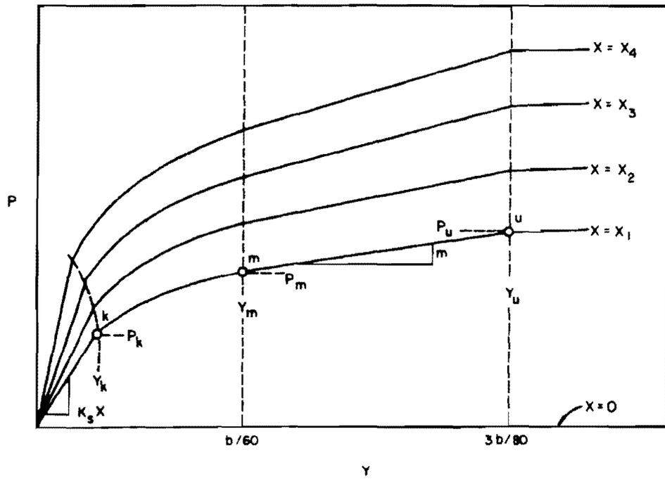
Fig. 2.8. Characteristic shape of a family of p-y curves in sand. (Reese, et al., 1974).
