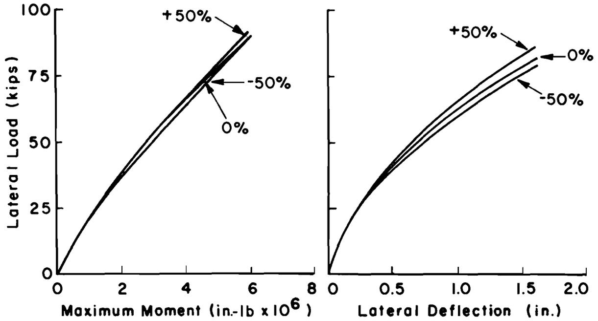
Fig. 3.13. Comparison between results for  $\pm 50\%$  variation in  $K_0$  using sand criteria for static loading.
