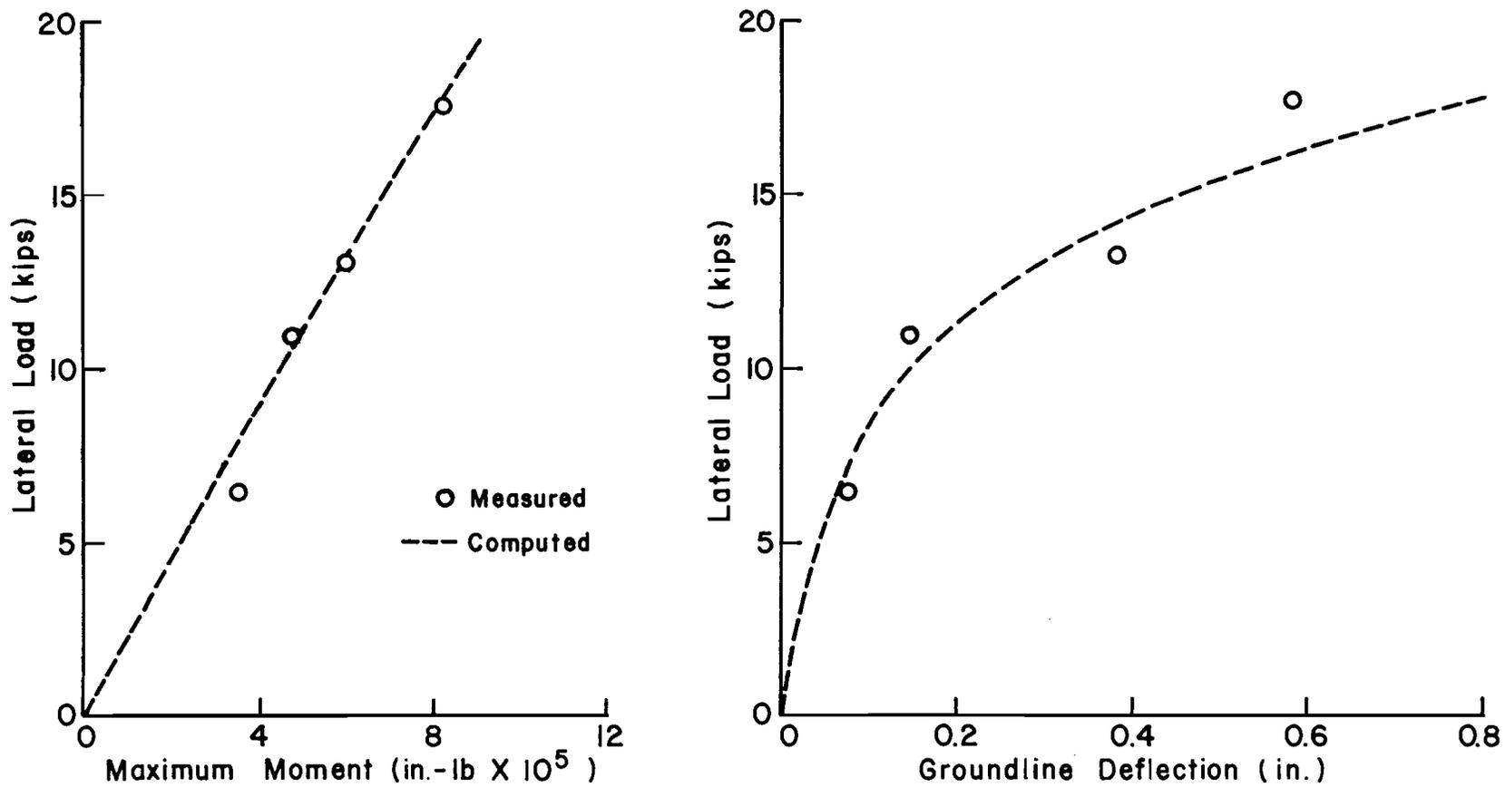
Fig. 4.3. Comparison between measured and computed results for test pile B5 at Bagnolet.
