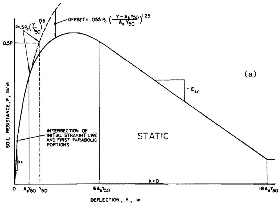
Fig. 2.4. Characteristic shape of the p-y curves for stiff clay below the water table. (Reese et al, 1975). (a) static loading. (b) cyclic loading.
