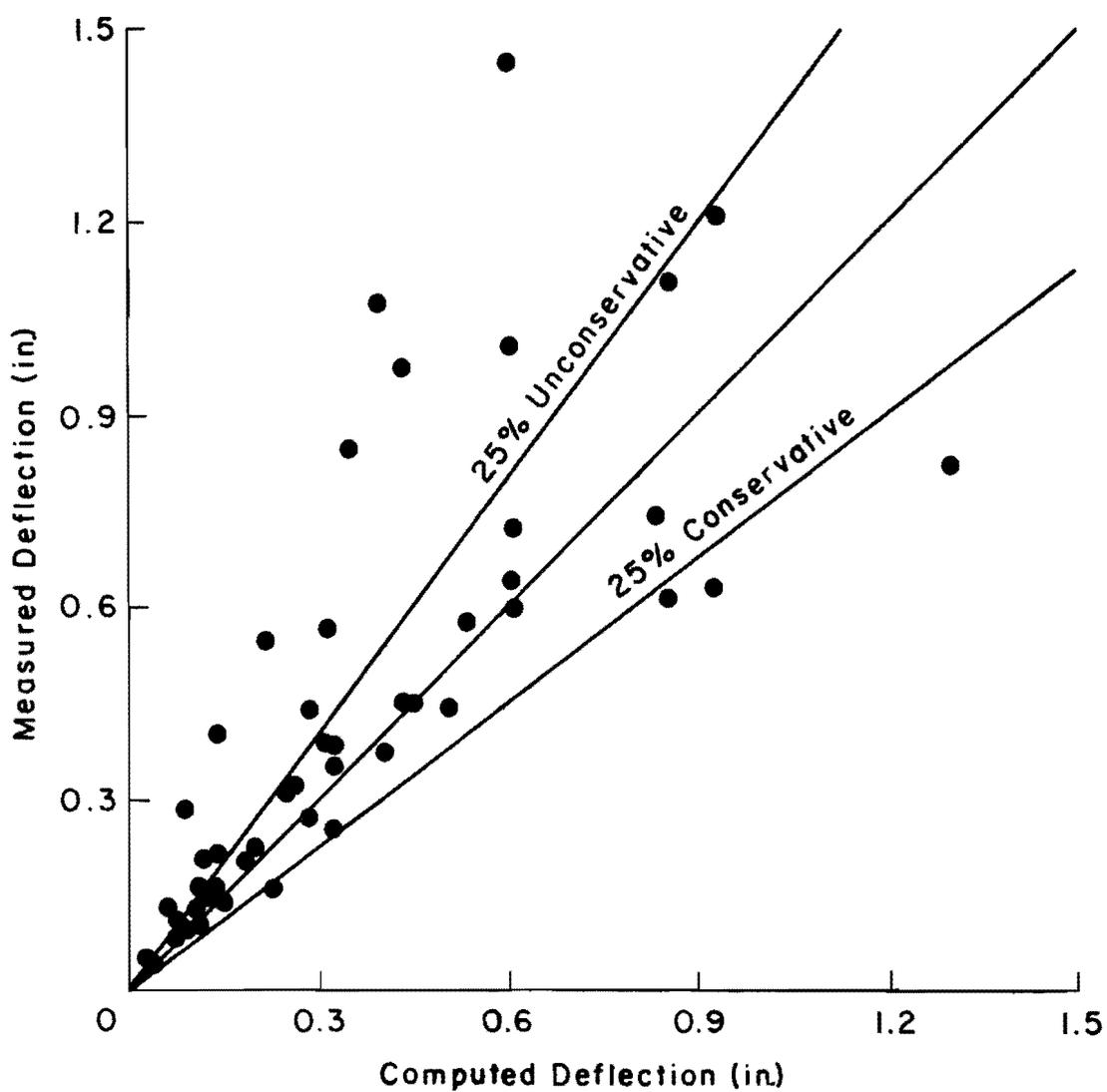
Fig. 4.29. Comparison between measured and computed deflections for tests using modified StiffA criteria.
