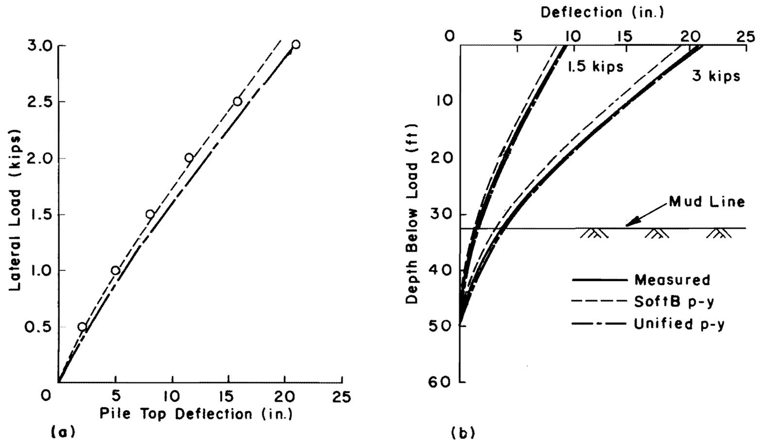
Fig. 4.10. Comparison between measured and computed results for test at Hudson River.
