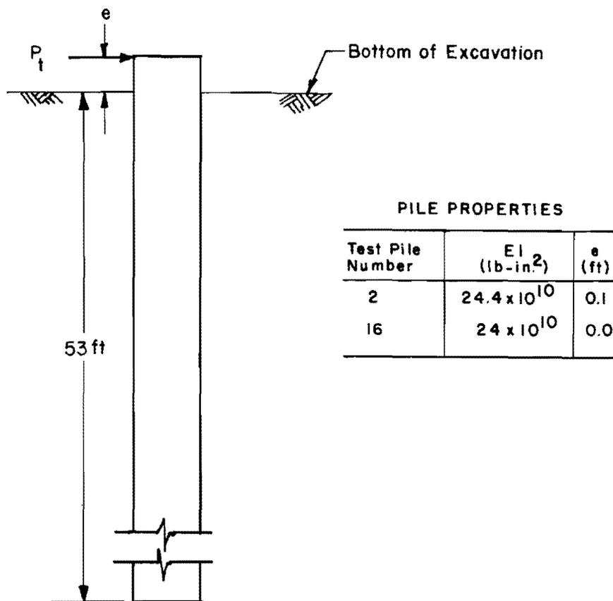
Fig. 5.6. Test setup and pile properties for test piles 2 and 16 at Arkansas River.
