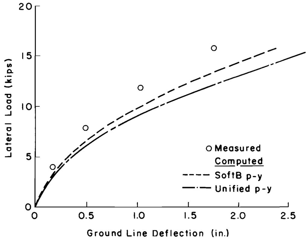
Fig. 4.26. Comparison between measured and computed deflections for test at St. Gabriel.
