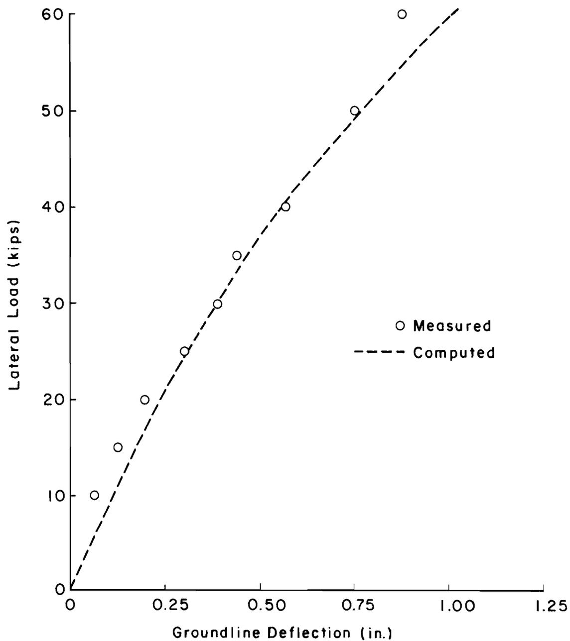
Fig. 5.22. Comparison between measured and computed deflections for test in Florida.
