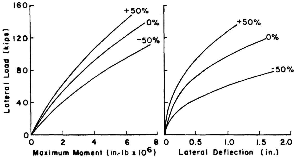
Fig. 3.1. Comparison between results for  $\pm 50\%$  variation in  $c$  using StiffA criteria for static loading.
