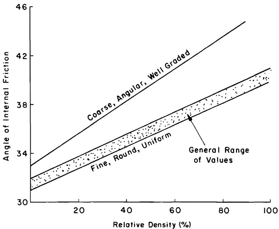
Fig. 5.1. Correlation between angle of internal friction and relative density (Schmertmann, 1975).
