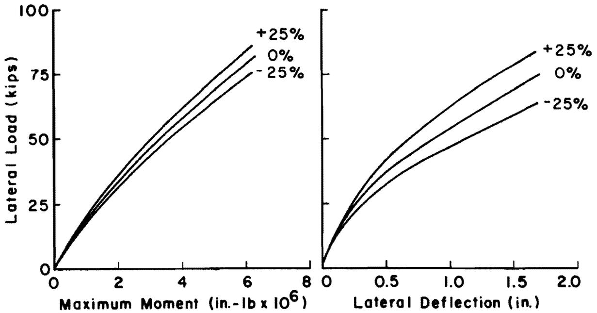
Fig. 3.16. Comparison between results for  $\pm 25\%$  variation in  $\gamma$  using sand criteria for cyclic loading.
