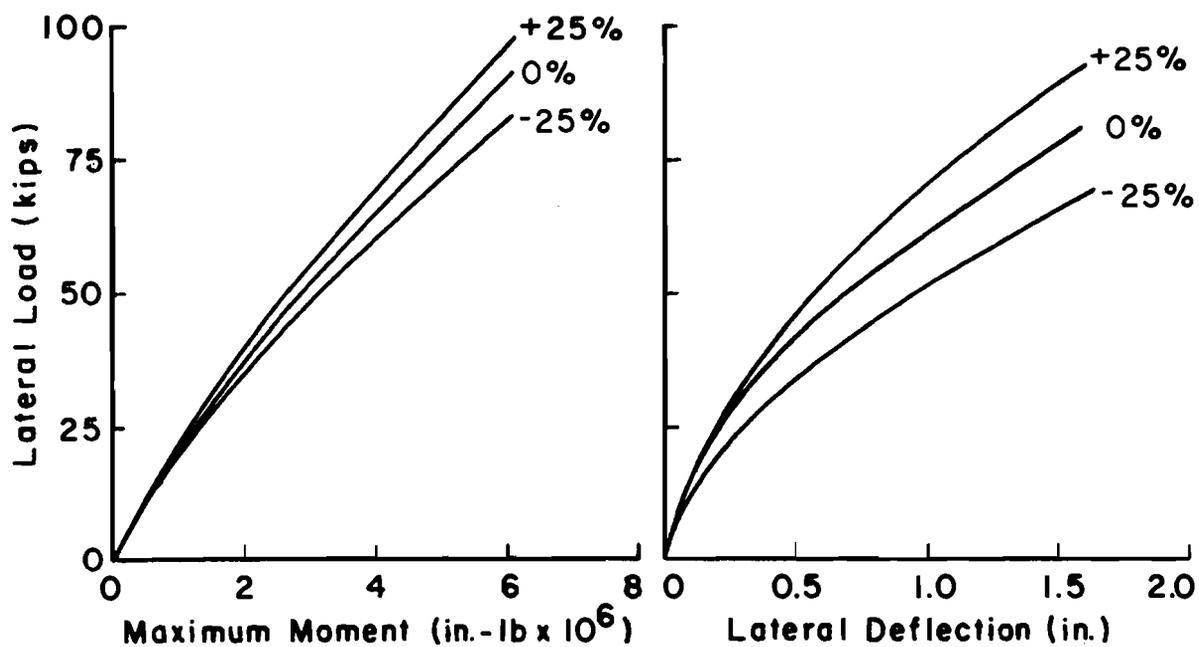
Fig. 3.12. Comparison between results for  $\pm 25\%$  variation in  $\gamma$  using sand criteria for static loading.
