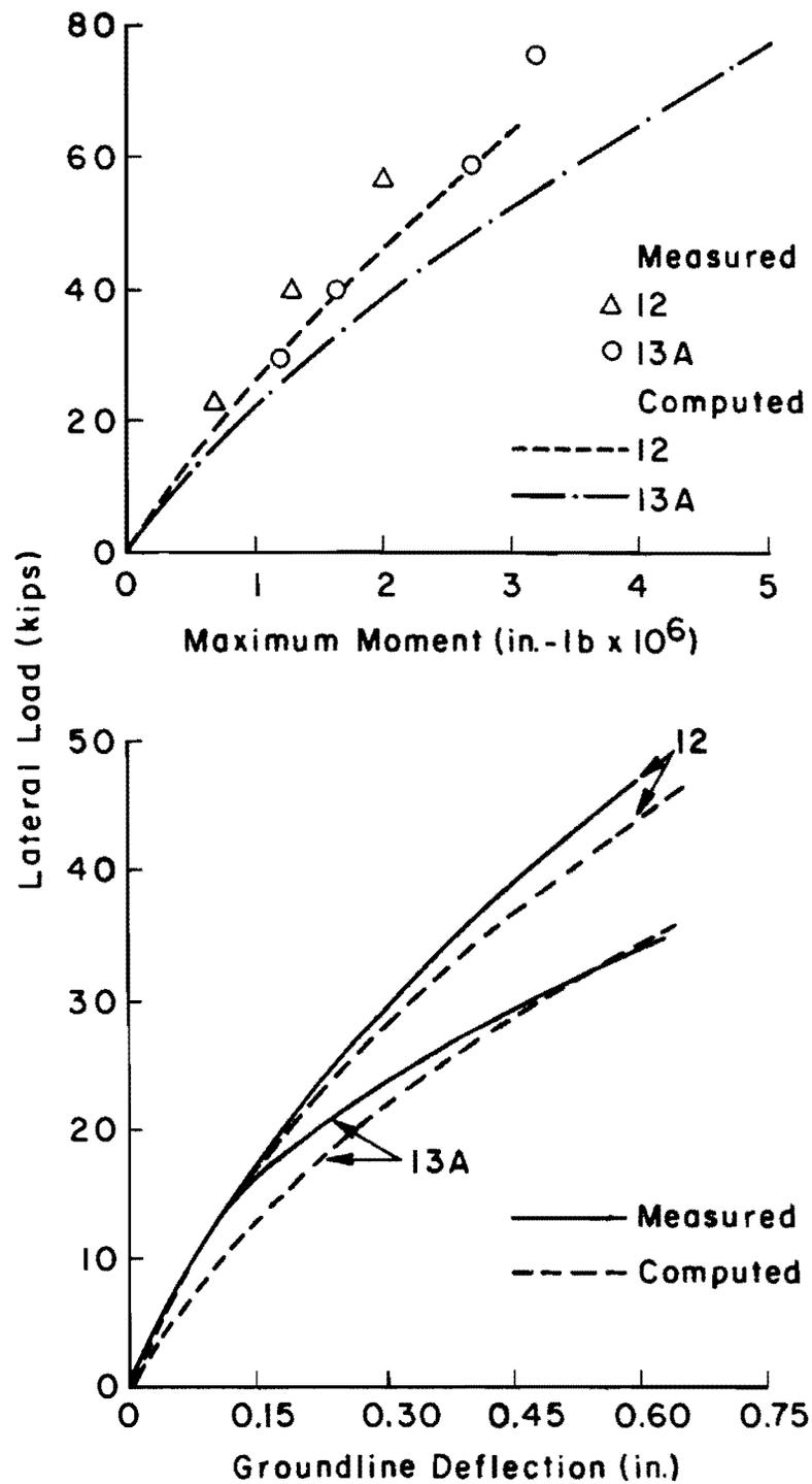
Fig. 5.16. Comparison between measured and computed results for test piles 12 and 13a at Arkansas River.
