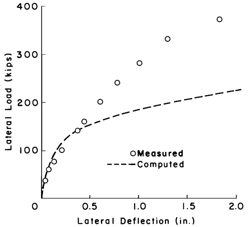
Fig. 4.22. Comparison between the measured and computed deflections for test pile 2 for Southern California Edison.
