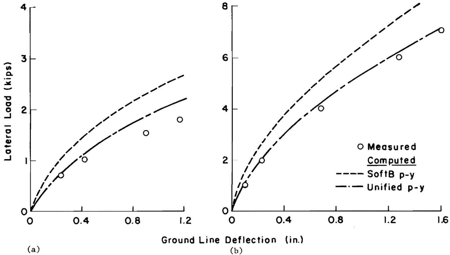
Fig. 4.7. Comparison between measured and computed deflections at flooded bay mud site. (a) test pile F1. (b) test pile F2.
