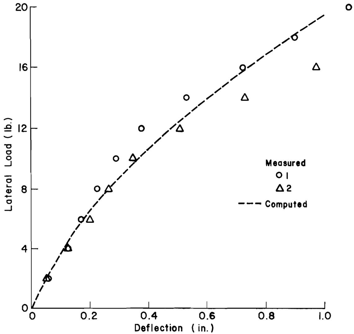
Fig. 5.18. Comparison between measured and computed deflections for test at Apapa.
