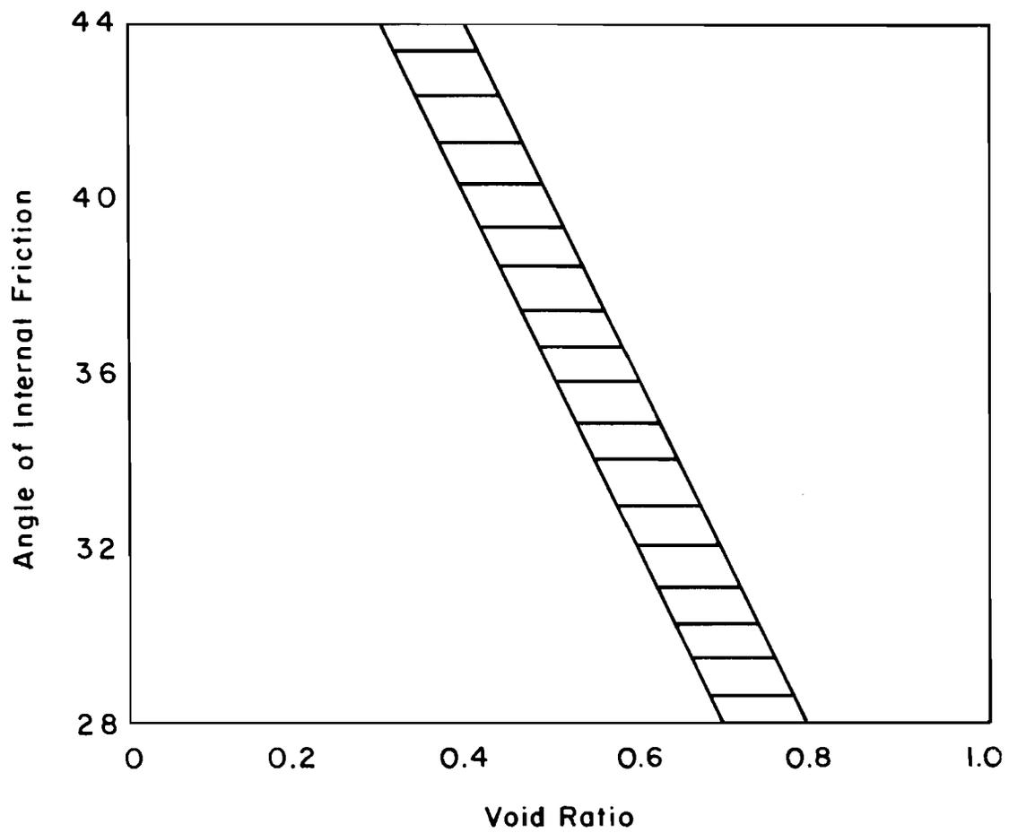
Fig. 5.4. Approximate relationship between angle of internal friction and void ratio for reported sands.
