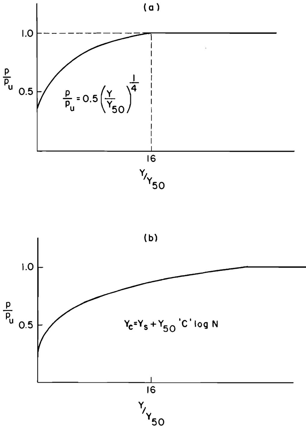
Fig. 2.2. Characteristic shape of the p-y curves for stiff clay above the water table. (a) static loading. (b) cyclic loading.
