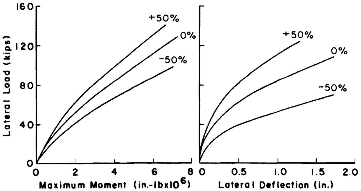
Fig. 3.4. Comparison between results for  $\pm 50$  variation in  $c$  using StiffA criteria for cyclic loading.
