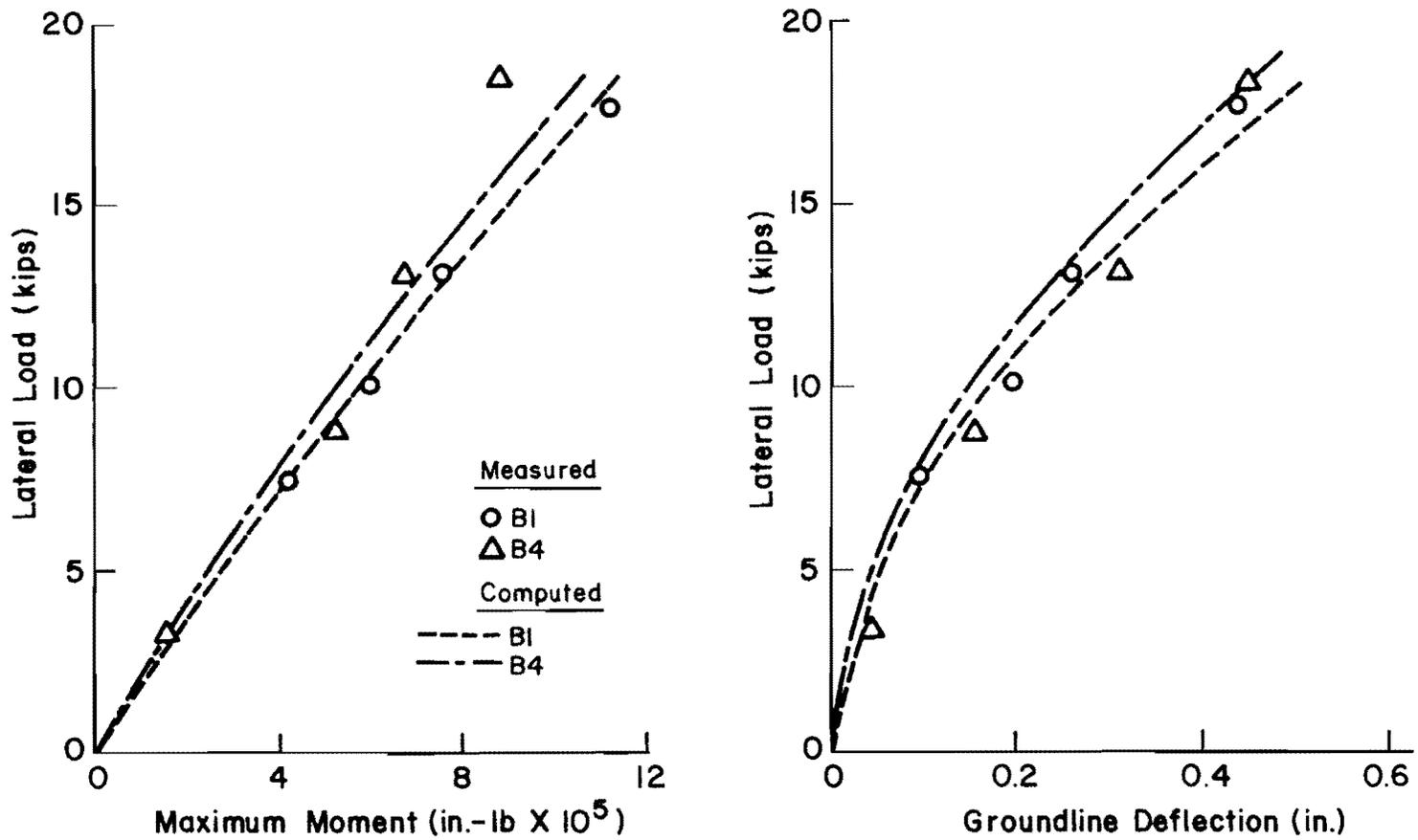
Fig. 4.2. Comparison between measured and computed results for test piles B1 and B4 at Bagnolet.
