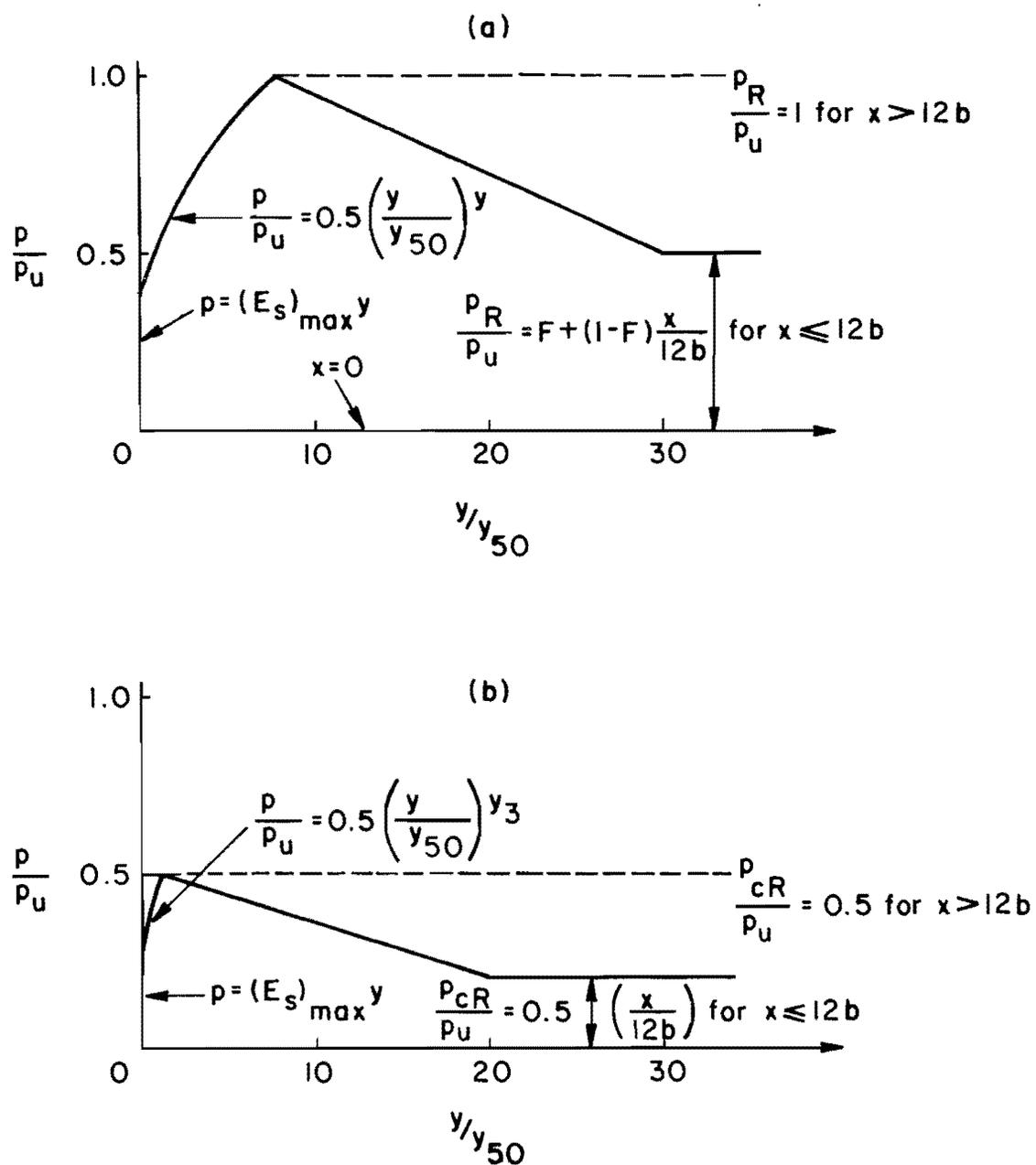
Fig. 2.6. Characteristic shape of the  $p$ - $y$  curves for clay, Unified criteria (Sullivan, 1977). (a) static loading. (b) cyclic loading.
