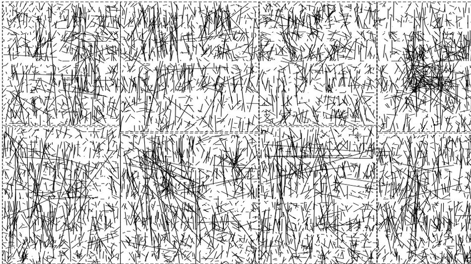
Fig. 4. “Uncut” nets of degree two on the third placement level, represented by line segments. The pin locations for a given net are strongly correlated: most nets span less than two cell rows.
