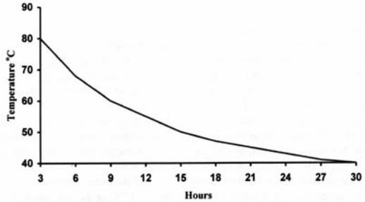
moulding. Whilst the resin cannot be over cured, it is not advisable to raise the temperature above 140°C. The influence of moulding temperature on the setting time of a typical polyester resin is shown in Figure 17.
