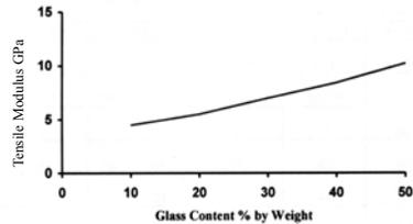
Figure 7 - Effect of glass content and orientation on the tensile strength of glass reinforced polyester laminates
