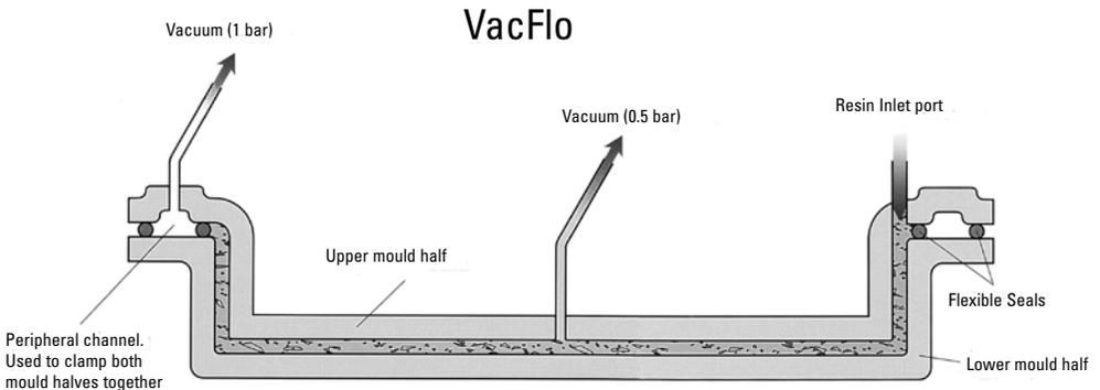
Once the gelcoat is sufficiently cured, the reinforcement is put in place. Finally, the required amount of catalysed resin is poured into the mould and the tools are closed.
