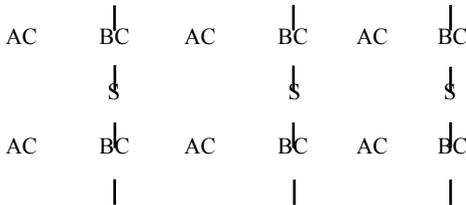
At this stage, the polyester resin is said to be cured. It is now a chemically resistant and (usually) hard solid. The cross-linking, or curing, process is called polymerisation and is a non-reversible chemical reaction.
