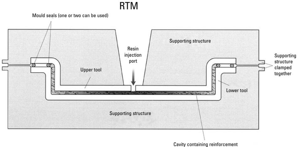
tolerances achieved, leading to mechanical properties which are more consistent and easier to accurately predict. One of the greatest benefits of closed mould systems, however, is their impact on the environment, as styrene emissions during moulding can be virtually eliminated by using these processes.
