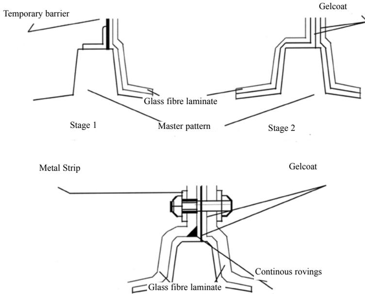
localised loads imposed by nuts and bolts or clamps, and for this reason, they should be made 50% thicker than the mould shell. It is also best to fix metal plates along the flanges so that fixings can be made every 150mm or so, to hold the two halves of the mould together.
