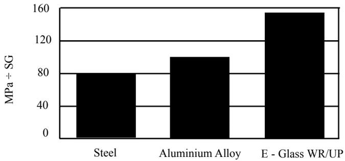
Figure 3 - Specific Tensile Modulus - Steel, Aluminium and GFRP
