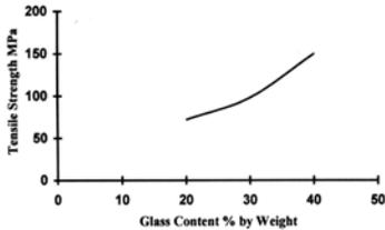
Figure 6 - Effect of glass content on the tensile modulus of random glass reinforced polyester laminates
