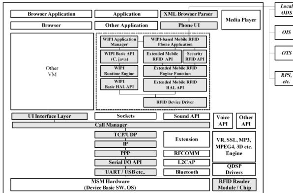
Fig.1. Mobile RFID Security S/W Architecture based on Cellular Phone.
