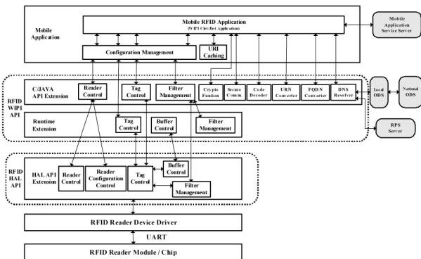
Fig.2. Security Enhanced Mobile RFID Middleware in the Mobile Phone.
