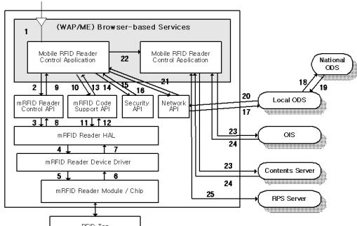
Fig.4. Scenario of Secure Mobile RFID M/W Terminal Function.
