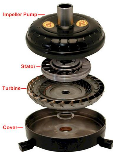
Fig.2 Constructional view of a hydraulic torque converter.
