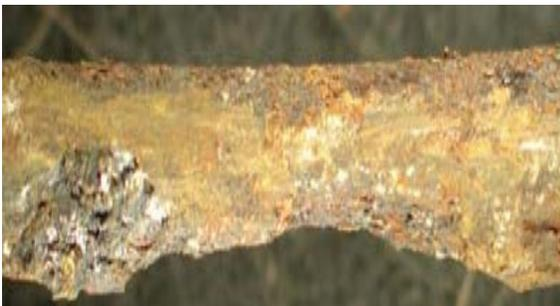
Fig.5. Crater dissolution (locally reduced by 50% of section)
