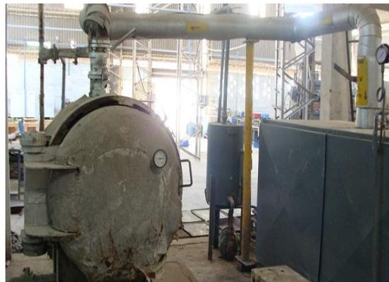
Fig. 1(c) Autoclave used for Dewaxing
