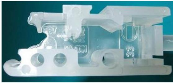
Fig. 14 Defects on part – short shots on real part
