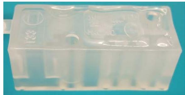
Fig. 13 Defects on part – sink marks
