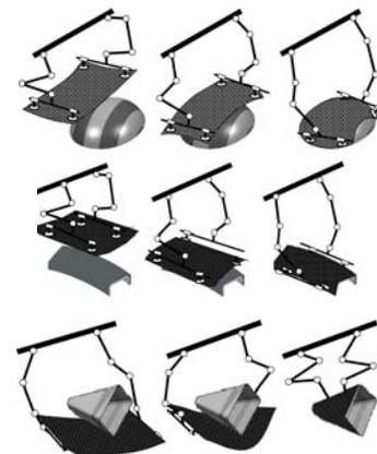
Fig.2 Work sequence in mould draping and wrapping tasks of carbon fibre preforms on different moulds
