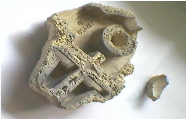
Fig. 3(a) Typical inside portion (after breaking) of the Sintered Shell
