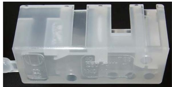
Fig. 12 Defects on part – voiding marks
