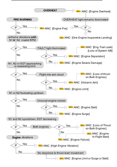
The flow chart above analyses all different kinds of engine failures. As a result, it is far too complex for use in flight. Since multiple kinds of engine failures refer to the same NNC, the following logic gate is more useful in flight:
