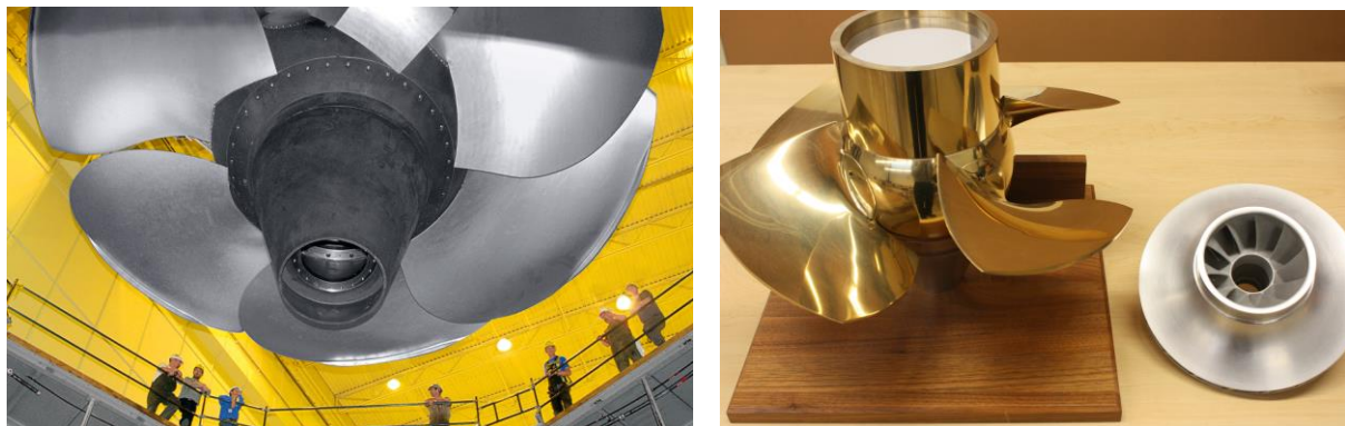
Figure 22: Prototype Kaplan Turbine (left) 27 , Model-size turbines (right)
