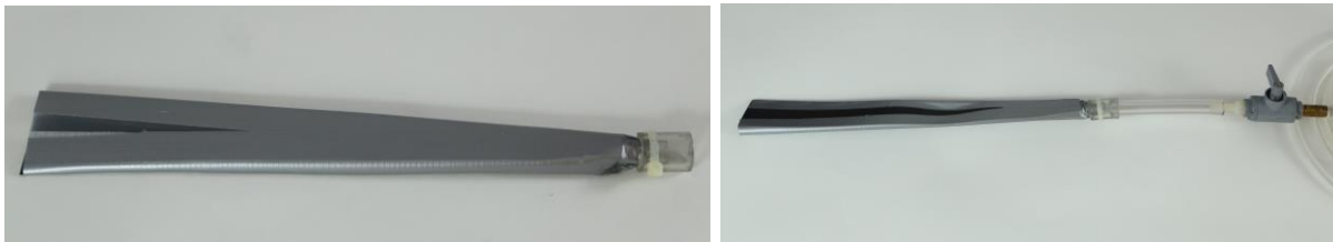
Figure 27: The diffuser (left) and the diffuser attached to the RankineCycler™ beaker
