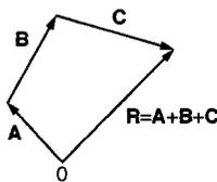
FIGURE 1.2.3 Addition of concurrent, coplanar vectors  $\mathbf{A}$ ,  $\mathbf{B}$ , and  $\mathbf{C}$ .
