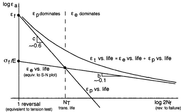
FIGURE 1.6.26 Schematic of strain vs. life curves.
