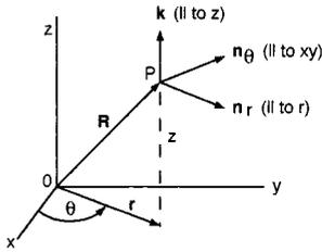
FIGURE 1.3.6 Motion of a particle in cylindrical coordinates.
