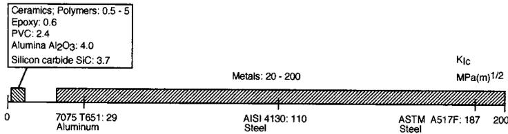
FIGURE 1.6.7 Plane strain fracture toughness ranges (approximate).
