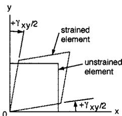
FIGURE 1.5.12 Shear strain in two dimensions.
