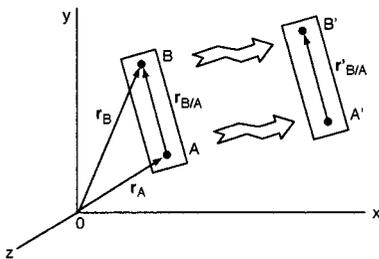
FIGURE 1.3.9 Translational motion of a rigid body.
