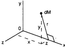
FIGURE 1.2.28 Mass element  $dM$  in  $xyz$  coordinates.
