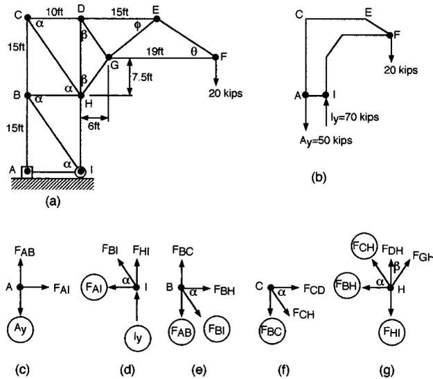
FIGURE 1.2.23 Method of joints in analyzing a truss.
