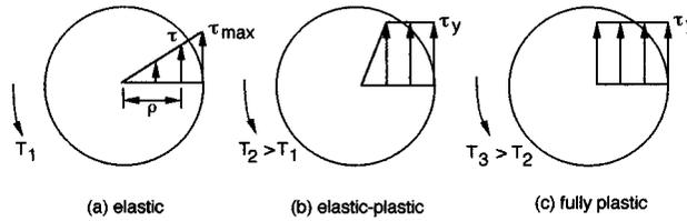
FIGURE 1.5.25 Shear stress distributions in a shaft.
