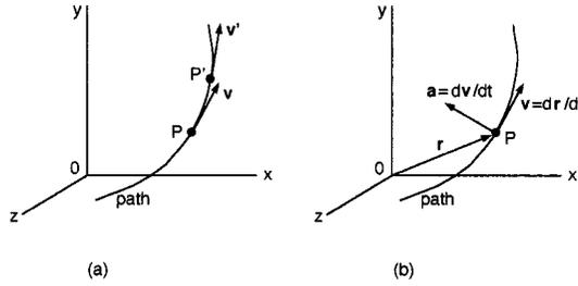
FIGURE 1.3.3 Vector method for a particle.
