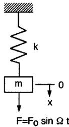
FIGURE 1.4.1 Model of a simple vibrating system.
