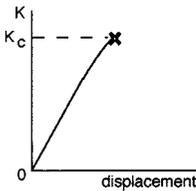
FIGURE 1.6.5  $K_c$  = fracture toughness of a particular member.
