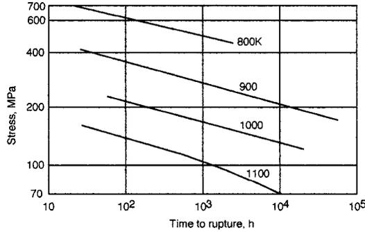
**FIGURE 1.6.15** Approximate stress vs. rupture lives of S-590 alloy as functions of temperature. (After Figure 15.8, Dowling, N. E. 1993. *Mechanical Behavior of Materials*. Prentice-Hall, Englewood Cliffs, NJ. With permission.)
