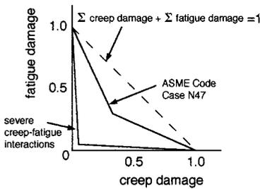
**FIGURE 1.6.27** Schematic of creep-fatigue interactions. The bilinear damage rule is recommended in the ASME Boiler and Pressure Vessel Code, Section III, Code Case N47.
