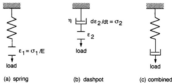
**FIGURE 1.6.16** Viscoelastic elements.
