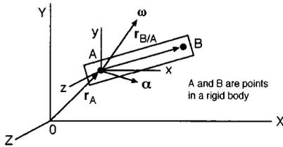
FIGURE 1.3.14 General motion of a rigid body.
