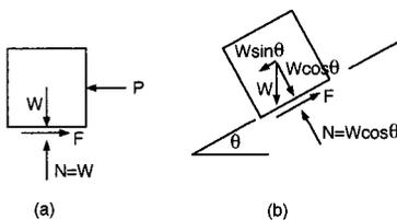
FIGURE 1.2.27 Models showing friction forces.
