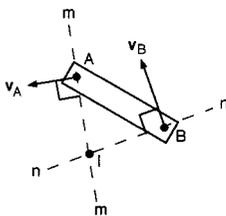
FIGURE 1.3.12 Schematic for instantaneous center of rotation.
