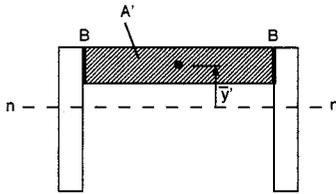
FIGURE 1.5.22 Critical joint regions of a built-up beam.
