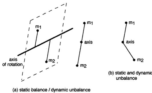
FIGURE 1.4.6 Schematic of two cases of dynamic unbalance.
