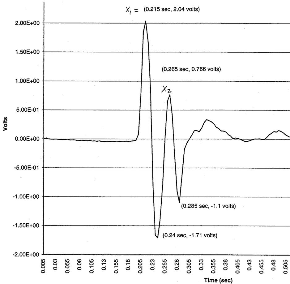
FIGURE 1.7.1 Accelerometer data from front suspension system of vehicle. Logarithmic decrement  $\delta = \ln(x_1/x_2)$ ; damping ratio  $\zeta = 0.16$ .
