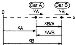
**FIGURE 1.3.2** Relative motion of two particles along a straight line.
