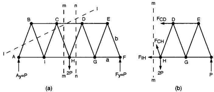
FIGURE 1.2.24 Method of sections in analyzing a truss.
