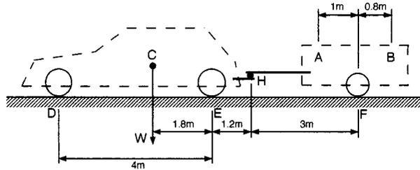
FIGURE 1.2.16 Analysis of a car with trailer.
