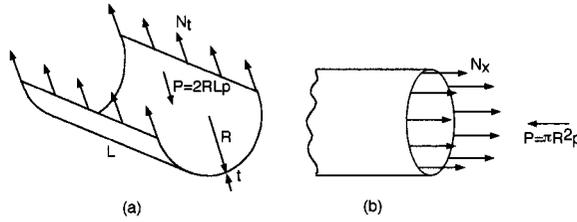
FIGURE 1.5.32 Analysis of cylindrical pressure vessels.
