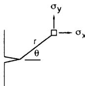
**FIGURE 1.6.4** Coordinates for fracture analysis.
