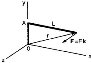
FIGURE 1.2.10 Model of a torque wrench.
