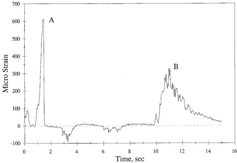
**FIGURE 1.4.7** Strain-time history at one strain-gage location on a steel bridge caused by two trucks moving in opposite directions. (A) Garbage truck in the near lane; (B) tractor trailer in the far lane. Weights unknown. (Data courtesy Mark J. Fleming, University of Wisconsin-Madison.)
