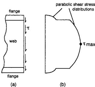
**FIGURE 1.5.21** Shear stress distribution for I-beam.
