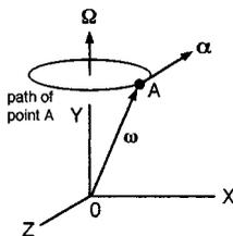
FIGURE 1.3.15 Rigid body fixed at point  $O$ .
