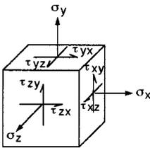
FIGURE 1.5.2 Three-dimensional general state of stress.
