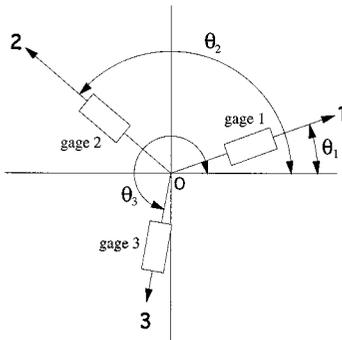
**FIGURE 1.5.41** Three gage elements placed at arbitrary angles relative to the  $x$  and  $y$  axes.
