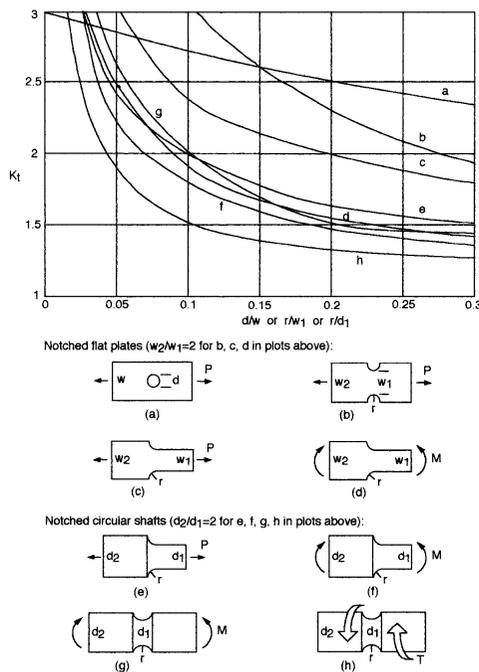
**FIGURE 1.6.2** Samples of elastic stress concentration factors. (Condensed from Figures 10.1 and 10.2, Dowling, N. E. 1993. *Mechanical Behavior of Materials*. Prentice-Hall, Englewood Cliffs, NJ. With permission.)
