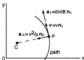
FIGURE 1.3.4 Tangential and normal components. C is the center of curvature.
