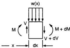
**FIGURE 1.2.25** Internal reactions in a beam under distributed loading.
