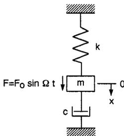
**FIGURE 1.4.2** Model of a damped vibrating system.
