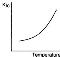
FIGURE 1.6.9 Temperature effect on toughness.
