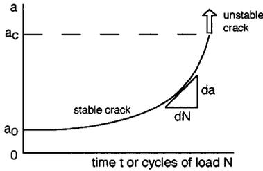
FIGURE 1.6.11 Crack growth rates under constant load.
