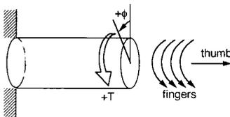
FIGURE 1.5.26 Right-hand rule for positive torque and angle.
