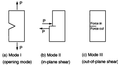
**FIGURE 1.6.3** Modes of deformation.
