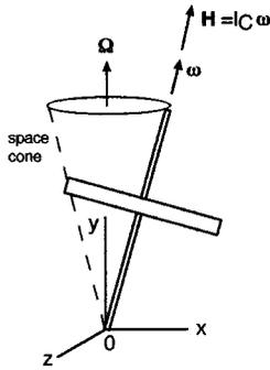
FIGURE 1.3.22 Motion of an inclined, spinning top.
