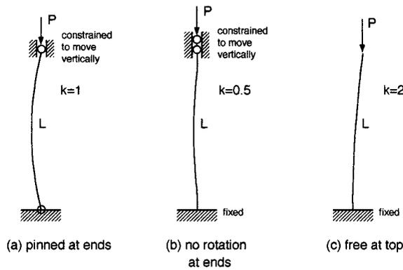
FIGURE 1.5.29 Common end conditions of slender columns.
