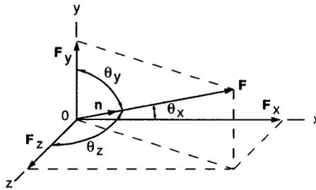
**FIGURE 1.2.5** Three-dimensional components of a vector  $\mathbf{F}$ .
