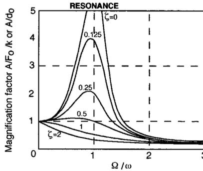
FIGURE 1.4.3 Magnification factor in damped forced vibration.
