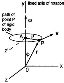
FIGURE 1.3.10 Rigid body rotating about a fixed axis.
