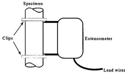
**FIGURE 1.5.38** Extensometer attached to a tensile specimen.
