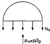
FIGURE 1.5.33 Analysis of spherical pressure vessels.
