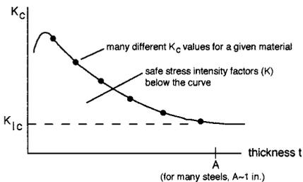
FIGURE 1.6.6  $K_{Ic}$  = plane strain fracture toughness of material.
