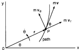
**FIGURE 1.3.8** Definition of angular momentum for a particle.
