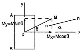
FIGURE 1.5.18 Schematic of arbitrary bending moment.
