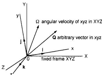
FIGURE 1.3.17 Time derivative of a vector using a rotating reference frame.
