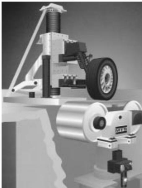
**FIGURE 1.1.1** Artist's concept of a moving stainless steel roadway to drive the suspension system through a spinning, articulated wheel, simulating three-dimensional motions and forces. (MTS Systems Corp., Minneapolis, MN. With permission.) Notes: Flat-Trac® Roadway Simulator, R&D100 Award-winning system in 1993. See also Color Plate 1.\*
