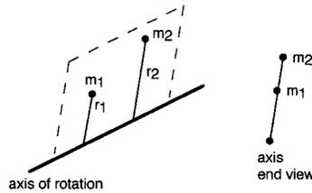
FIGURE 1.4.5 Schematic of static unbalance.
