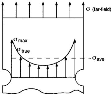
**FIGURE 1.6.1** Stress distribution (simplistic) in a notched member under uniaxial load.
