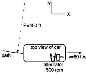
FIGURE 1.3.16 Schematic of shaft's motion.
