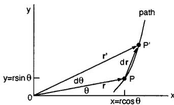
FIGURE 1.3.5 Motion of a particle in polar coordinates.
