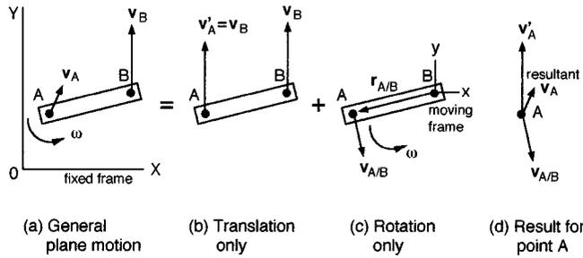
FIGURE 1.3.11 Analysis of velocities in general plane motion.
