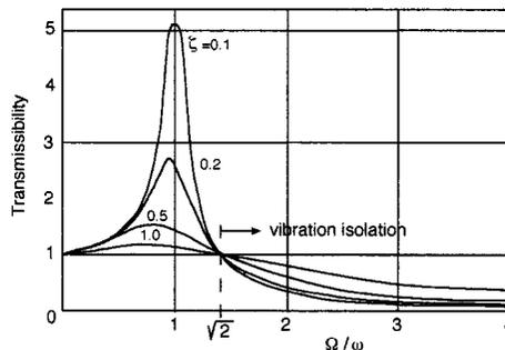
FIGURE 1.4.4 Transmissibility patterns of a vibration isolator.
