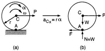
FIGURE 1.3.19 Pure rolling of a wheel.
