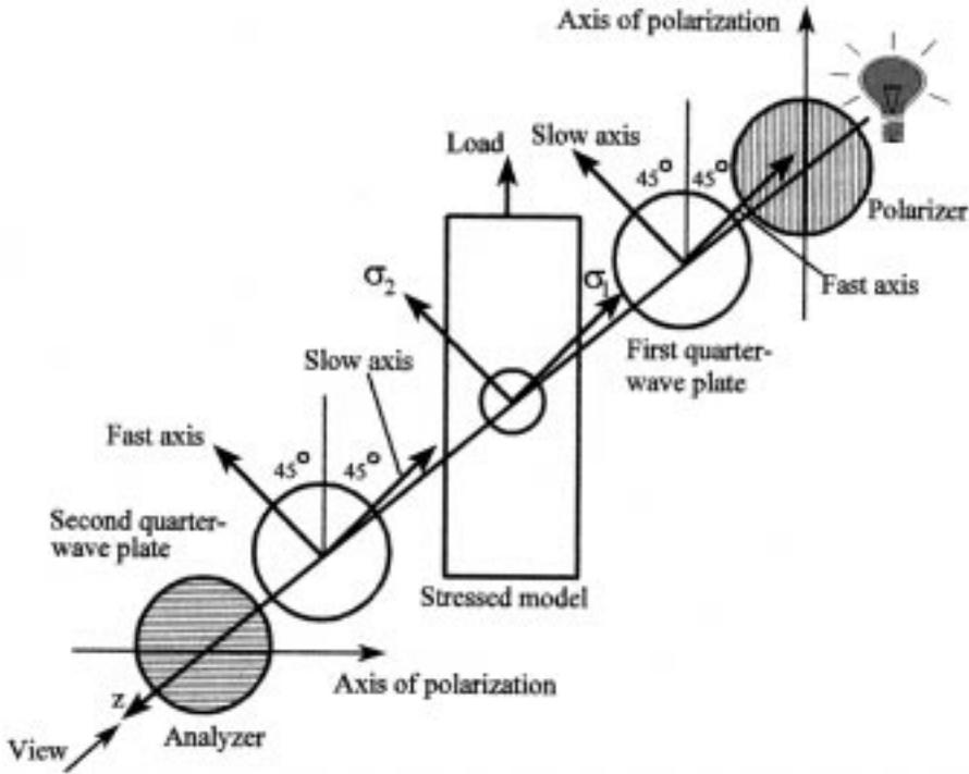
FIGURE 1.5.43 Schematic of a stressed photoelastic model in a circular polariscope.
