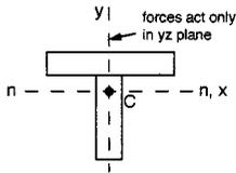
FIGURE 1.5.17 Neutral axis of a semisymmetric area.
