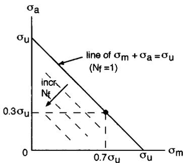
FIGURE 1.6.19 Schematic of tensile mean stress effect.
