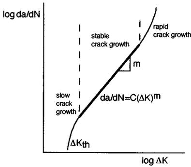
FIGURE 1.6.28 Schematic of fatigue crack propagation data.
