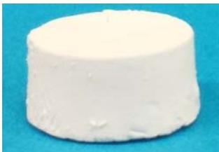
Figure 3: SF+AA aerogel picture.
