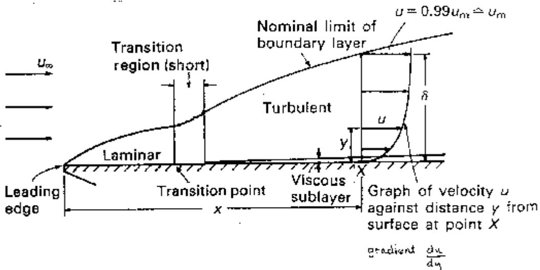
We define the thickness of this boundary layer as the distance from the wall to the point where the velocity is 99% of the “free stream” velocity, the velocity in the middle of the pipe or river.
