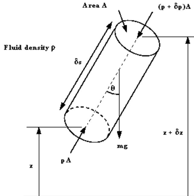
A cylindrical element of fluid at an arbitrary orientation.
