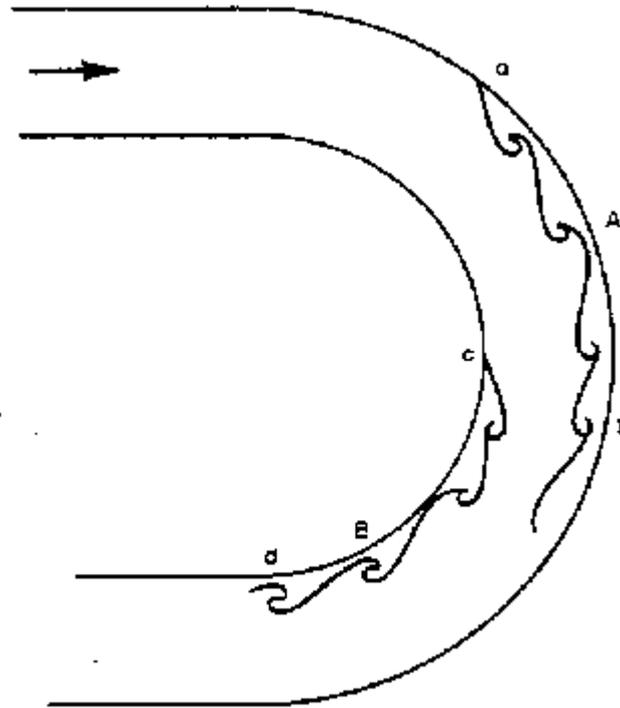
Two separation zones occur in bends as shown above. The pressure at b must be greater than at a as it must provide the required radial acceleration for the fluid to get round the bend. There is thus an adverse pressure gradient between a and b so separation may occur here.
