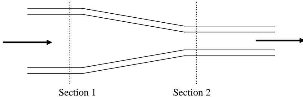
A liquid is flowing from left to right and the pipe is narrowing in the same direction. By the continuity principle, the *mass flow rate* must be the same at each section - the mass going into the pipe is equal to the mass going out of the pipe. So we can write:
