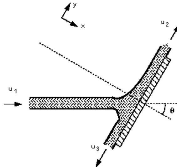
A jet hitting an inclined plane.
