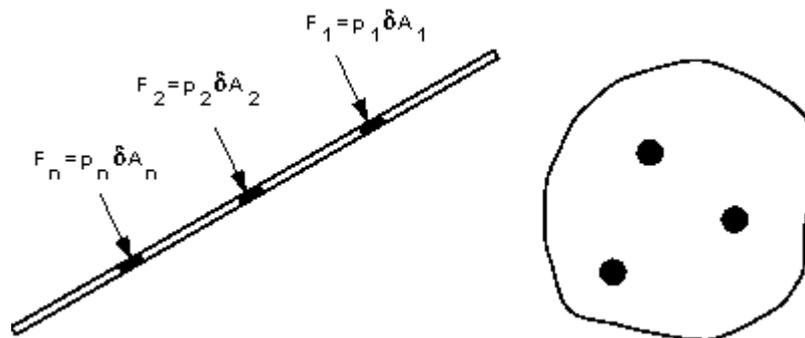
We can find the total or **resultant** force,  $R$ , on the plane by summing up all of the forces on the small elements i.e.
