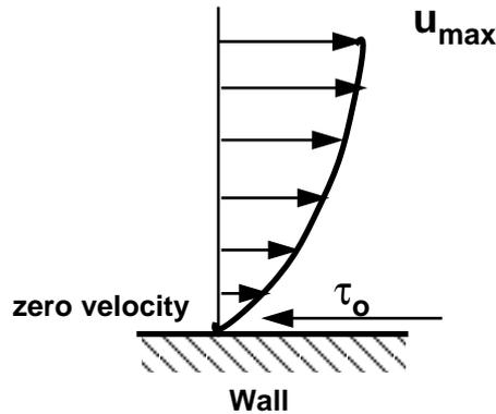
Looking at this two-dimensionally we get the above velocity profile from the wall to the centre of the flow.
