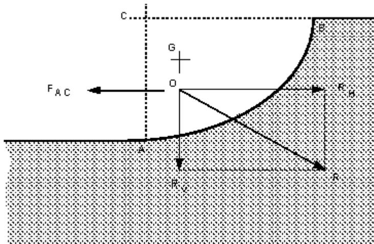
The calculation of the forces acting from the fluid below is very similar to when the fluid is above.
