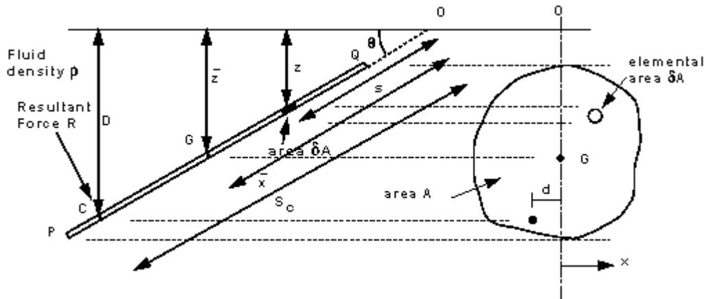
This plane surface is totally submerged in a liquid of density  $\rho$  and inclined at an angle of  $\theta$  to the horizontal. Taking pressure as zero at the surface and measuring down from the surface, the pressure on an element  $\delta A$ , submerged a distance  $z$ , is given by
