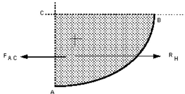
We can see that the horizontal force on AC,  $F_{AC}$ , must equal and be in the opposite direction to the resultant force  $R_H$  on the curved surface.
