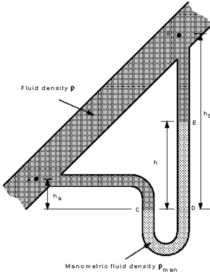
Pressure difference measurement by the “U”-Tube manometer
