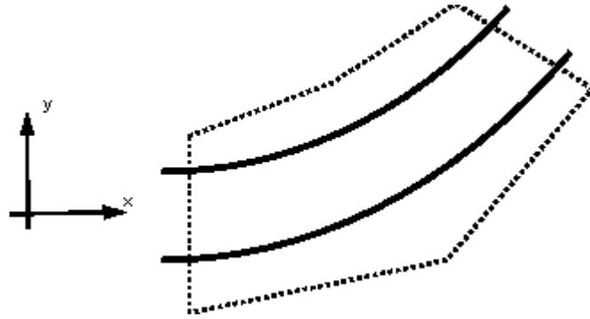
The control volume is drawn in the above figure, with faces at the inlet and outlet of the bend and encompassing the pipe walls.
