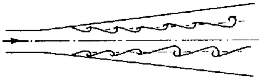
Increasing the angle of the diffuser increases the probability of boundary layer separation. In a Venturi meter it has been found that an angle of about  $6^\circ$  provides the optimum balance between length of meter and danger of boundary layer separation which would cause unacceptable pressure energy losses.
