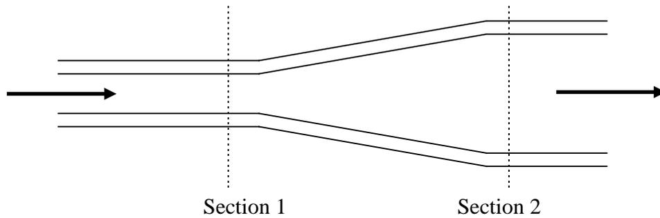
If the diameter at section 1 is  $d_1 = 30\text{mm}$  and at section 2  $d_2 = 40\text{mm}$  and the mean velocity at section 2 is  $u_2 = 3.0\text{m/s}$ . The velocity entering the diffuser is given by,
