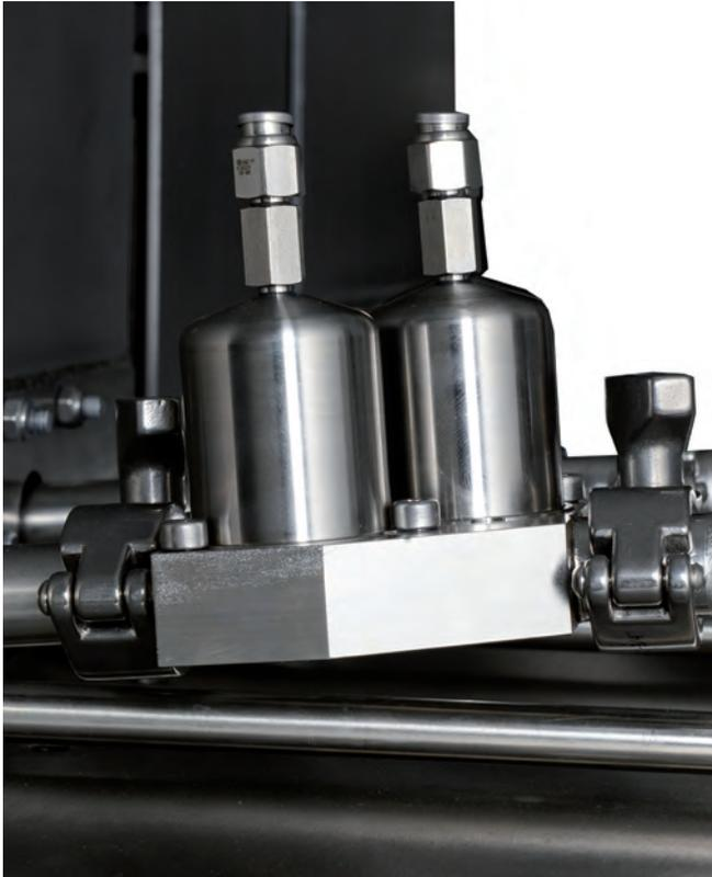
*A double valve allows to the filler to reach high speed.*
