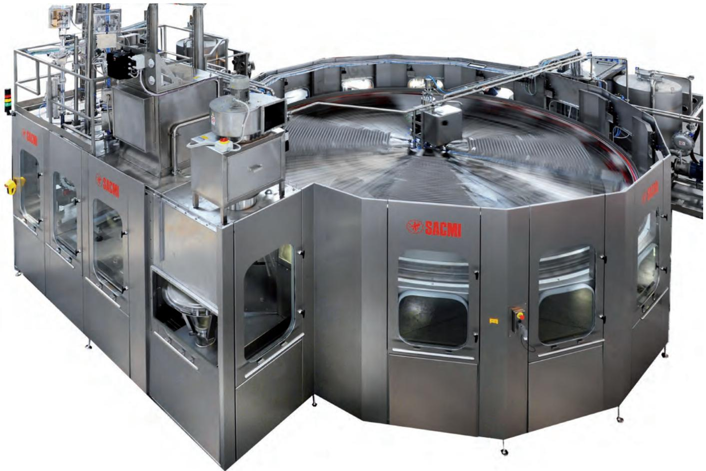
The electronic filling operation allows to monitor every single valve, sensing in real time its performance and any malfunction which may occur. It also allows to modify from the operator panel the fill level in the bottle.
