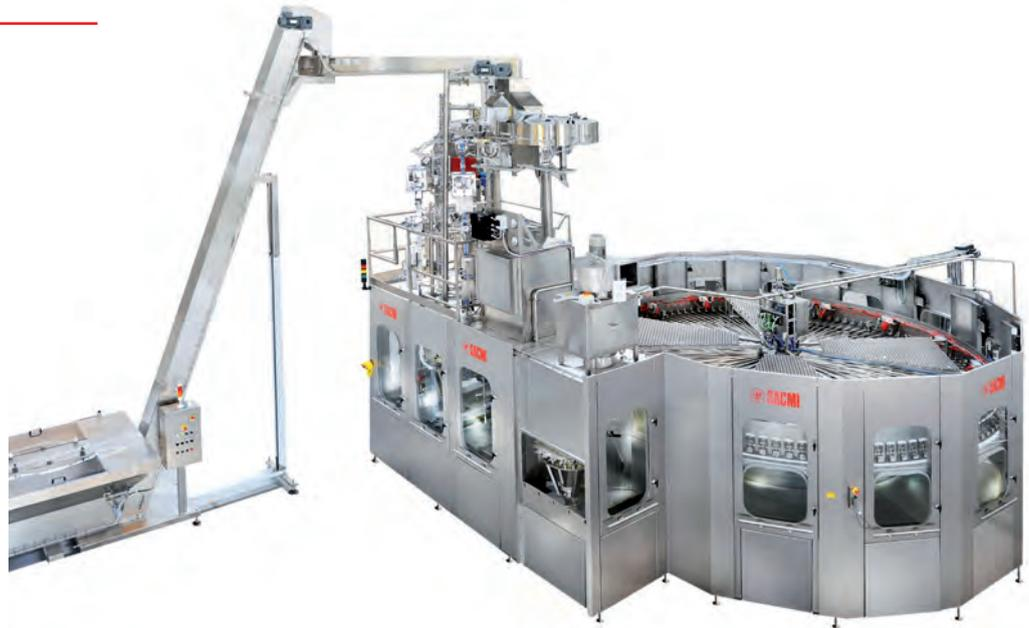
**EN** Monoblock can be equipped with cappers for both flat and sport plastic screw caps, aluminium screw caps, crown caps and pressure caps. This extremely flexible solution also enables two capping towers to be installed upon request, which is particularly recommended if the system is able to handle both glass and PET bottles.
