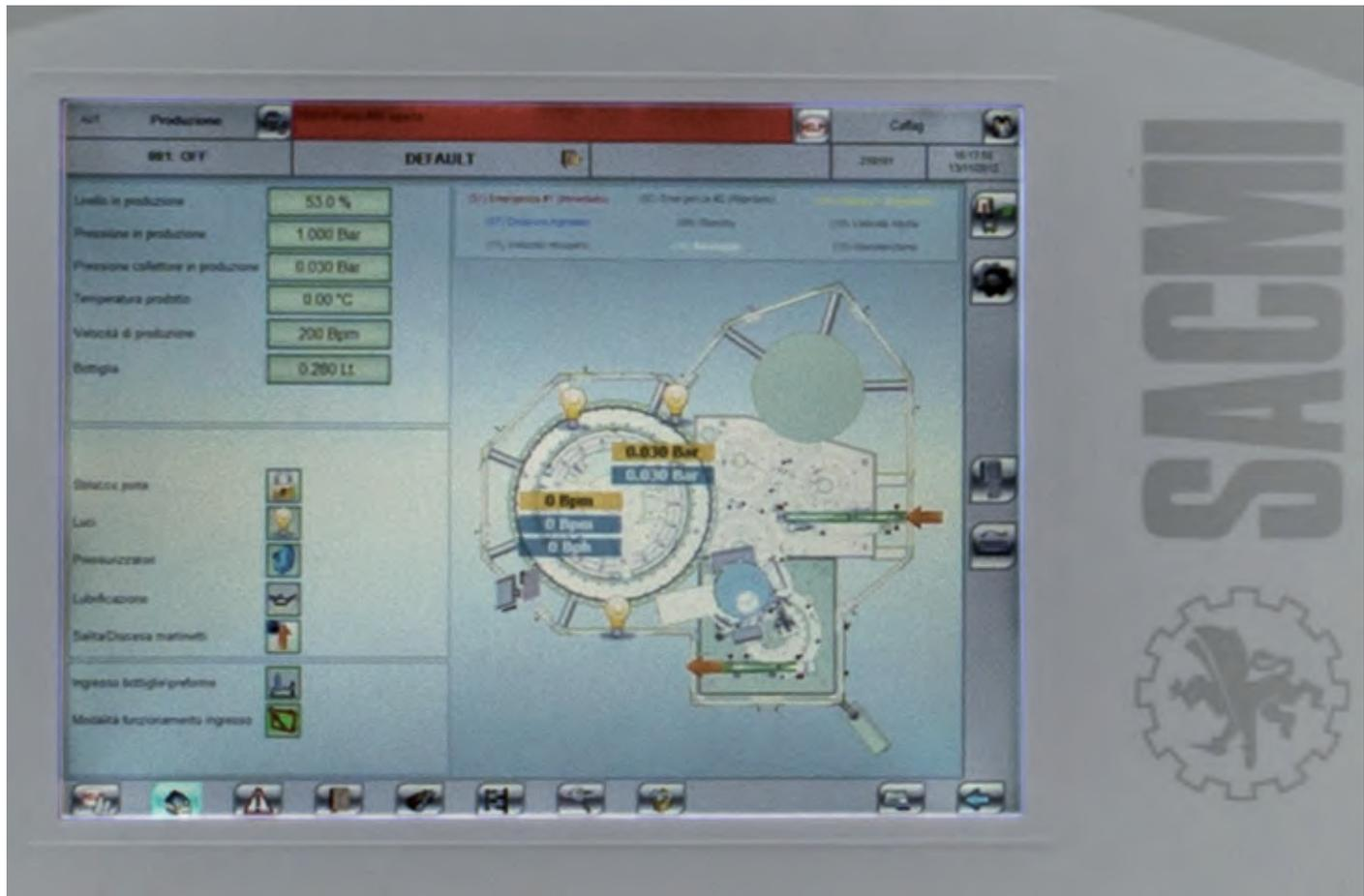
**EN** All system parameters are controlled by dedicated software, and adjusted using a touch screen. There is also the option of a model that can record and analyse alarms, efficiency and production data and working parameters, with the possibility of exporting this data to the company management system.
