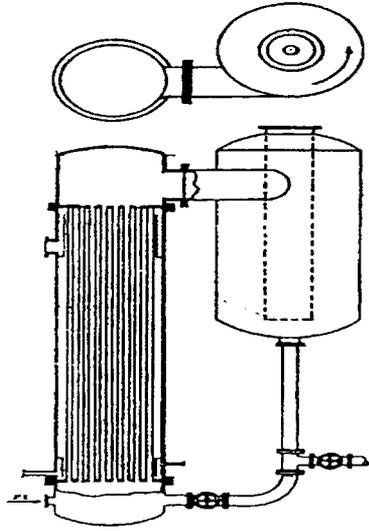
Figure 5. Natural circulation, long tube film evaporator.
