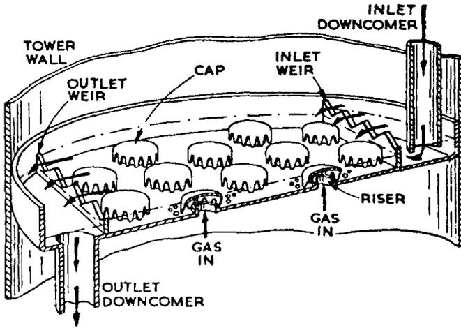
Figure 4. Bubble cap tray configuration.
