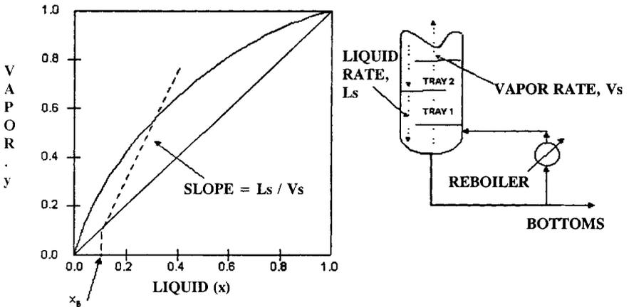
Figure 14. Construction of operating line for stripping section.
