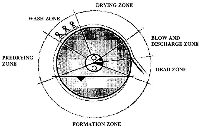
Figure 13. Cycle sequence of a rotary drum filter.
