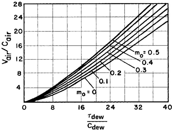
Figure 39. Volume of blowing air vs. dewatering time.
