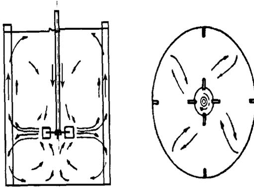
Figure 8. Axial flow patterns in a tank.
