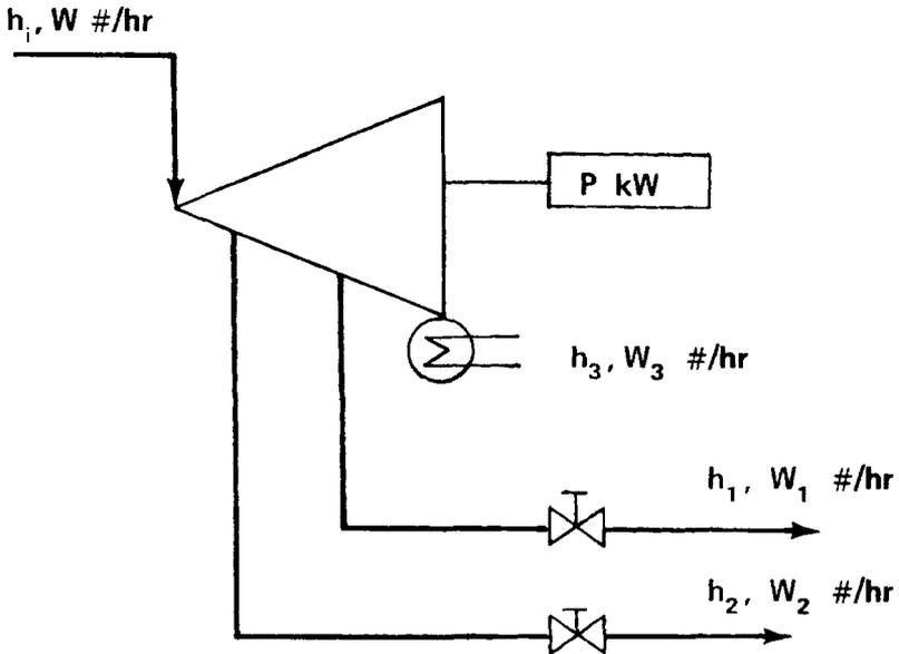
Figure 6. Simplified diagram for back-pressure turbine analysis.
