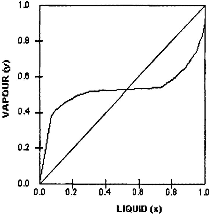
Figure 12. VLE curve for a heterogeneous azeotropic system.
