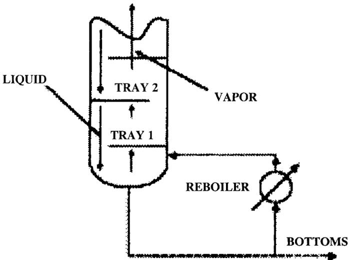
Figure 2. Diagram shows role of the reboiler.
