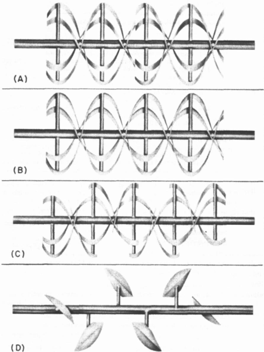
**Figure 4.** Ribbon blender agitator configurations: (A) continuous ribbon, arranged for center discharge; (B) continuous ribbon arranged for end discharge; (C) interrupted ribbon; (D) paddle-type ribbon.
