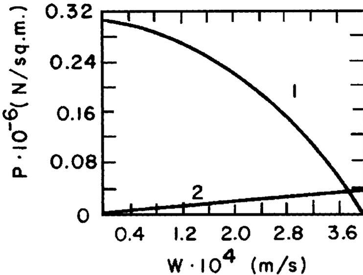
Figure 35. Characteristic pump curve (1) and liquid static pressure on the boundary between the cake and filter plate (curve 2).
