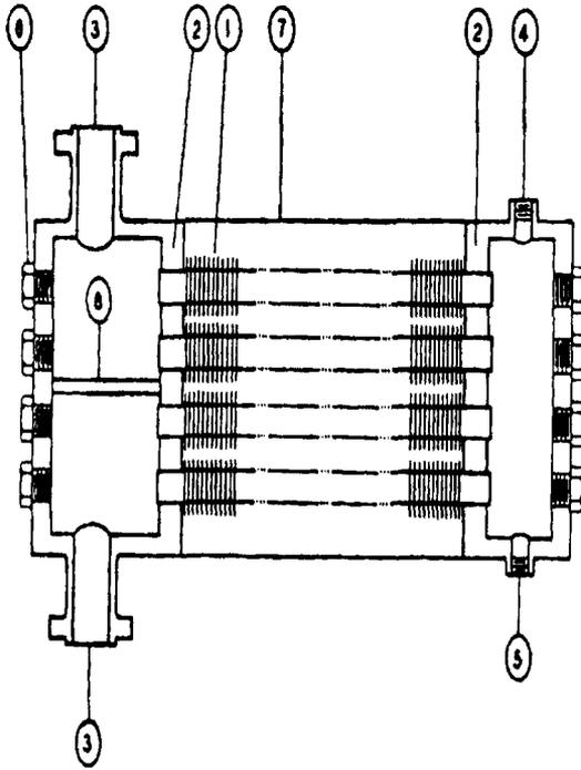
**Figure 2.** *Typical tube bundle (two pass) using box headers with tube plugs opposite each tube end. Key: (1) Tube; (2) Tube Sheet; (3) Inlet/Outlet Nozzles; (4) Vent; (5) Drain; (6) Tube Plugs; (7) Side Frame; (8) Pass Rib .*
