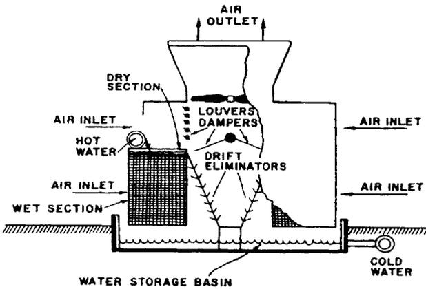
Figure 5. Single structure type wet-dry cooling tower.
