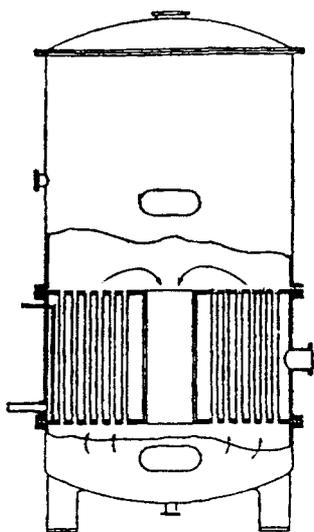
Figure 2. Vertical evaporator.
