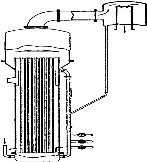
Figure 6. Natural circulation, long tube-vertical film evaporator.
