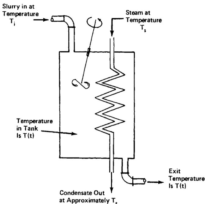
Figure 7. System diagram for heated mixing tank.
