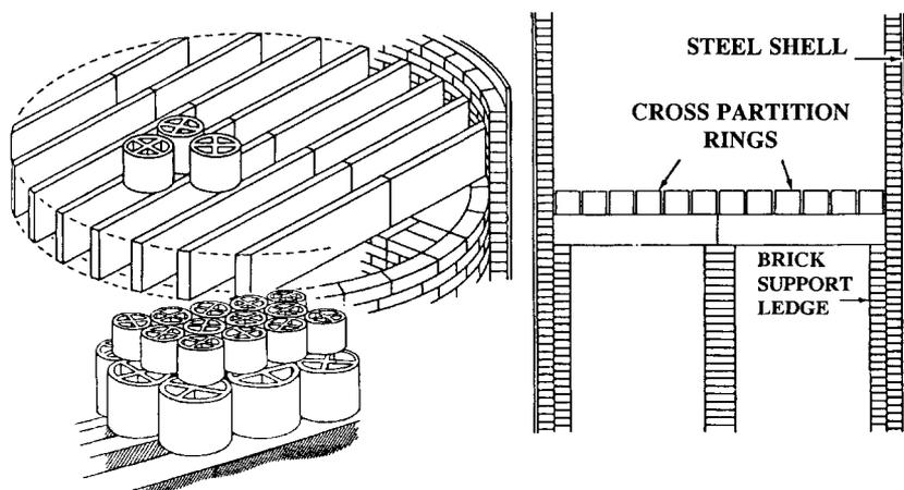
Figure 14. Cross-partition rings used as packing supports.
