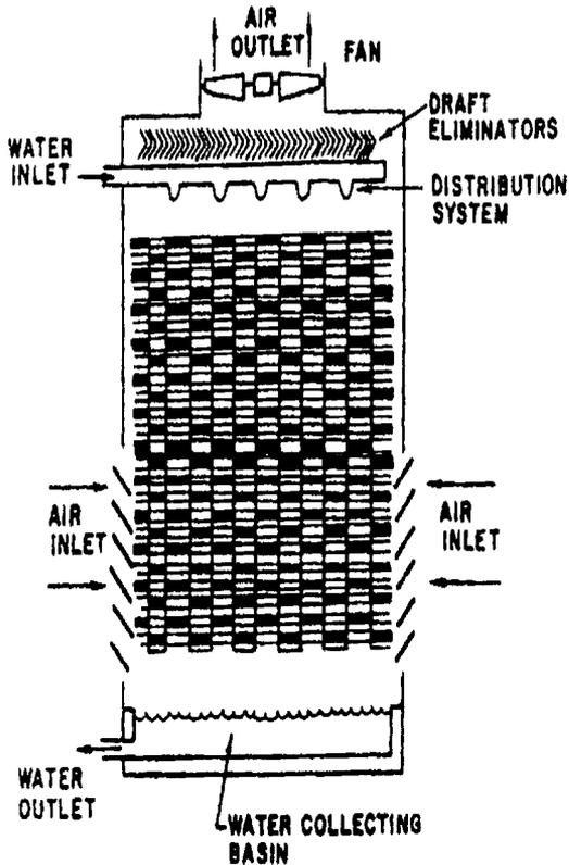
Figure 3. Counterflow cooling tower.
