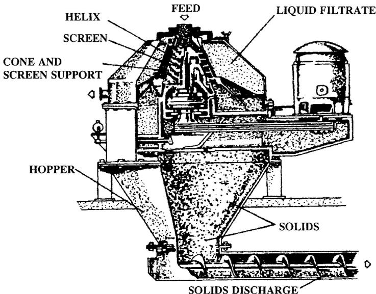
Figure 28. Cutaway view of filter centrifuge.
