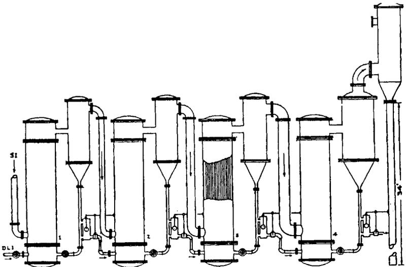
Figure 8. *Quadruple effect, natural circulation vertical tube evaporator.*
