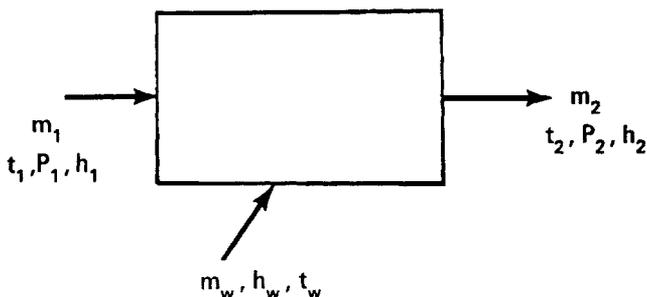
Figure 4. Mass and energy balance for desuperheater system.
