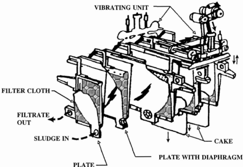
Figure 26. Cake discharge from a diaphragm filter press.
