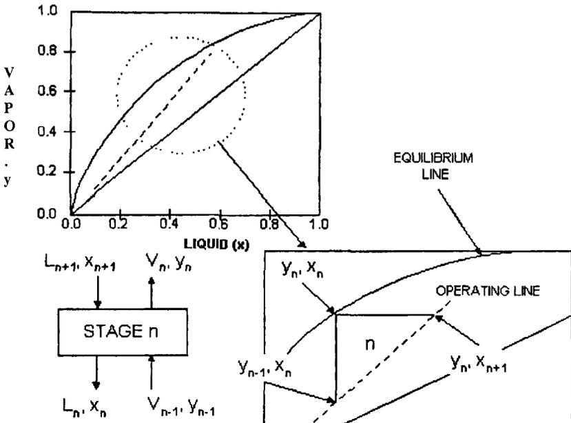
Figure 15. Illustrates the construction of an operating line.
