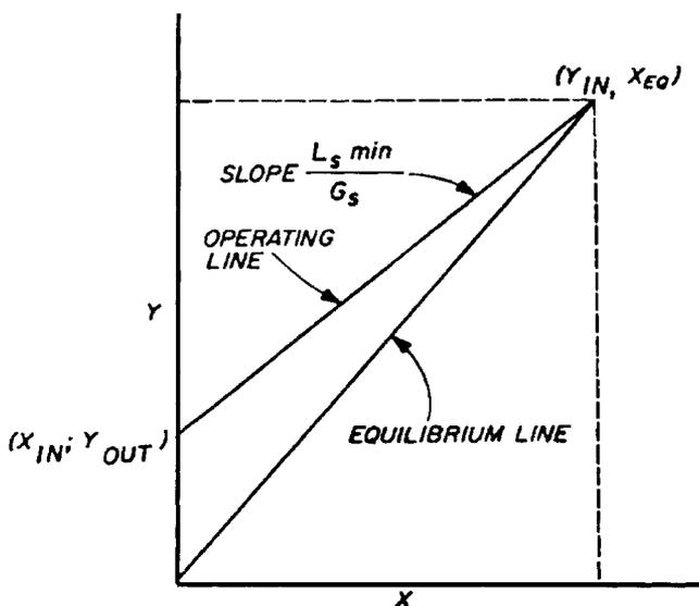
Figure 10. Operating line for absorption.
