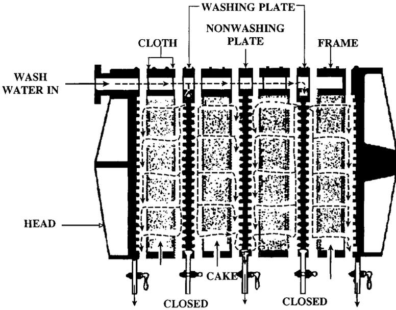
Figure 18. Wash water outlets on a filter press.
