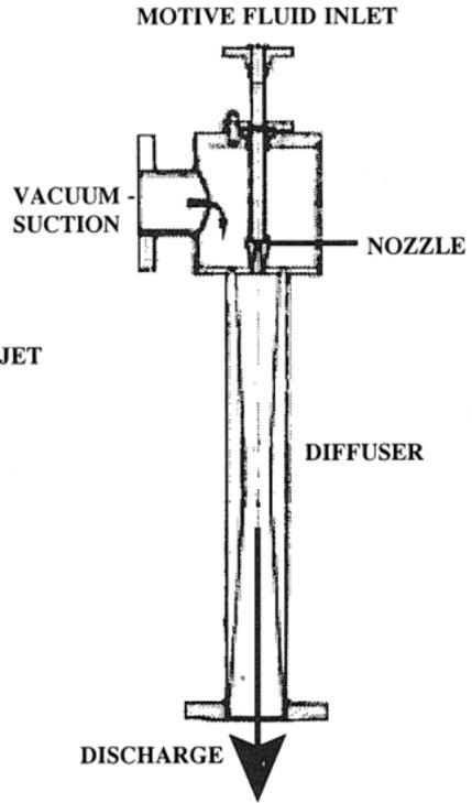
Figure 17. Jet vacuum pump.
