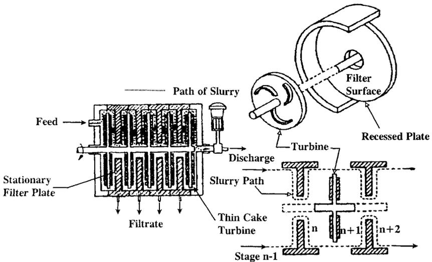
Figure 27. Components of a staged, thin-film filter/thickener.
