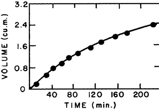
Figure 37. Volume versus filtration time.
