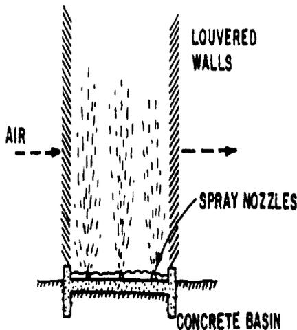
Figure 7. Simple configuration.
