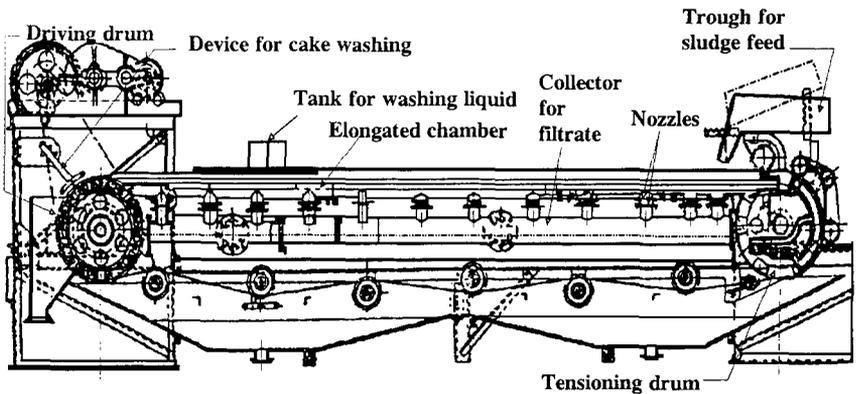
Figure 16. Basic design features of a belt filter.
