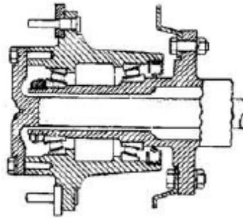
**Fig. Fully floating axle.**
