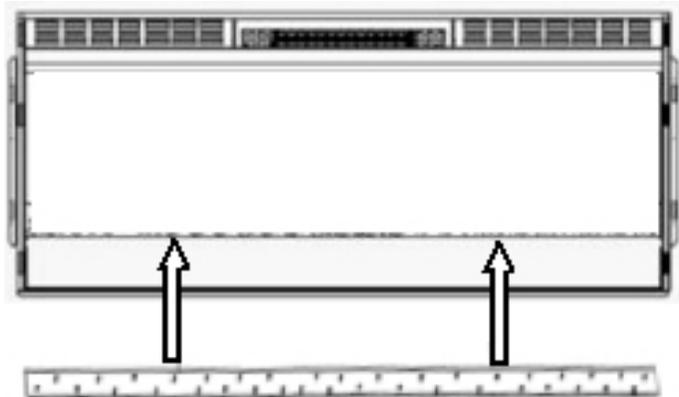
2. Carefully, place crystal embers on plastic strip as illustrated in the picture to the right. Apply an even layer from side to side.
