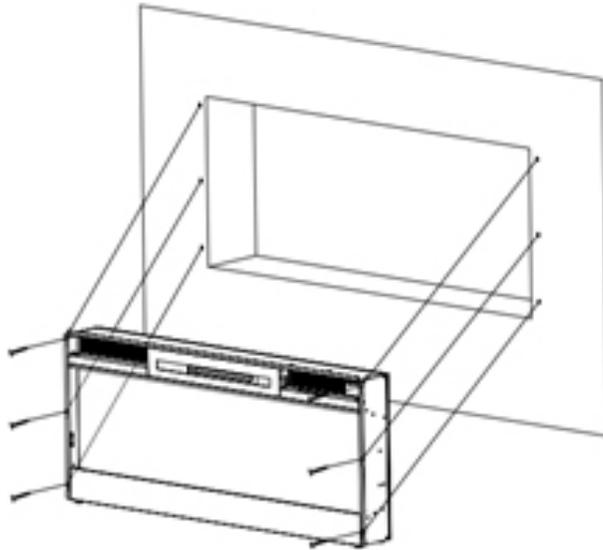
4. Once the fireplace is installed in the wall, place crystal embers or fire log in the fireplace.
