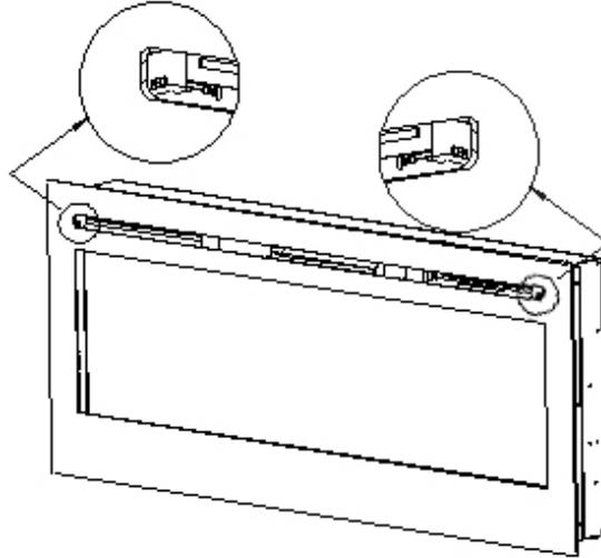
2. After removing screws, lift glass panel UP and STRAIGHT OUT toward you to remove from fireplace. Place glass panel in a soft, dry place.
