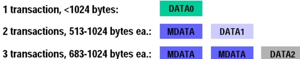
Figure 28 - Data Phase PID Sequence for Isochronous OUT endpoints
