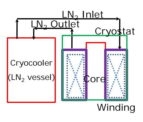
Superconducting transformers and generators have coils (and cores sometimes) maintained at low temperature to minimize the I<sup>2</sup>R (copper) losses.
