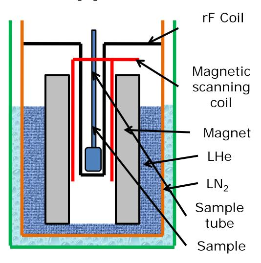
It has a superconducting magnet (10 T ~ 25 T) and the accuracy of measurement increases with field strength.
