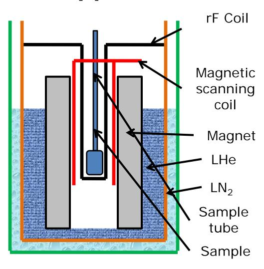
The NMR (Nuclear Magnetic Resonance) is used by the pharmaceutical industry to study the molecular structure.
