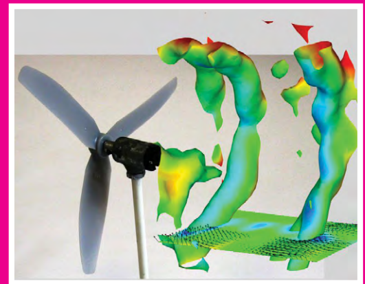
Wake downstream of a water turbine with flow from left to right. Slices represent streamwise velocity, with Red indicating high speed and Blue representing low speed fluid, University of Minnesota, USA
