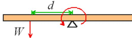
A force applied to a pivoted beam causes the beam to rotate
