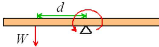
A force applied to a pivoted beam causes the beam to rotate
