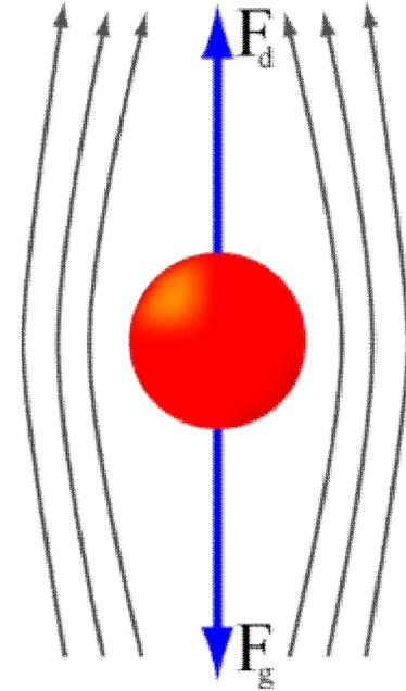
An object moving through a fluid experiences a force in direction opposite to its motion. Terminal velocity is achieved when the drag force is equal in magnitude but opposite in direction to the force propelling the object.
