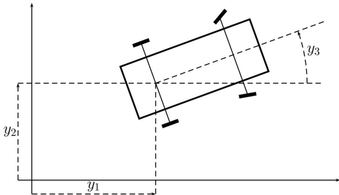
$$\dot{y}_1 = u_1 \cos y_3, \quad \dot{y}_2 = u_1 \sin y_3, \quad \dot{y}_3 = u_2, \quad n = 3, \quad m = 2.$$
