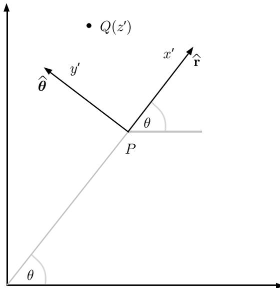
**Figure 2.19:** Let  $Q$  be  $z$  relative to  $Oxy$  and  $z'$  relative to  $Ox'y'$ .
