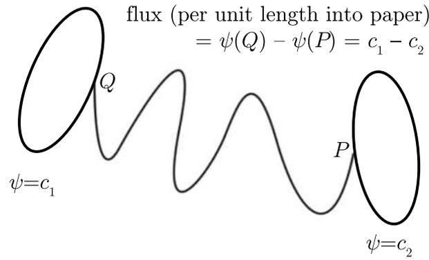
**Figure 1.17:** Flux between two points
