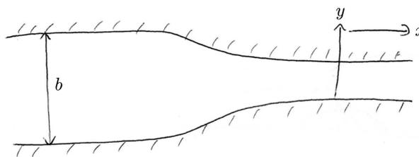
**Figure 3.27:** Plan view of a channel with variable width.
