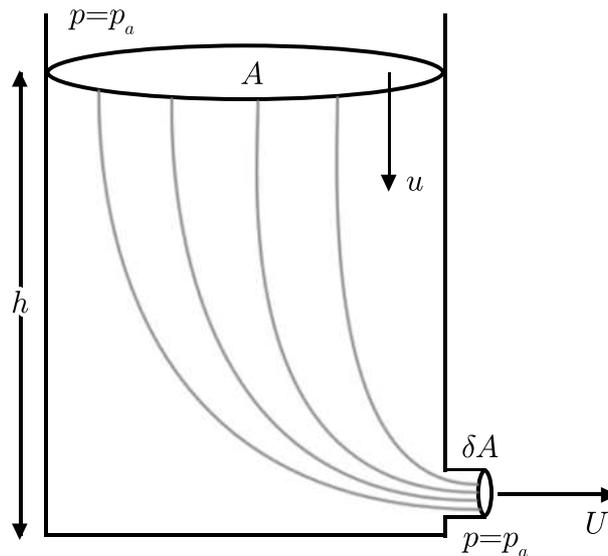
**Figure 3.9:** Our cup with a hole in the bottom, from Example 3.5. The streamlines are tangent to the velocity field and are marked in grey.
