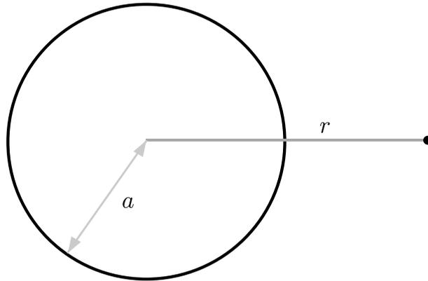
**Figure 2.31:** The optical image is at  $a^2/r$  along some line from the origin.
