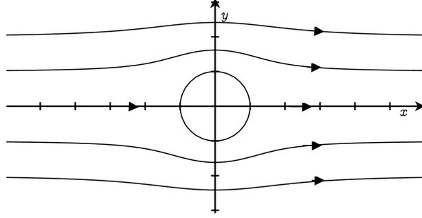
**Figure 2.7:** A plot of the streamlines of the flow in Example 2.11
