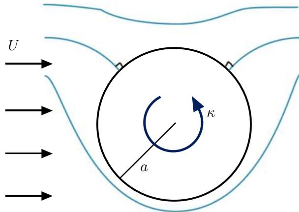
Figure 3.10: A spinning cylinder in a uniform stream.
