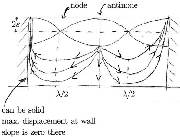
**Figure 4.8:** The walls can be solid. The maximum displacement is at the wall, where the slope is zero.
