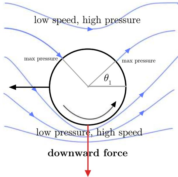
**Figure 2.21:** The ball is travelling right-to-left with topspin.  $0 \leq s \leq 1$ .
