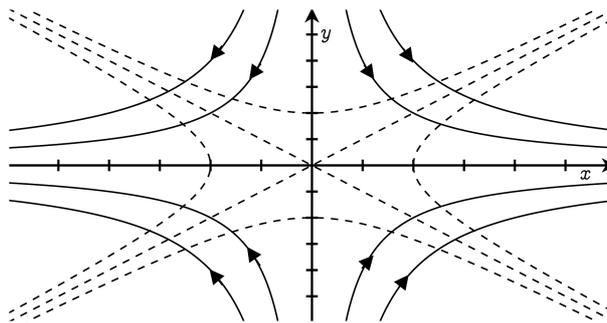
**Figure 2.4:** Plot of the streamlines and equipotential lines from example 2.6
