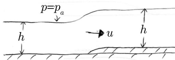
Figure 3.17: Elevation view of a channel of variable width
