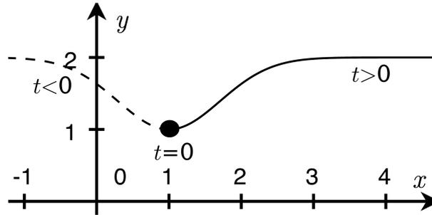
**Figure 1.6:** Plot of the Streakline for this flow
