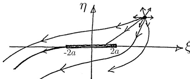
Figure C.27: Solution to Sheet 10, Q2. Streamlines are radial at source.
