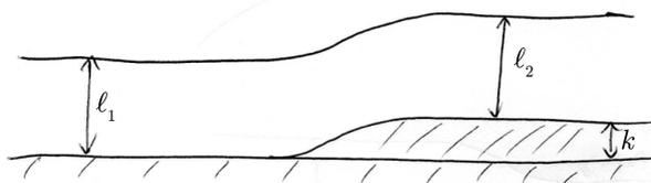
**Figure 3.23:** For flow over a ridge, there are two cases, depending on the value of  $F$ .
