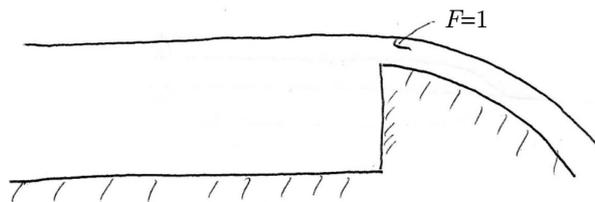
**Figure 3.26:** In a weir, the critical point, where  $F = 1$ , is directly above the edge of the top of the spout.
