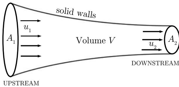
**Figure 1.10:** Fluid of constant density flows through this pipe
