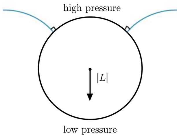
**Figure 3.14:** Pressure effects on the cylinder.
