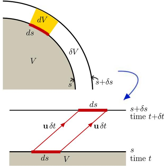
**Figure 3.2:** In time  $\delta t$  a particle moves a displacement  $\mathbf{u} \delta t$ . Thus a small element of area  $dS$  sweeps out a sliced cylinder with volume  $dV = \text{area of base} \times \text{height}$ .
