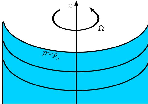
**Figure 3.6:** Paraboloids of revolution
