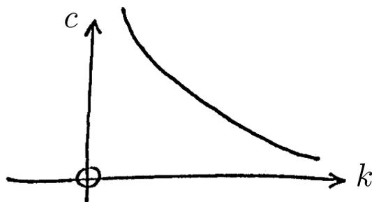
**Figure C.13:** Solution to Sheet 6, Q1d where  $\sigma = 0$ . Graph of  $c = \left(\frac{g}{k}\right)^{1/2}$ .
