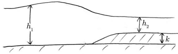
**Figure 3.21:** We start with a deep, slow flow with a high surface: low KE and high PE. We end with a shallow, fast flow with a lower surface, i.e. it converts some PE into KE to get over the bump.
