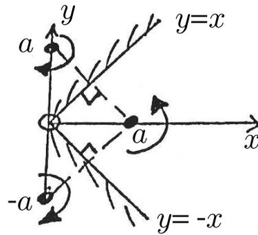
**Figure C.10:** Solution to Sheet 5, Q1. Diagram of image vortices.
