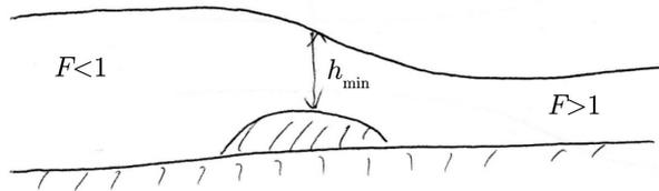
**Figure 3.25:** We observe a transition between  $F < 1$  and  $F > 1$ . The critical point is directly above the centre of the lump.
