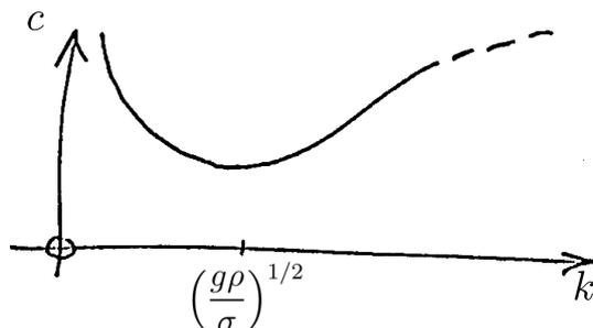
**Figure C.14:** Solution to Sheet 6, Q1d, where  $\sigma \neq 0$ . As  $k \rightarrow \infty$ ,  $c \sim \left(\frac{\sigma k}{\rho}\right)^{1/2}$ .
