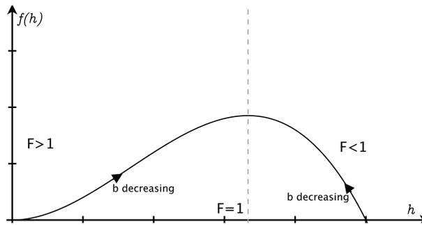
**Figure 3.29:** For a particle on the left-hand side,  $b$  decreasing leads to the flow deepening. For a particle on the right-hand side,  $b$  decreasing leads to the flow getting shallower.
