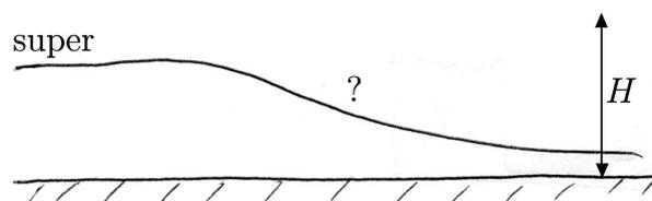
**Figure 3.35:** The depth smoothly increases to 0 as  $b \rightarrow \infty$ . Over on the left we have supercritical flow. No waves can travel upstream since  $U > \sqrt{gh}$ .
