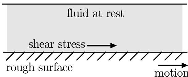
**Figure 1.2:** Inviscid fluids cannot support shear stress.
