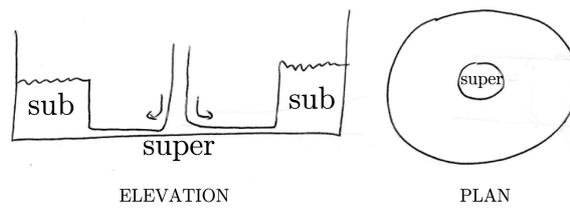
**Figure 3.39:** *Left:* If you turn the tap on in a sink (an actual sink), you see supercritical flow under the tap, and subcritical flow at the sides. *Right:* Top-down view of the sink.
