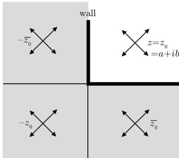
**Figure 2.27:** A source of strength  $m$  sits in the first quadrant at  $z_0$  with walls ( $x = 0, y > 0$ ) and ( $y = 0, x > 0$ )
