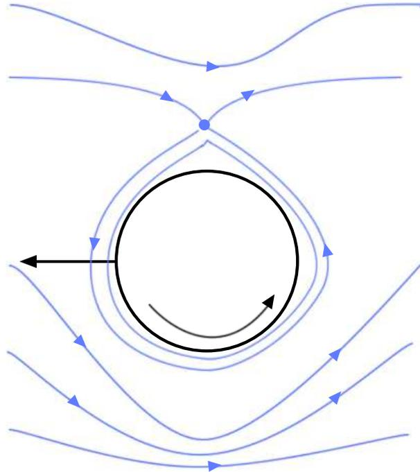
**Figure 2.23:** The ball is travelling right-to-left with topspin.  $s > 1$ .
