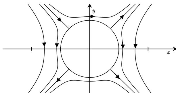
**Figure 2.10:** A plot of the streamlines of the flow in Example 2.12
