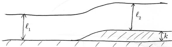
**Figure 3.22:** We start with a shallow, fast flow with a low surface: low PE and high KE. We end with a deeper, slower flow and a high surface: high PE and low KE.
