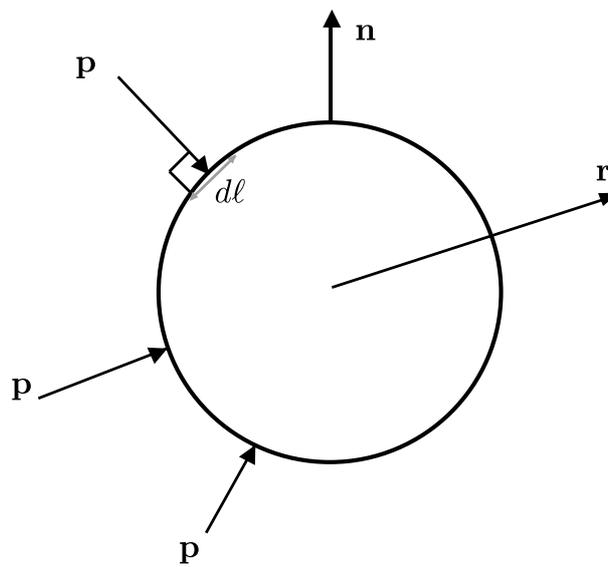
Figure 3.11: Pressure acts normal to the wall of the cylinder, in the  $-\hat{\mathbf{n}} = -\hat{\mathbf{r}}$  direction.
