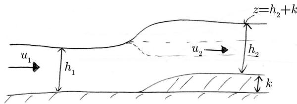
**Figure 3.19:** Will the surface rise, fall or stay level if we raise the floor of the channel?
