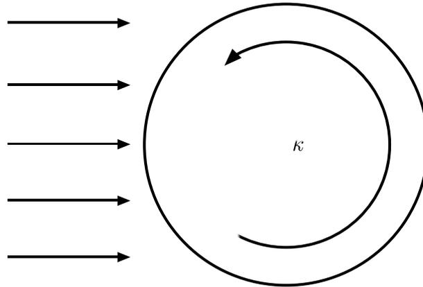
**Figure 2.18:** A cylinder with circulation  $\kappa$  in a flow that at infinity has velocity  $U$  in the  $x$ -direction
