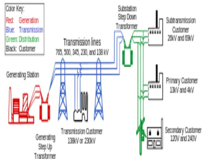
**Figure 2: Simplified diagram of AC electricity delivery from generation stations to consumers [12].**
