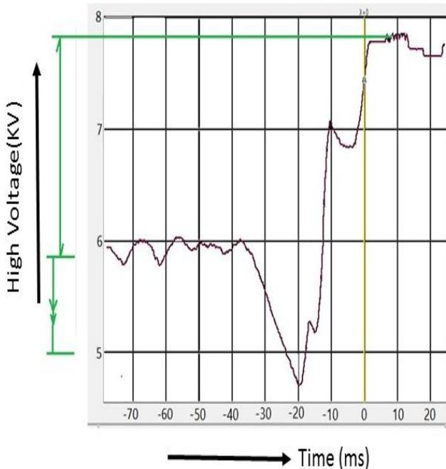
**Figure 6: High voltage in KV versus time for 11 KV input for the tested VSD.**
