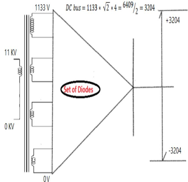
**Figure 5: Simplified diagram of 11 KV input supply to the tested VSD.**
