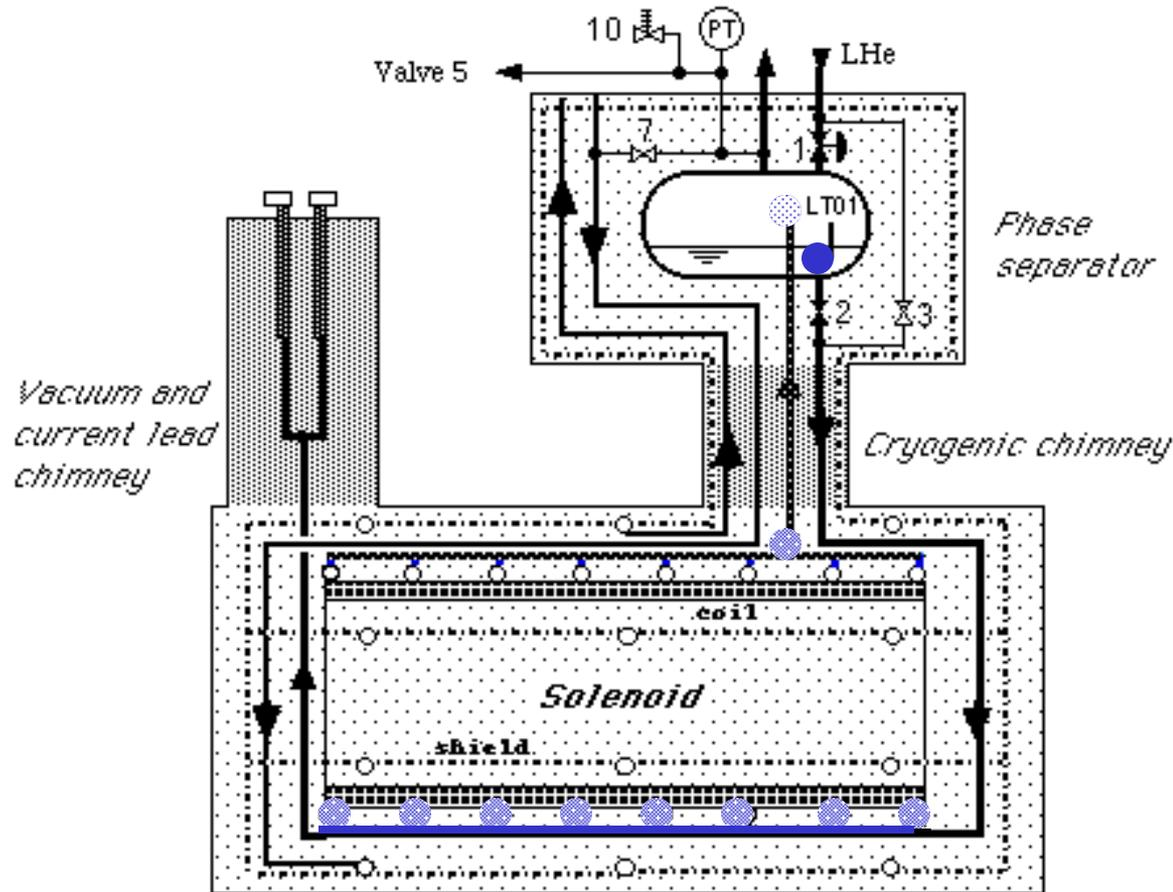
Coil cooling system for CMS detector magnet at CERN-LHC
