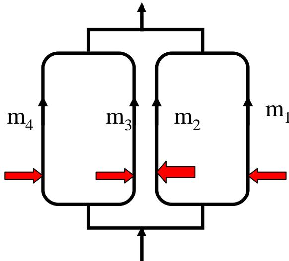
$\Delta p$  is the same for all channels, but vapor mass flow will increase for the channels with higher heat load. This will decrease the mass flow and could lead to "dry out" or vapor lock condition.
