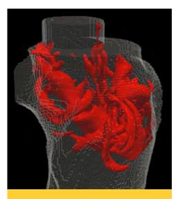
MAE researchers are using computational fluid dynamics (CFD) to improve the design and placement of cardiovascular devices such as artificial heart valves.
