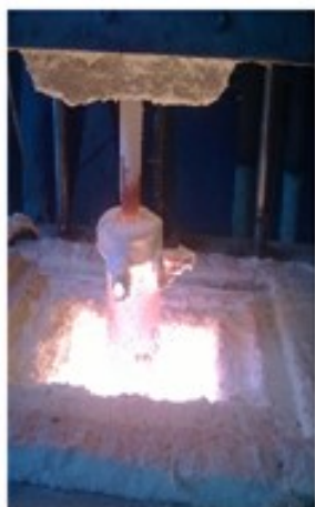
Fig. 2: The cup with liquid metal is taken out from the furnace after gas blowing process.
