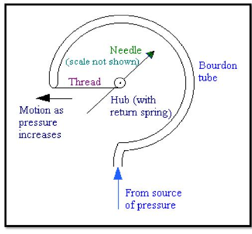
The pressure to be measured is applied to a curved tube, oval in cross section. Pressure applied to the tube tends to cause the tube to straighten out, and the deflection of the end of the tube is communicated through a system of levers to a recording needle. This gauge is widely used for steam and compressed gases. The pressure indicated is the difference between that communicated by the system to the external (ambient) pressure, and is usually referred to as the gauge pressure.
