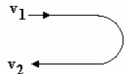
5. A horizontal pipe bend reduces from 300 mm bore diameter at inlet to 150 mm diameter at outlet. The bend is swept through 50° from its initial direction. The flow rate is 0.05 m<sup>3</sup>/s and the density is 1000 kg/m<sup>3</sup>. Calculate the momentum force on the bend and resolve it into two perpendicular directions relative to the initial direction.
