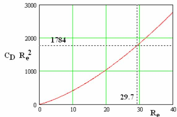
7. A glass sphere of diameter 1.5 mm and density  $2500 \text{ kg/m}^3$  is allowed to fall through water under the action of gravity. Find the terminal velocity assuming the drag coefficient is
