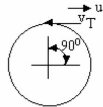
Putting  $r = \text{infinity}$  and  $\theta = 90^\circ$  and remembering that  $+v_T$  is anticlockwise  $+u$  is left to right, we have  $v_T = -3$  m/s.  $B/r^2 \rightarrow 0$
