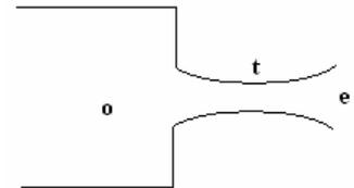
The throat is choked  $\left(\frac{p_t}{p_o}\right) = \left(\frac{2}{\gamma-1}\right)^{\frac{\gamma}{\gamma-1}} = 0.528$
