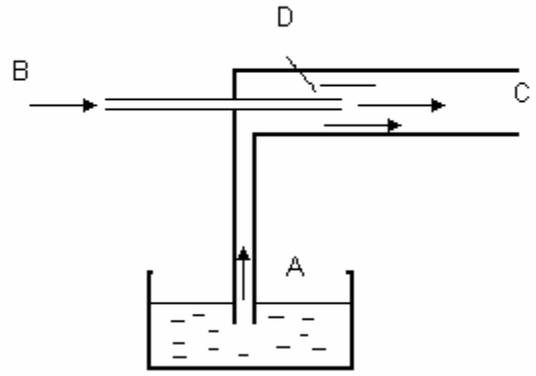
Evaluate the pressure  $p$  at section D, just downstream of the end of pipe B, the velocity in pipe B and the required height of the free water level in the reservoir supplying pipe B. (-21.8 kPa gauge, 12.9 m/s, 6.3 m).
