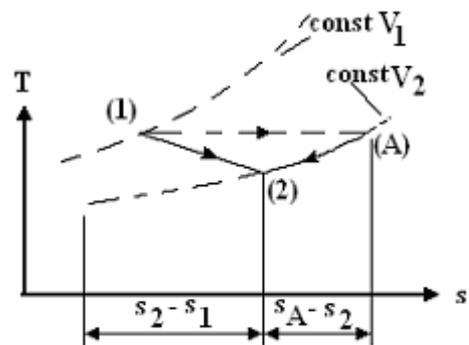
6. A perfect gas is expanded from 5 bar to 1 bar by the law  $pV^{1.6} = C$ . The initial temperature is  $200^{\circ}\text{C}$ . Calculate the change in specific entropy.
