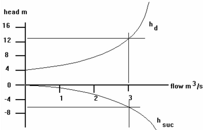
The pump must deliver 3 m<sup>3</sup>/s at 2 000 rev/min. Determine the specific speed.
