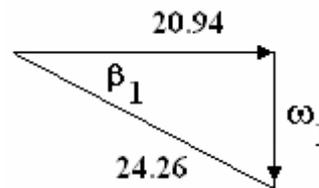
2. A radial flow turbine has a rotor 400 mm diameter and runs at 600 rev/min. The vanes are 30 mm high at the outer edge. The vanes are inclined at 42° to the tangent to the inner edge. The flow rate is 0.5 m<sup>3</sup>/s and leaves the rotor radially. Determine
