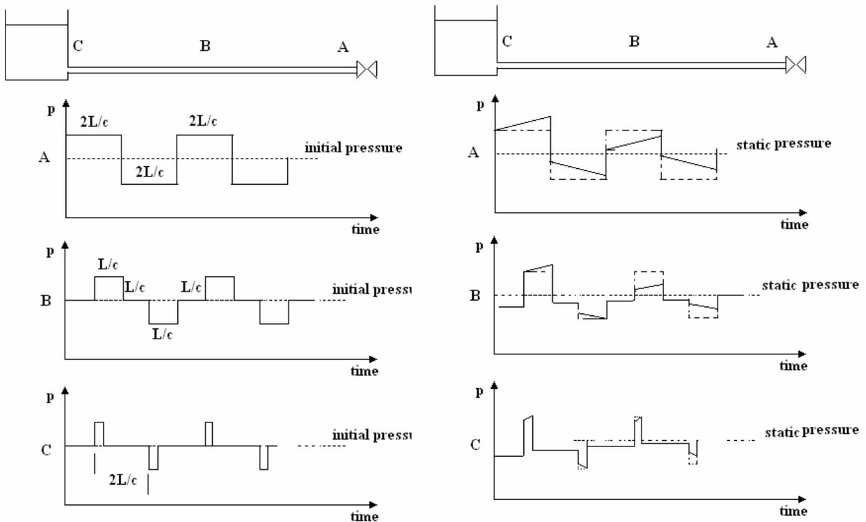
When cavitation occurs the minimum pressure is the vapour pressure so the bottom part of the cycle will be at this pressure.
