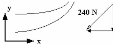
$$F_{py2} = 240 \sin 45^\circ = 169.7 \text{ N} \quad F_{px2} = 240 \cos 45^\circ = 169.7 \text{ N}$$
