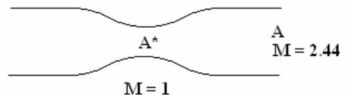
Hence this is a correct solution and this is the theoretical result when m = 0.24 at inlet and 1.0 at the throat.
