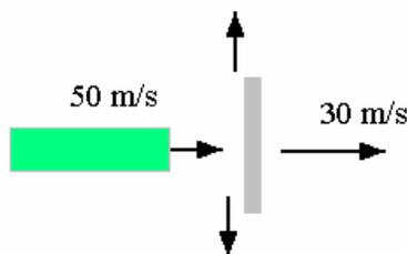
$$\text{Diagram Power} = mu (v - u) = 2.5 \times 30 (50 - 30) = 1500 \text{ Watts}$$
