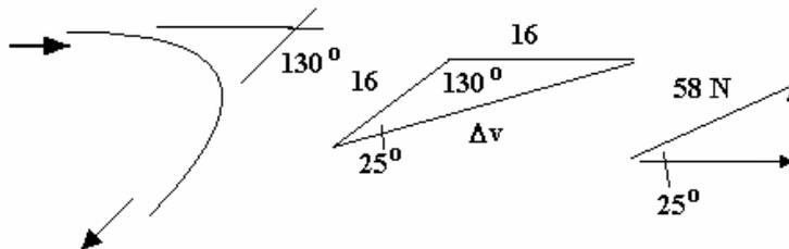
$$\Delta v = 16 \sin 130 / \sin 25 = 29 \text{ m/s} \quad F = m \Delta v = 2 \times 29 = 58 \text{ N}$$
