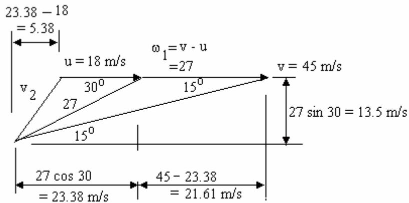
The relative velocity at exit is  $\omega_2 = 27 \text{ m/s}$
