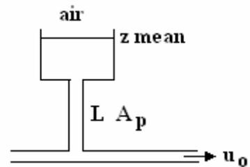
This force decelerates the fluid and the mass decelerated is  $m = \rho A_p L \quad \Delta F = m a$
