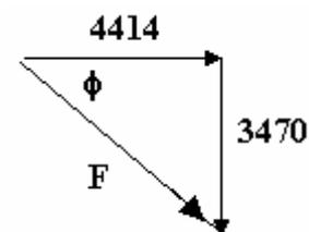
2. A nozzle produces a jet of water. The gauge pressure behind the nozzle is 2 MPa. The exit diameter is 100 mm. The coefficient of velocity is 0.97 and there is no contraction of the jet. The approach velocity is negligible. The jet of water is deflected  $165^\circ$  from its initial direction by a stationary vane. Calculate the resultant force on the nozzle and on the vane due to momentum changes only.
