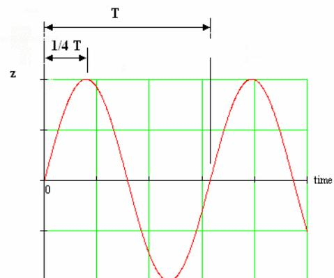
The standard solution to this equation is  $z = z_o \sin(\omega t)$
