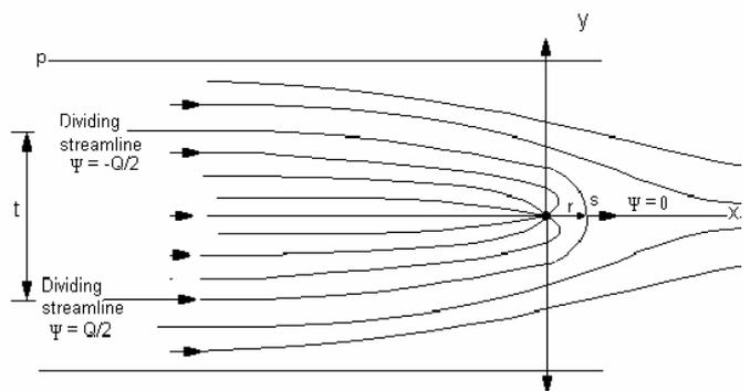
$$\psi_1 = u y \quad \psi_2 = B\theta \quad \psi = u y + B\theta \quad B = Q/2\pi \text{ for a sink}$$
