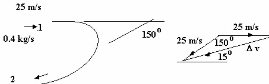
$$\Delta v = 25 \sqrt{2(1 - \cos 150^\circ)} = 48.3 \text{ m/s} \quad F = m \Delta v = 0.4 \times 48.3 = 19.32 \text{ N}$$
