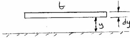
$$d\phi = u b dy = b \left( \frac{dp}{dx} \right) \frac{1}{2\mu} [y^2 - hy] dy$$
