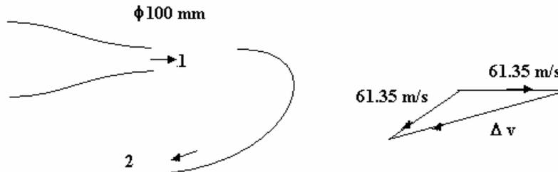
$$v_1 = c_v \sqrt{2\Delta p/\rho} = 0.97\sqrt{2 \times 2 \times 10^6/1000} = 61.35 \text{ m/s}$$
