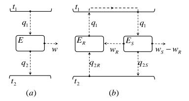
Figure 3.1: (a) An engine E operates between heat reservoirs at temperatures  $t_1$  and  $t_2$ . (b) A perpetual motion machine can be built by coupling a superefficient engine  $E_S$  to a reversible engine  $E_R$ .
