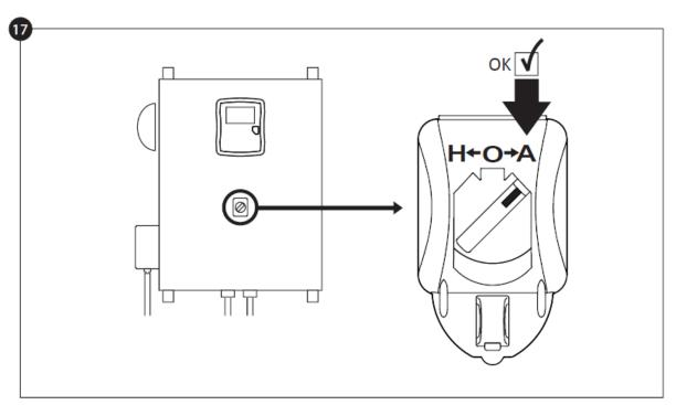
17-Turn the "Main Selector Switch" to the "AUTO" position. This is the preferred position and from now on, the "Main Selector Switch" should always remain in that position.
