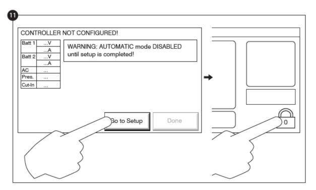
11-Click on the "Go to Setup" button. The "Config" page is now visible. Click on the "padlock" button to log in with your password. If needed, read the "User Login / KeyPad" section for more information on how to enter your password. Once a valid password is confirmed, the "Config" page will be visible again with the "padlock" showing that it is open the actual user security level.
