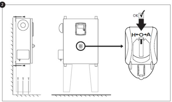
2-Verify that the controller is installed securely on the wall, or optionally on the mounting stand. Verify the Main Selector Switch is in the "OFF" position.
