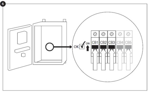
6-Activate all breakers by setting them to the ON position. The controller will boot up for the first time.
