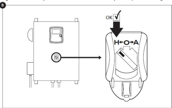
8-Turn the Main Selector Switch in the "HAND" position.
