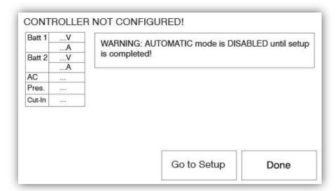
The first Setup must be done prior to using the controller. Completing the First Setup is the only way to access the homepage and enable the automatic mode of the controller. The complete procedure can be found in the "Quick Start-Up Guide" that is available with the controller.
