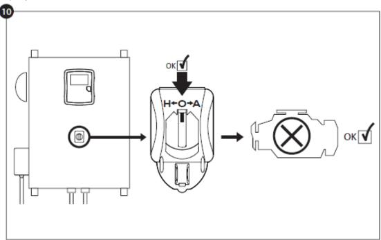
10-Stop the engine by turning the "Main Selector Switch" in the "OFF" position.
