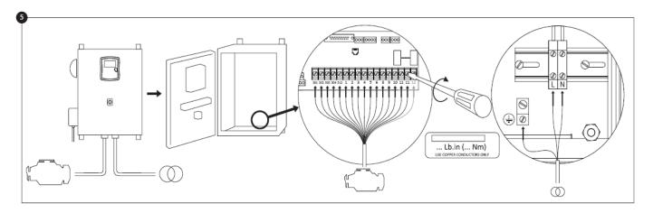
5-Connect all cables between the engine control panel and the controller engine terminal (Identified as "S" on the IO board diagram displayed in the Terminal Strips Descriptions in the manual). Secure with the appropriate torque as indicated on the torque label and verify all connections. Connect the AC main line and ground to the AC terminal in the controller.
