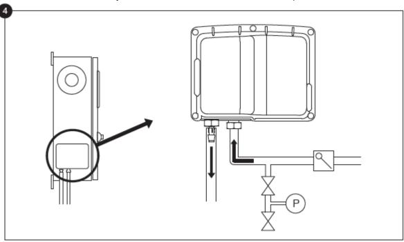
4-Verify and/or install the proper water connections for the water input and the drain. They must be securely installed and tightened. Refer to the silkscreen markings on the plastic cover.
