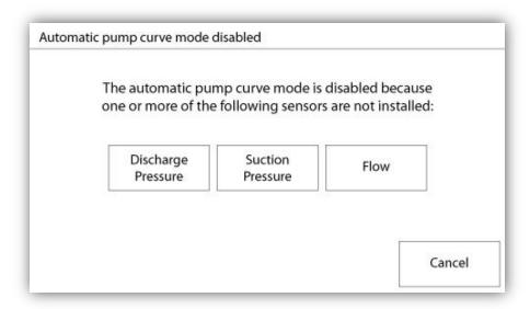
The automatic pump curve was disabled because it needs three sensors installed. The three sensors buttons link to the corresponding sensor page, allowing a quick navigation. If the button is orange, this indicates that this particular sensor is not installed. If the button is blue, it means that this particular sensor is installed. It is always possible to quit the automatic mode by pressing the "Cancel" button.
