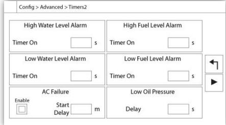
Most common timers for fire pump control can be configured here. Note that any timer set to 0 will remove the delay in the decision process.
