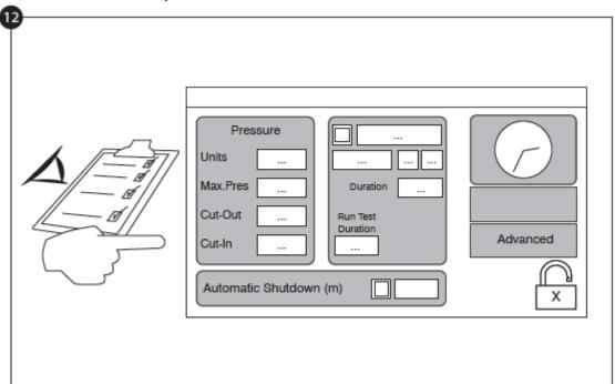
12- Select the controller pressure units, cut-in and cut-out. Verify that all other parameters on the setup page are correct.
