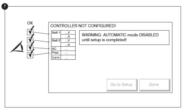
7- The "First Setup" page replaces the Homepage until the "First Setup" is done. Verify that the controller reads the batteries voltage and current. Verify the "AC" is "OK" and not "FAIL". Verify that the pressure reading is correct.
