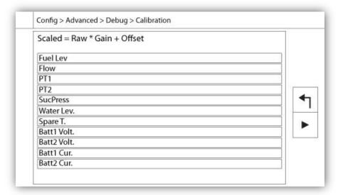
This table displays all calibration parameters. The "Scaled" value is the final calculated value used in the ViZiTouch. It is calculated by multiplying the "Raw" value by the "Gain" coefficient and by adding the "Offset" value. This information is useful when debugging the analog inputs on the IO board.
