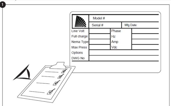
1-The rating label is the most important label. It must be read carefully to ensure the compatibility between the controller and the installation.
