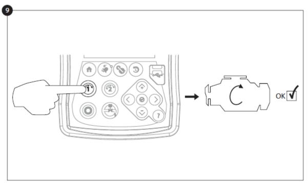
9-Before trying to start the engine, verify that the engine setup is complete and the exhaust pipe is connected properly. Start the engine manually by using the "Crank 1" membrane button. Verify that the engine has started and is running properly.
