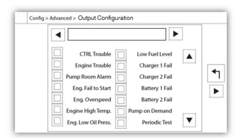
This page allows the configuration of alarm signals on the inputs, and outputs relay signals. Two buttons located far right navigates between the input and output section of the page.
