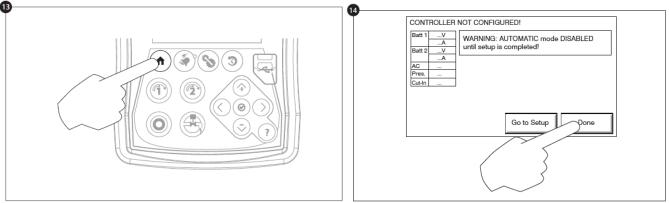
13-14- When satisfied with the controller settings, press the "Home" button on the membrane, acknowledge the changes by pressing the done button. If the done button is unavailable, ensure that a sufficient authorization code has been entered.
