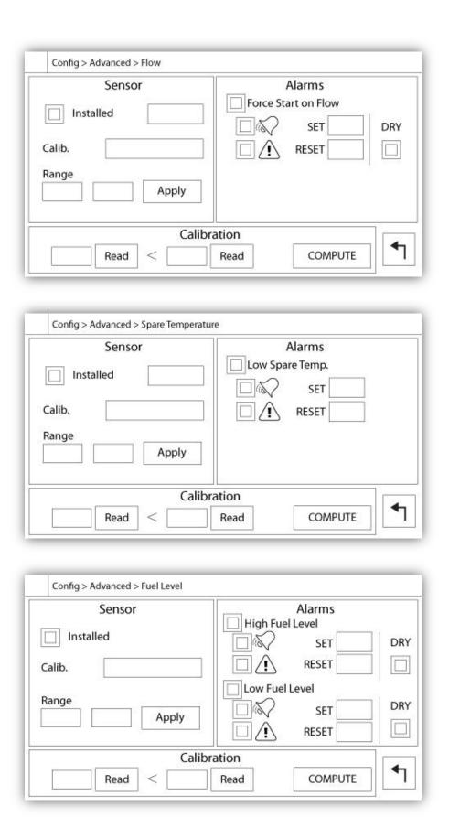
In the ViZiTouch, all sensors refer to analog input connectors on the I/O board. They all have similar settings and configuration.
