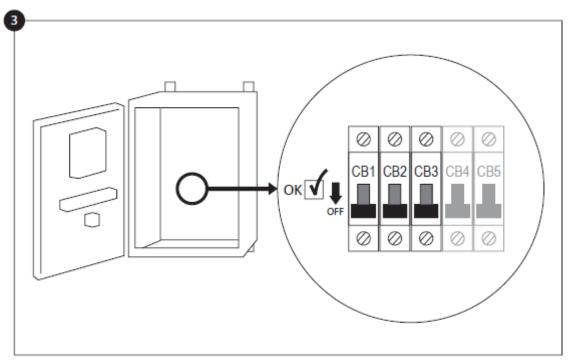
3-Open the controller's door and verify all circuit breakers are in the lower "OFF" position.
