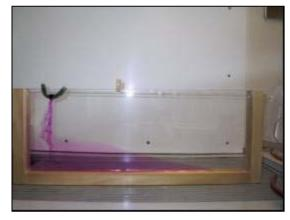
with salt water, a circulation can be created by heating (with a hair-drier) or cooling (ice) the water at certain places in the aquarium. With sponge material easily a submarine topography can be built and fluxes of higher complexity can by studied.
