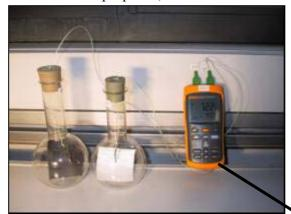
closed with a plug. A thermo sensor measures the temperature inside the flasks. With a strong spotlight. The emission of the white paper is mostly in the short wave range, which passes the glass and escapes. The black paper emits mostly long wave radiation, which cannot transmit through the glass and heats the air inside the flask. Within a short time a significant temperature difference can be measured between the air in the two flasks.
