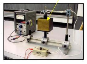
Steal, black painted Aluminium). A Millivac device is connected to a thermo-column. The thermo-column measures the heat irradiation intensity. By turning the Lesslie-cube, the surface exposed to the thermo-column can be changed and thus the infrared emission intensity can be compared. The experiment can quantitatively be evaluated by applying the Stefan-Boltzmann law.
