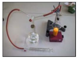
that the syringe can intake air and smoke from a match or a candle, held in front of the open end of the glass tube. Switching the valve again, the smoky air is let in the glass flask. When now the syringe is pulled rapidly the water vapour condensates to fog. The experiment does not work without smoke!
