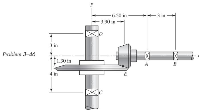
**3–47** Repeat the analysis of Prob. 3–46 for shaft  $AB$ . Let the diameter of the shaft be 1.0 in, and assume that bearing  $A$  is a thrust bearing.
