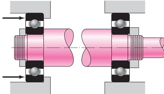
**Figure 11-21**An alternative bearing
