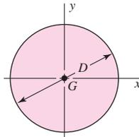
$$A = \frac{\pi D^2}{4} \quad I_x = I_y = \frac{\pi D^4}{64} \quad I_{xy} = 0 \quad J_G = \frac{\pi D^4}{32}$$
