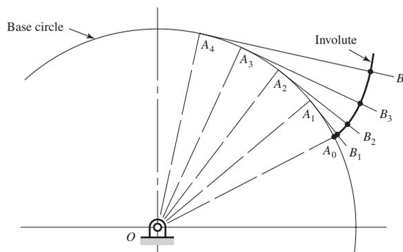
First, it is necessary to learn how to construct an involute curve. As shown in Fig. 13–8, divide the base circle into a number of equal parts, and construct radial lines  $OA_0$ ,  $OA_1$ ,  $OA_2$ , etc. Beginning at  $A_1$ , construct perpendiculars  $A_1B_1$ ,  $A_2B_2$ ,  $A_3B_3$ , etc. Then along  $A_1B_1$  lay off the distance  $A_1A_0$ , along  $A_2B_2$  lay off twice the distance  $A_1A_0$ , etc., producing points through which the involute curve can be constructed.
