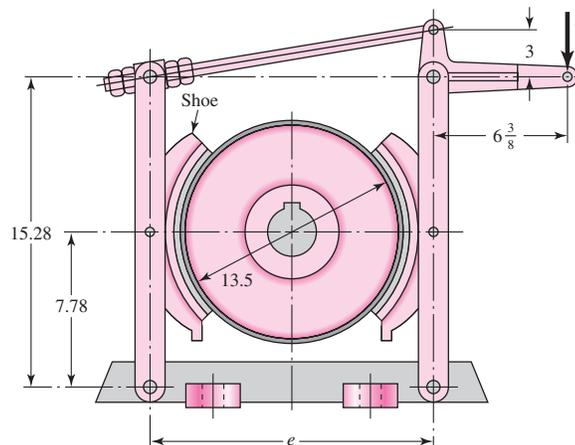
**16-10** Problem 16–9 is preliminary to analyzing the brake. A molded lining is used dry in the brake of Prob. 16–9 on a cast iron drum. The shoes are 7.5 in wide and subtend a  $90^\circ$  arc. Find the actuation force and the braking torque.
