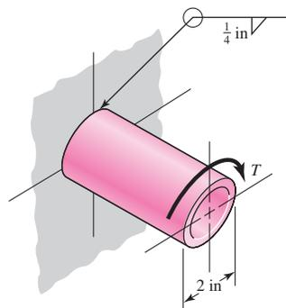
**9-21** Find the maximum shear stress in the throat of the weld metal in the figure.
