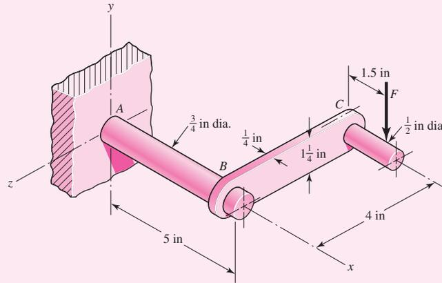
(c) Locate a stress element on the top surface of the shaft at A, and calculate all the stress components that act upon this element.
