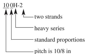
This convention makes the pitch directly readable from the chain number. In Ex. 17–5 ascertain the pitch from the selected chain number and confirm from Table 17–19.
