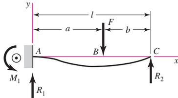
$$R_1 = \frac{Fb}{2l^3}(3l^2 - b^2) \quad R_2 = \frac{Fa^2}{2l^3}(3l - a)$$
