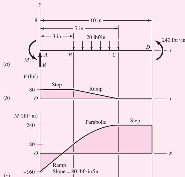
and are not shown in the  $V$  diagram. Also note that both the  $M_1$  and  $240 \text{ lbf} \cdot \text{in}$  moments are counterclockwise and negative singularity functions; however, by the convention shown in Fig. 3–2 the  $M_1$  and  $240 \text{ lbf} \cdot \text{in}$  are negative and positive bending moments, respectively, which is reflected in Fig. 3–6c.
