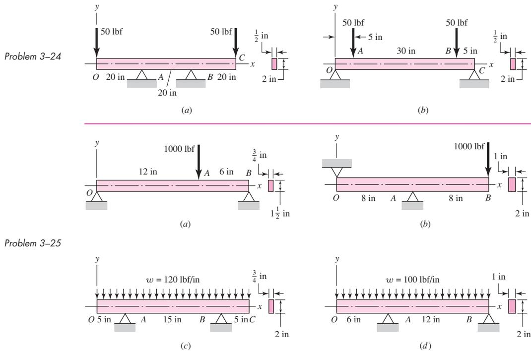
**3–26** The figure illustrates a number of beam sections. Use an allowable bending stress of 1.2 kpsi for wood and 12 kpsi for steel and find the maximum safe uniformly distributed load that each beam can carry if the given lengths are between simple supports.
