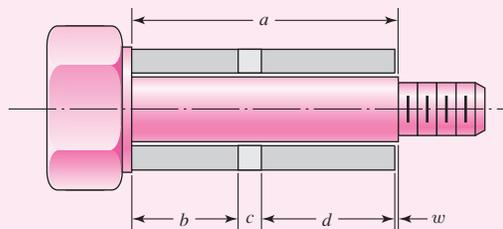
All parts except the part with the dimension  $d$  are supplied by vendors. The part containing the dimension  $d$  is made in-house.
