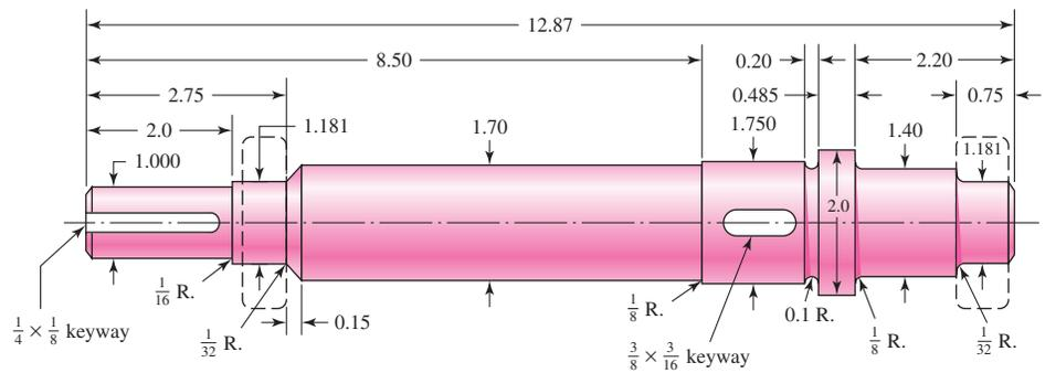
**7-10** An AISI 1020 cold-drawn steel shaft with the geometry shown in the figure carries a transverse load of 7 kN and a torque of 107 N · m. Examine the shaft for strength and deflection. If the largest allowable slope at the bearings is 0.001 rad and at the gear mesh is 0.0005 rad, what
