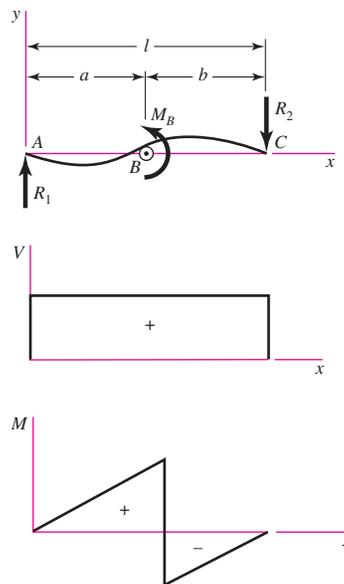
$$R_1 = R_2 = \frac{M_B}{l} \quad V = \frac{M_B}{l}$$
