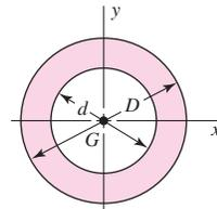
$$A = \frac{\pi}{4}(D^2 - d^2) \quad I_x = I_y = \frac{\pi}{64}(D^4 - d^4) \quad I_{xy} = 0 \quad J_G = \frac{\pi}{32}(D^4 - d^4)$$
