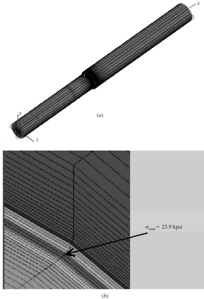
Resorting to another source,<sup>13</sup> the stress concentration factor is found to be  $K_t = 3.00$ . The reaction at the right support is  $R_F = (8/20)600 = 240$  lbf. The bending moment at the start of the fillet is  $M = 240(11.52) = 2765$  lbf · in = 2.765 kip · in. The analytical prediction of the maximum stress is thus
