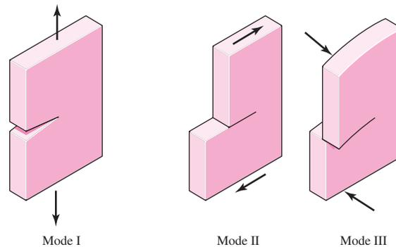
**Crack Modes and the Stress Intensity Factor**
