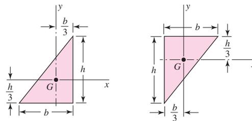
$$A = \frac{bh}{2} \quad I_x = \frac{bh^3}{36} \quad I_y = \frac{b^3h}{36} \quad I_{xy} = \frac{b^2h^2}{72}$$
