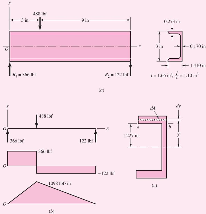
**Solution** The loading, shear-force, and bending-moment diagrams are shown in Fig. 3-19b. If the direct shear force is included in the analysis, the maximum stresses at the top and bottom of the beam will be the same as if only bending were considered. The maximum bending stresses are
