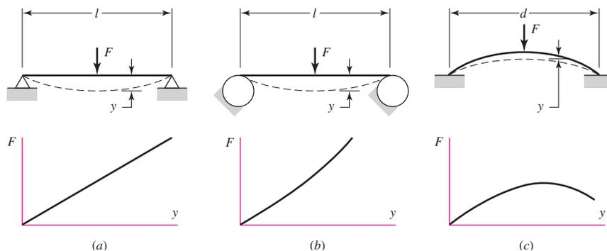
Figure 4–1c is an edge-view of a dish-shaped round disk. The force necessary to flatten the disk increases at first and then decreases as the disk approaches a flat configuration, as shown by the graph. Any mechanical element having such a characteristic is called a *nonlinear softening spring*.
