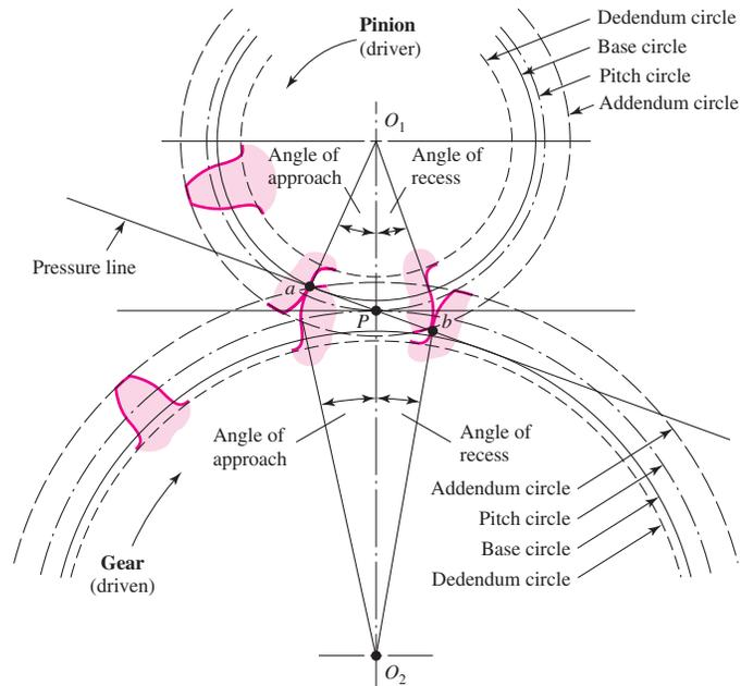
To draw a tooth, we must know the tooth thickness. From Eq. (13-4), the circular pitch is
