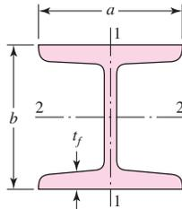
$$A_{0.95\sigma} = \begin{cases} 0.10at_f & \text{axis 1-1} \\ 0.05ba & \text{axis 2-2} \end{cases} \quad t_f > 0.025a$$
