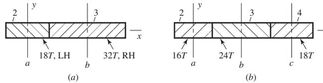
**13–32** This is a continuation of Prob. 13–31. Here, you are asked to find the forces exerted by gears 2 and 3 on their shafts as shown in part *b*. Gear 2 rotates clockwise about the  $y$  axis. Gear 3 is an idler.
