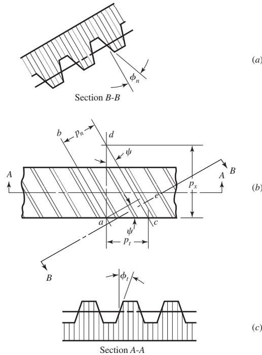
Figure 13–22 represents a portion of the top view of a helical rack. Lines  $ab$  and  $cd$  are the centerlines of two adjacent helical teeth taken on the same pitch plane. The angle  $\psi$  is the *helix angle*. The distance  $ac$  is the *transverse circular pitch*  $p_t$  in the plane of rotation (usually called the *circular pitch*). The distance  $ae$  is the *normal circular pitch*  $p_n$  and is related to the transverse circular pitch as follows:
