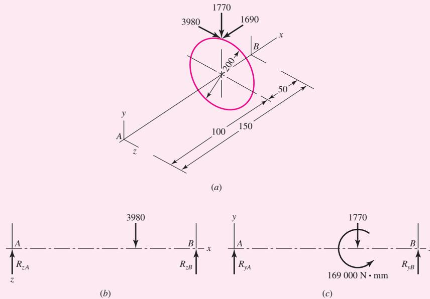
The reactions in the  $xy$  plane from Fig. 11-18c are
