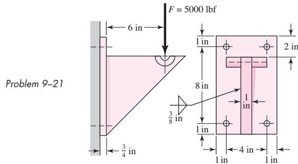
**9-22** The figure shows a welded steel bracket loaded by a static force  $F$ . Estimate the factor of safety if the allowable shear stress in the weld throat is 120 MPa.
