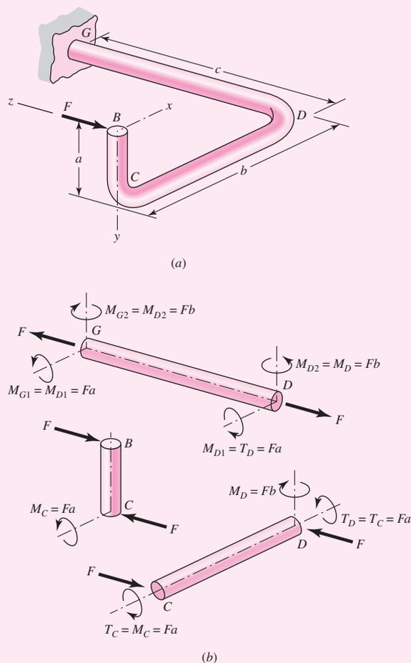
appropriate use of *free-body diagrams* is essential here. The reader should verify that the reactions as functions of  $F$  in elements  $BC$ ,  $CD$ , and  $GD$  are as shown in Fig. 4-11b.
