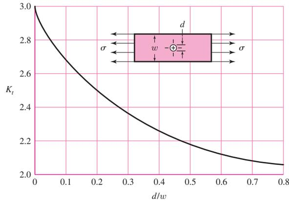
An example is shown in Fig. 3–29, that of a thin plate loaded in tension where the plate contains a centrally located hole.
