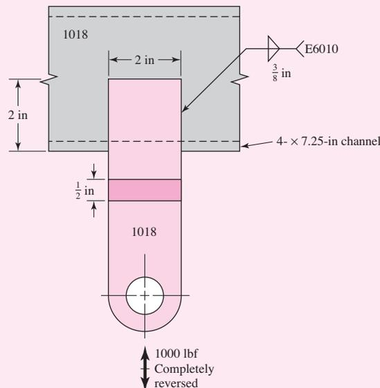
In the absence of a midrange component, the fatigue factor of safety  $n_f$  is given by
