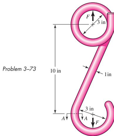
**3-74** The steel eyebolt shown in the figure is loaded with a force  $F$  of 100 lbf. The bolt is formed of  $\frac{1}{4}$ -in-diameter wire to a  $\frac{3}{8}$ -in radius in the eye and at the shank. Estimate the stresses at the inner and outer surfaces at sections A-A and B-B.
