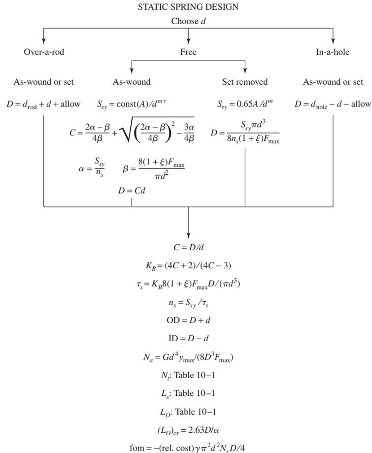
Print or display:  $d, D, C, \text{OD}, \text{ID}, N_a, N_f, L_s, L_0, (L_0)_{\text{cr}}, n_s, \text{fom}$
