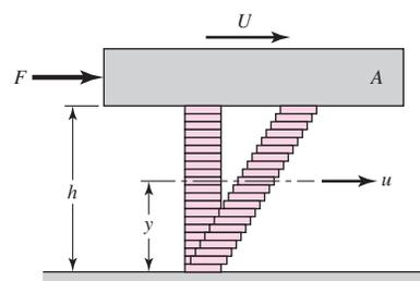
where  $\mu$  is the constant of proportionality and defines *absolute viscosity*, also called *dynamic viscosity*. The derivative  $du/dy$  is the rate of change of velocity with distance and may be called the rate of shear, or the velocity gradient. The viscosity  $\mu$  is thus a measure of the internal frictional resistance of the fluid. For most lubricating fluids, the rate of shear is constant, and  $du/dy = U/h$ . Thus, from Eq. (12–1),
