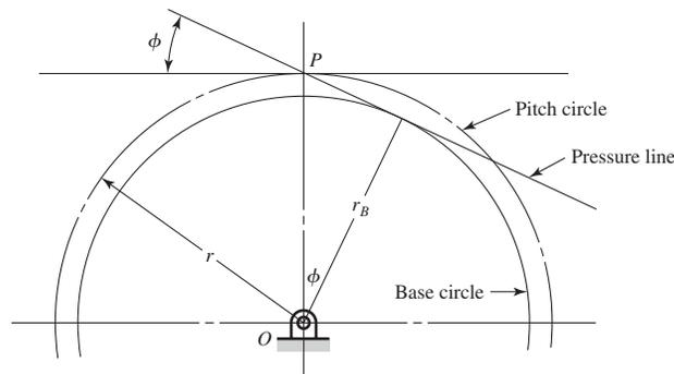
Next, on each gear draw a circle tangent to the pressure line. These circles are the *base circles*. Since they are tangent to the pressure line, the pressure angle determines their size. As shown in Fig. 13-10, the radius of the base circle is
