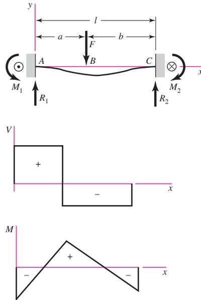
$$R_1 = \frac{Fb^2}{l^3}(3a + b) \quad R_2 = \frac{Fa^2}{l^3}(3b + a)$$
