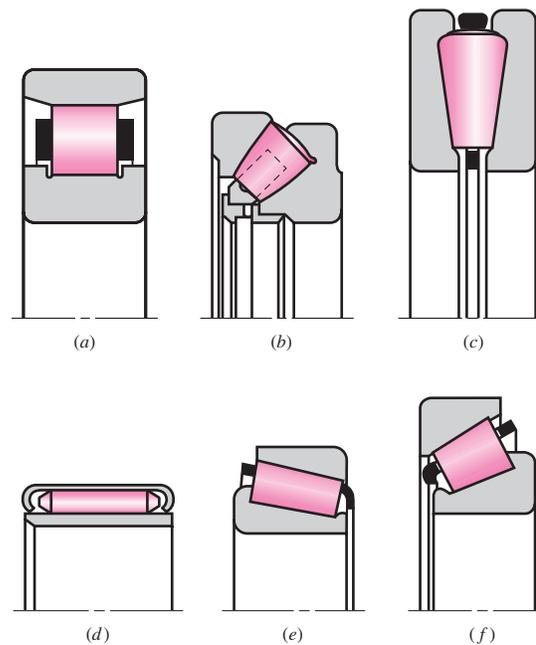
The spherical-roller thrust bearing (Fig. 11–3*b*) is useful where heavy loads and misalignment occur. The spherical elements have the advantage of increasing their contact area as the load is increased.
