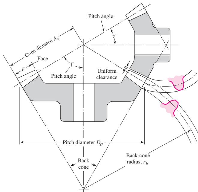
where the subscripts  $P$  and  $G$  refer to the pinion and gear, respectively, and where  $\gamma$  and  $\Gamma$  are, respectively, the pitch angles of the pinion and gear.
