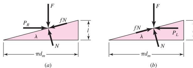
In Fig. 8-5 a square-threaded power screw with single thread having a mean diameter  $d_m$ , a pitch  $p$ , a lead angle  $\lambda$ , and a helix angle  $\psi$  is loaded by the axial compressive force  $F$ . We wish to find an expression for the torque required to raise this load, and another expression for the torque required to lower the load.
