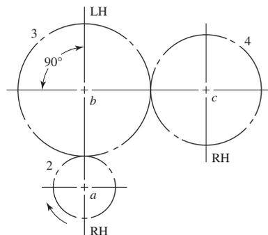
**13–36** The figure shows a double-reduction helical gearset. Pinion 2 is the driver, and it receives a torque of 1200 lbf · in from its shaft in the direction shown. Pinion 2 has a normal diametral pitch of 8 teeth/in, 14 teeth, and a normal pressure angle of  $20^\circ$  and is cut right-handed with a helix angle
