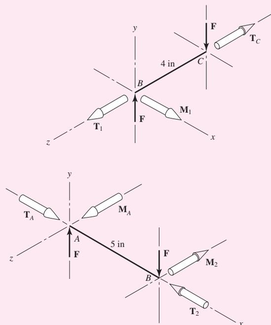
(b) For arm  $BC$ , the bending moment will reach a maximum near the shaft at  $B$ . If we assume this is  $1200 \text{ lbf} \cdot \text{in}$ , then the bending stress for a rectangular section will be
