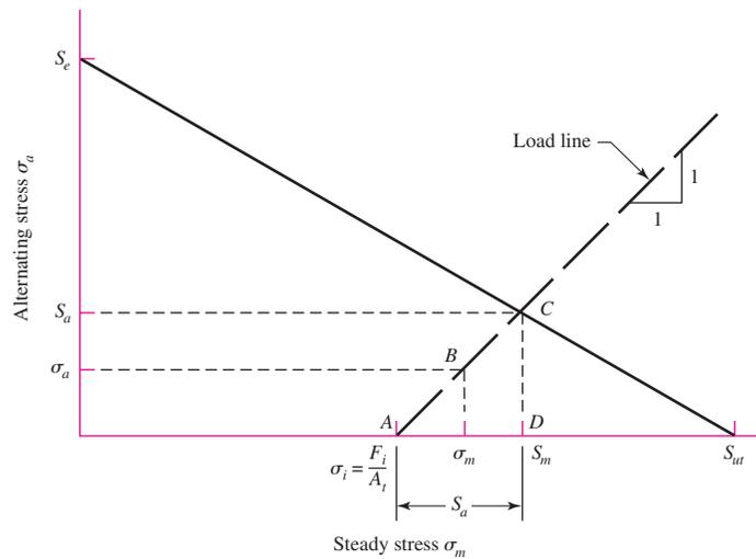
maximum force  $P$ . This would be the situation in a pressure cylinder, for example, where a pressure either exists or does not exist. For such cases,  $F_{\max} = F_b$  and  $F_{\min} = F_i$  and the alternating component of the force is  $F_a = (F_{\max} - F_{\min})/2 = (F_b - F_i)/2$ . Dividing this by  $A_t$  yields the alternating component of the bolt stress. Employing the notation from Sec. 8-7 with Eq. (8-24), we obtain
