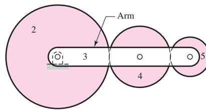
Figure 13–31 shows a planetary train composed of a sun gear 2, an arm or carrier 3, and planet gears 4 and 5. The angular velocity of gear 2 relative to the arm in rev/min is
