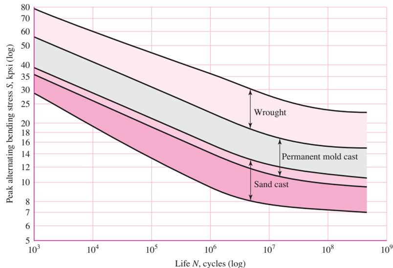
The ordinate of the  $S$ - $N$  diagram is called the *fatigue strength*  $S_f$ ; a statement of this strength value must always be accompanied by a statement of the number of cycles  $N$  to which it corresponds.
