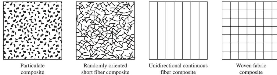
epoxy resin reinforced with continuous graphite fibers will have very high strength and stiffness in the direction of the fibers, but very low properties normal or transverse to the fibers. For this reason, structures of composite materials are normally constructed of multiple plies (laminates) where each ply is oriented to achieve optimal structural stiffness and strength performance.
