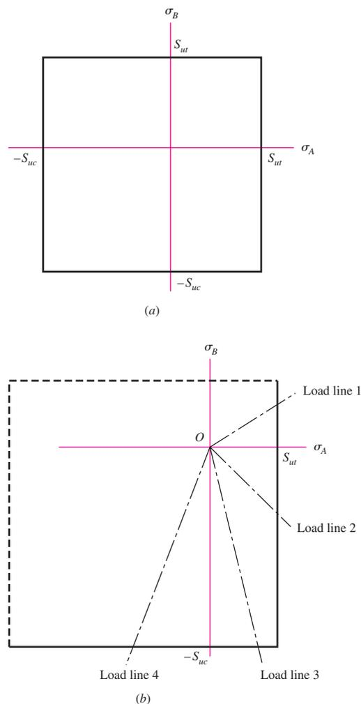
$$\begin{aligned} \sigma_A = \frac{S_{ut}}{n} \quad \sigma_A \geq \sigma_B \geq 0 & \quad \text{Load line 1} \\ \sigma_A \geq 0 \geq \sigma_B \quad \text{and} \quad \left| \frac{\sigma_B}{\sigma_A} \right| \leq \frac{S_{uc}}{S_{ut}} & \quad \text{Load line 2} \end{aligned} \quad (5-30a)$$
