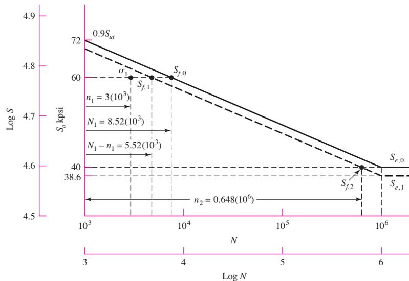
Figure 6–34 shows that the material has a life  $N_1 = 8520$  cycles at 60 kpsi, and consequently, after the application of  $\sigma_1$  for 3000 cycles, there are  $N_1 - n_1 = 5520$  cycles of life remaining at  $\sigma_1$ . This locates the finite-life strength  $S_{f,1}$  of the damaged material, as shown in Fig. 6–34. To get a second point, we ask the question: With  $n_1$  and  $N_1$  given, how many cycles of stress  $\sigma_2 = S'_{e,0}$  can be applied before the damaged material fails?
