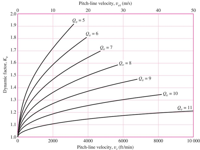
allowance for the effect of gear-tooth quality related to speed and load, and the increase in stress that follows. AGMA uses a *transmission accuracy number*  $Q_v$  to describe the precision with which tooth profiles are spaced along the pitch circle. Figure 15–5 shows graphically how pitch-line velocity and transmission accuracy number are related to the dynamic factor  $K_v$ . Curve fits are
