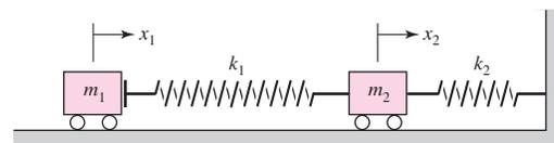
only in a solution up to the point in time for which  $x_2$  reaches a maximum. That is, the solution for the rebound isn't needed. The differential equations are not difficult to derive. They are
