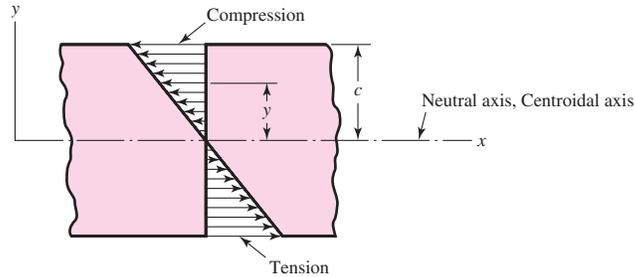
The bending stress varies linearly with the distance from the neutral axis,  $y$ , and is given by
