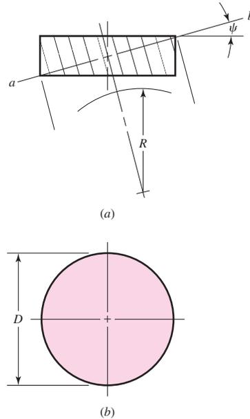
increases until, when  $\psi = 90^\circ$ ,  $R = \infty$ . The radius  $R$  is the apparent pitch radius of a helical-gear tooth when viewed in the direction of the tooth elements. A gear of the same pitch and with the radius  $R$  will have a greater number of teeth, because of the increased radius. In helical-gear terminology this is called the *virtual number of teeth*. It can be shown by analytical geometry that the virtual number of teeth is related to the actual number by the equation
