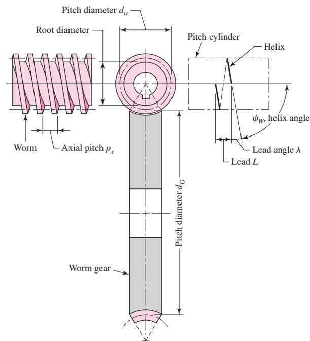
Since it is not related to the number of teeth, the worm may have any pitch diameter; this diameter should, however, be the same as the pitch diameter of the hob used to cut the worm-gear teeth. Generally, the pitch diameter of the worm should be selected so as to fall into the range
