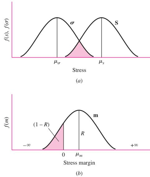
$1 - R$  where parts are expected to fail. We next consider some typical cases involving stress-strength interference.
