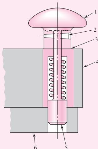
Since the pull knob must be raised  $\frac{3}{4}$  in for indexing and the space for the spring is  $1\frac{3}{8}$  in long when the pin is down, the solid length cannot be more than  $\frac{5}{8}$  in.
