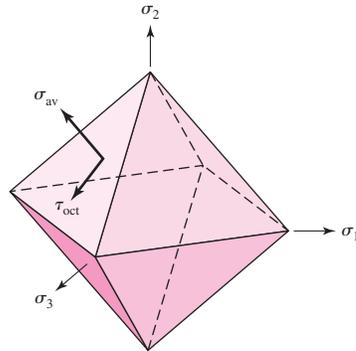
Under the name of the octahedral-shear-stress theory, *failure is assumed to occur whenever the octahedral shear stress for any stress state equals or exceeds the octahedral shear stress for the simple tension-test specimen at failure.*
