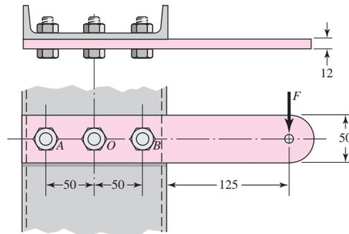
**8-49** Find the total shear load on each of the three bolts for the connection shown in the figure and compute the significant bolt shear stress and bearing stress. Find the second moment of area of the 8-mm plate on a section through the three bolt holes, and find the maximum bending stress in the plate.
