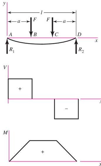
$$R_1 = R_2 = F \quad V_{AB} = F \quad V_{BC} = 0$$
