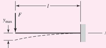
**Solution** At any point  $x$  along the beam, the moment is  $M = -Fx$ . Substituting this value of  $M$  into Eq. (4-18), we find
