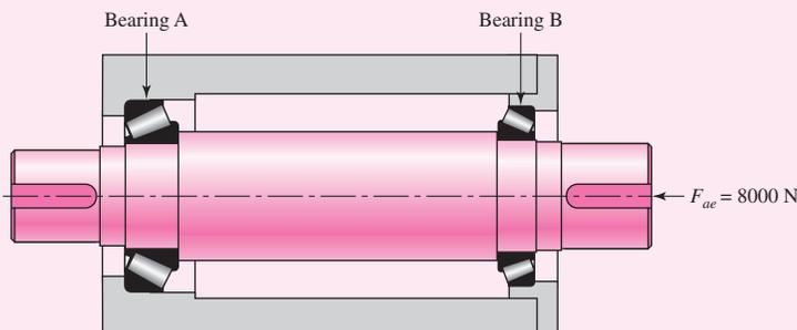
Noting that  $F_{ae}$  to the right is positive (Table 11-6), with direct mounting  $m = +1$ , we can write
