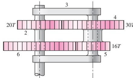
**13–21** In the gear train of Prob. 13–20, let gear 2 be driven at 180 rev/min counterclockwise while gear 6 is held stationary. What is the speed and direction of rotation of the arm?
