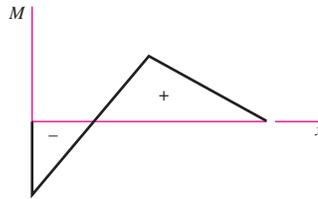
12 One fixed and one simple support—intermediate load
