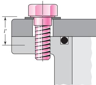
A section through a tension-loaded bolted joint is illustrated in Fig. 8-13. Notice the clearance space provided by the bolt holes. Notice, too, how the bolt threads extend into the body of the connection.
