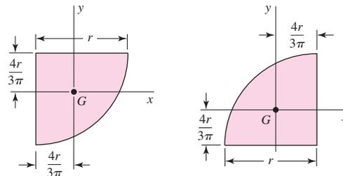
$$A = \frac{\pi r^2}{4} \quad I_x = I_y = r^4 \left( \frac{\pi}{16} - \frac{4}{9\pi} \right) \quad I_{xy} = r^4 \left( \frac{4}{9\pi} - \frac{1}{8} \right)$$
