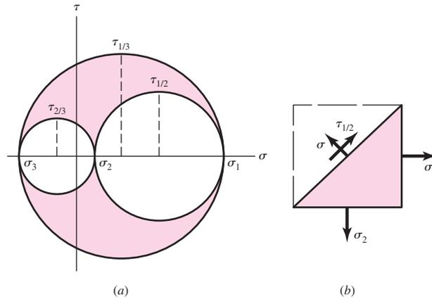
stress components  $\sigma_x$ ,  $\sigma_y$ ,  $\sigma_z$ ,  $\tau_{xy}$ ,  $\tau_{yz}$ , and  $\tau_{zx}$ , involves finding the roots of the cubic equation<sup>1</sup>
