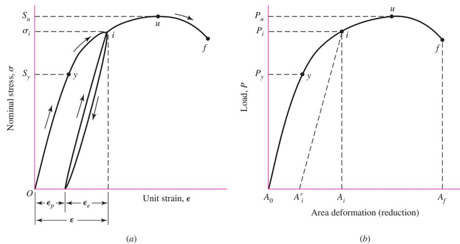
the amount  $\epsilon_e$ . Thus at point  $i$  the total unit strain consists of the two components  $\epsilon_p$  and  $\epsilon_e$  and is given by the equation
