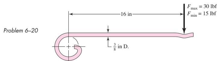
that the surface finish corresponds closely to a hot-rolled finish. What number of applications is likely to cause failure? Solve using:
