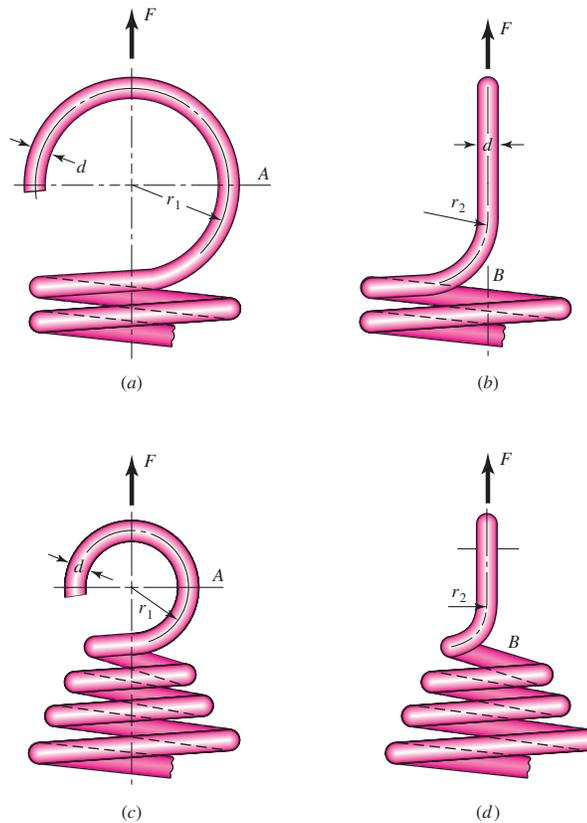
Note: Radius  $r_1$  is in the plane of the end coil for curved beam bending stress. Radius  $r_2$  is at a right angle to the end coil for torsional shear stress.
