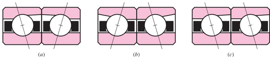
Figure 11-23 shows another two-bearing mounting. Note the use of washers against the cone backs.
