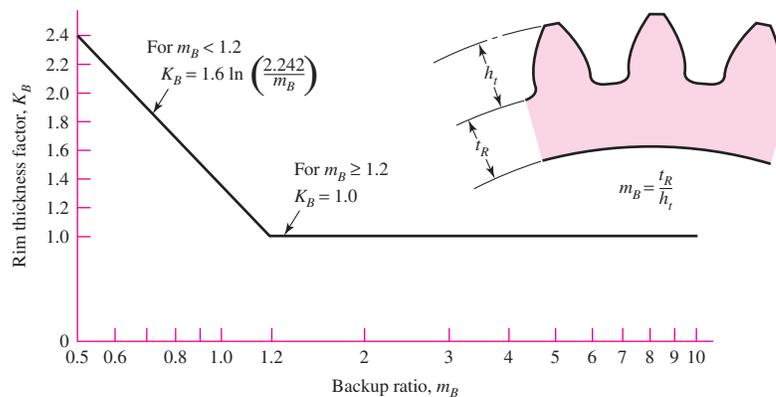
Figure 14–16 also gives the value of  $K_B$  graphically. The rim-thickness factor  $K_B$  is applied in addition to the 0.70 reverse-loading factor when applicable.
