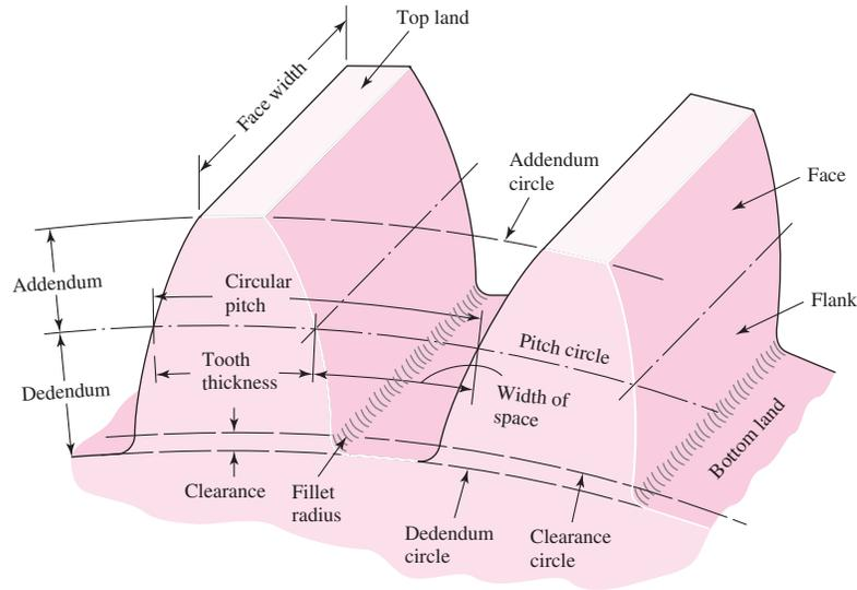
The *module*  $m$  is the ratio of the pitch diameter to the number of teeth. The customary unit of length used is the millimeter. The module is the index of tooth size in SI.
