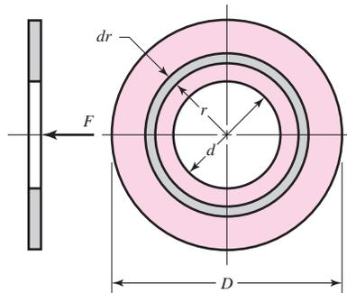
single-plate disk clutch; a multiple-disk clutch-brake is shown in Fig. 16–15. Let us now determine the capacity of such a clutch or brake in terms of the material and geometry.
