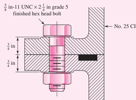
From Table A–17 the next fraction size bolt is  $L = 2\frac{1}{4}$  in. From Eq. (8–13), the thread length is  $L_T = 2(0.625) + 0.25 = 1.50$  in. Thus the length of the unthreaded portion in the grip is  $l_d = 2.25 - 1.50 = 0.75$  in. The threaded length in the grip is  $l_t = l - l_d = 0.75$  in. From Table 8–2,  $A_t = 0.226$  in<sup>2</sup>. The major-diameter area is  $A_d = \pi(0.625)^2/4 = 0.3068$  in<sup>2</sup>. The bolt stiffness is then
