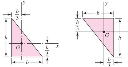
$$A = \frac{bh}{2} \quad I_x = \frac{bh^3}{36} \quad I_y = \frac{b^3h}{36} \quad I_{xy} = \frac{-b^2h^2}{72}$$
