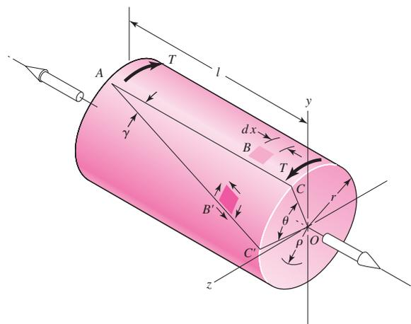
Shear stresses develop throughout the cross section. For a round bar in torsion, these stresses are proportional to the radius  $\rho$  and are given by
