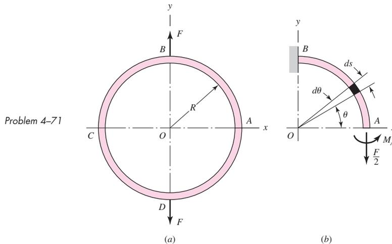
**4-72** Find the increase in the diameter of the ring of Prob. 4-71 due to the forces  $F$  and along the  $y$  axis.
