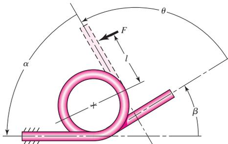
where  $N_p$  is the number of partial turns. The above equation means that  $N_b$  takes on noninteger, discrete values such as 5.3, 6.3, 7.3, . . . , with successive differences of 1 as possibilities in designing a specific spring. This consideration will be discussed later.
