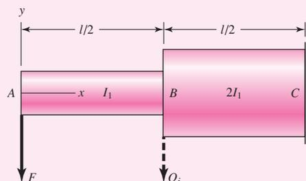
$$\delta_A = \frac{\partial U}{\partial F} = \int_0^l \frac{1}{EI} \left( M \frac{\partial M}{\partial F} \right) dx \quad (2)$$
