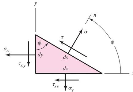
Equation (3–10) defines two particular values for the angle  $2\phi_p$ , one of which defines the maximum normal stress  $\sigma_1$  and the other, the minimum normal stress  $\sigma_2$ . These two stresses are called the *principal stresses*, and their corresponding directions, the *principal directions*. The angle between the principal directions is  $90^\circ$ . It is important to note that Eq. (3–10) can be written in the form
