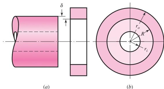
With  $p$ , Eq. (3–49) can be used to determine the radial and tangential stresses in each member. For the inner member,  $p_o = p$  and  $p_i = 0$ . For the outer member,  $p_o = 0$  and  $p_i = p$ . For example, the magnitudes of the tangential stresses at the transition radius  $R$  are maximum for both members. For the inner member
