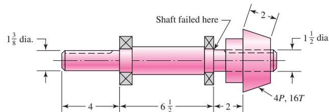
**7–14** A 1-in-diameter uniform steel shaft is 24 in long between bearings.
