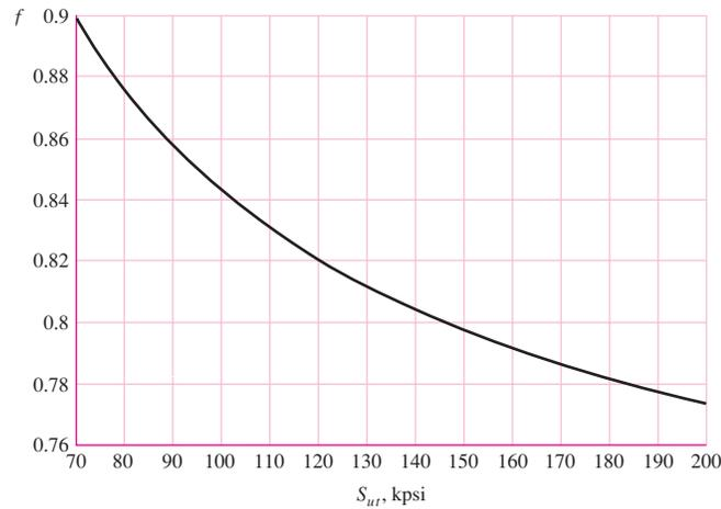
The process given for finding  $f$  can be repeated for various ultimate strengths. Figure 6-18 is a plot of  $f$  for  $70 \leq S_{ut} \leq 200$  kpsi. To be conservative, for  $S_{ut} < 70$  kpsi, let  $f = 0.9$ .
