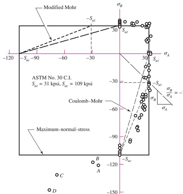
stress conditions, with several brittle failure hypotheses shown, superposed. We note the following:
