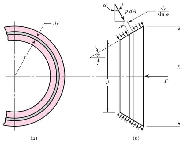
cone angle is too small, say, less than about  $8^\circ$ , then the force required to disengage the clutch may be quite large. And the wedging effect lessens rapidly when larger cone angles are used. Depending upon the characteristics of the friction materials, a good compromise can usually be found using cone angles between  $10$  and  $15^\circ$ .
