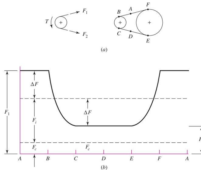
Figure 17-12 illustrates the variation of flexible flat-belt tensions at some cardinal points during a belt pass.
