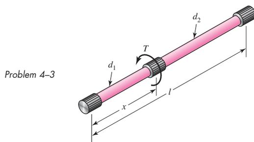
**4-4** An engineer is forced by geometric considerations to apply the torque on the spring of Prob. 4-3 at the location  $x = 0.2l$ . For a uniform-diameter spring, this would cause the long leg of the span to be underutilized when both legs have the same diameter. If the diameter of the long leg is reduced sufficiently, the shear stress in the two legs can be made equal. How would this change affect the allowable angle of twist, the largest torque, and the spring rate?
