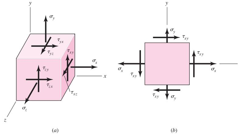
dimensions of the cube in Fig. 3–8a approach zero, the stresses on the hidden faces become equal and opposite to those on the opposing visible faces. Thus, in general, a complete state of stress is defined by nine stress components,  $\sigma_x$ ,  $\sigma_y$ ,  $\sigma_z$ ,  $\tau_{xy}$ ,  $\tau_{xz}$ ,  $\tau_{yx}$ ,  $\tau_{yz}$ ,  $\tau_{zx}$ , and  $\tau_{zy}$ .
