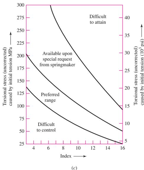
$L_0$  and  $F_i$  is the initial tension in the spring that must be exceeded before the spring deflects. The load-deflection relation is then
