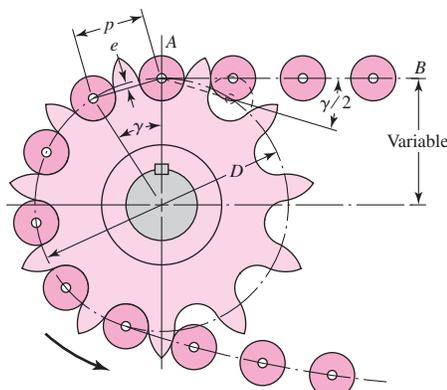
rollers and the sprocket teeth and also wear in the chain joint. Since the life of a properly selected drive is a function of the wear and the surface fatigue strength of the rollers, it is important to reduce the angle of articulation as much as possible.
