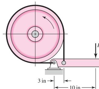
**16-15** The figure shows a band brake designed to prevent “backward” rotation of the shaft. The angle of wrap is  $270^\circ$ , the band width is  $2\frac{1}{8}$  in, and the coefficient of friction is 0.20. The torque to be resisted by the brake is 150 lbf · ft. The diameter of the pulley is  $8\frac{1}{4}$  in.
