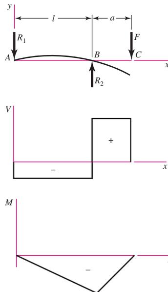
$$R_1 = \frac{Fa}{l} \quad R_2 = \frac{F}{l}(l+a)$$
