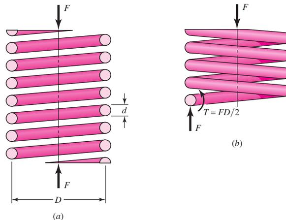
at the *inside* fiber of the spring. Substitution of  $\tau_{\max} = \tau$ ,  $T = FD/2$ ,  $r = d/2$ ,  $J = \pi d^4/32$ , and  $A = \pi d^2/4$  gives
