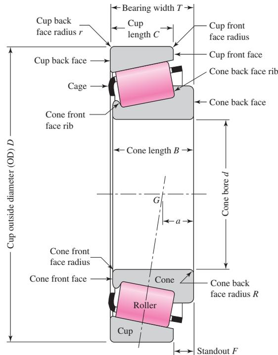
A radial load will induce a thrust reaction. The *load zone* includes about half the rollers and subtends an angle of approximately  $180^\circ$ . Using the symbol  $F_{a(180)}$  for the induced thrust load from a radial load with a  $180^\circ$  load zone, Timken provides the equation
