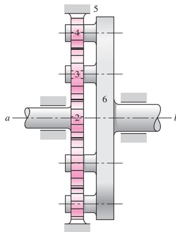
**13–23** The tooth numbers for the gear train illustrated are  $N_2 = 24$ ,  $N_3 = 18$ ,  $N_4 = 30$ ,  $N_6 = 36$ , and  $N_7 = 54$ . Gear 7 is fixed. If shaft  $b$  is turned through 5 revolutions, how many turns will shaft  $a$  make?
