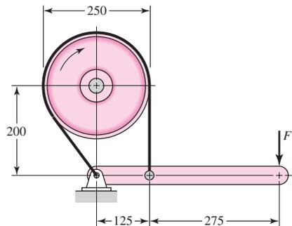
**16-14** The figure depicts a band brake whose drum rotates counterclockwise at 200 rev/min. The drum diameter is 16 in and the band lining 3 in wide. The coefficient of friction is 0.20. The maximum lining interface pressure is 70 psi.
