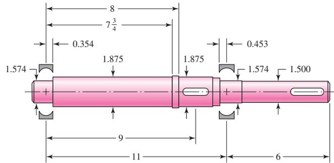
**7-9** The shaft shown in the figure is driven by a gear at the right keyway, drives a fan at the left keyway, and is supported by two deep-groove ball bearings. The shaft is made from AISI 1020 cold-drawn steel. At steady-state speed, the gear transmits a radial load of 230 lbf and a tangential load of 633 lbf at a pitch diameter of 8 in.
