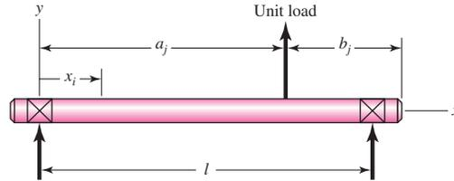
Computer assistance is often used to lessen the difficulty in finding transverse deflections of a stepped shaft. Rayleigh's equation overestimates the critical speed.
