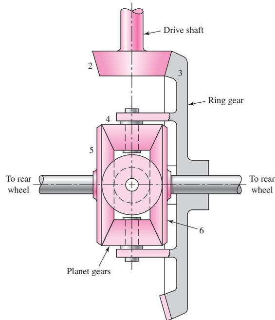
(c) Suppose, with a rear-wheel drive vehicle, the auto is parked with the right wheel resting on a wet icy surface. Does the answer to part (b) give you any hint as to what would happen if you started the car and attempted to drive on?
