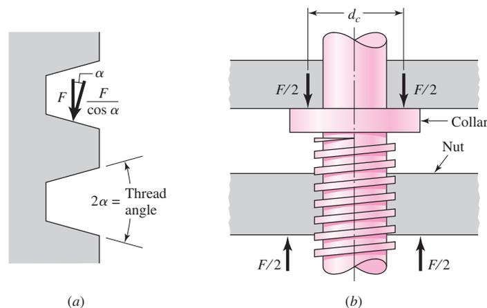
Nominal body stresses in power screws can be related to thread parameters as follows. The maximum nominal shear stress  $\tau$  in torsion of the screw body can be expressed as
