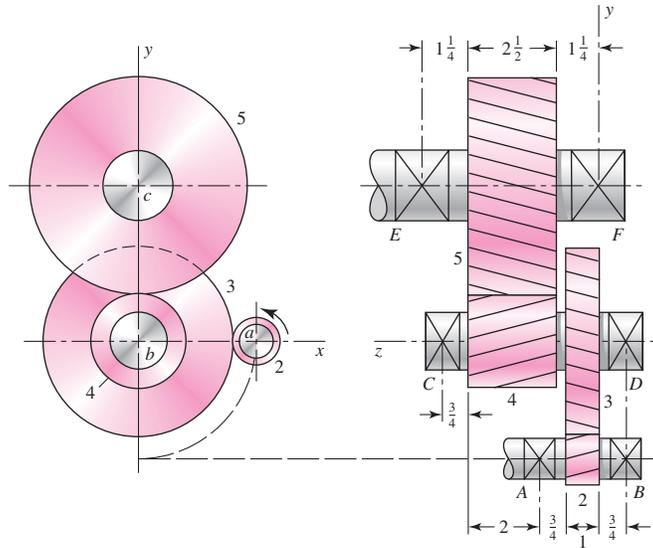
normal pressure angle of  $20^\circ$ . The second pair of gears in the train, gears 4 and 5, have a normal diametral pitch of 6 teeth/in, a  $25^\circ$  helix angle, and a normal pressure angle of  $20^\circ$ . The tooth numbers are:  $N_2 = 14$ ,  $N_3 = 54$ ,  $N_4 = 16$ ,  $N_5 = 36$ . Find:
