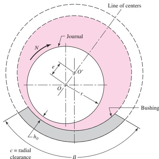
Fig. 12–6 the center of the journal is at  $O$  and the center of the bearing at  $O'$ . The distance between these centers is the *eccentricity* and is denoted by  $e$ . The *minimum film thickness* is designated by  $h_0$ , and it occurs at the line of centers. The film thickness at any other point is designated by  $h$ . We also define an *eccentricity ratio*  $\epsilon$  as
