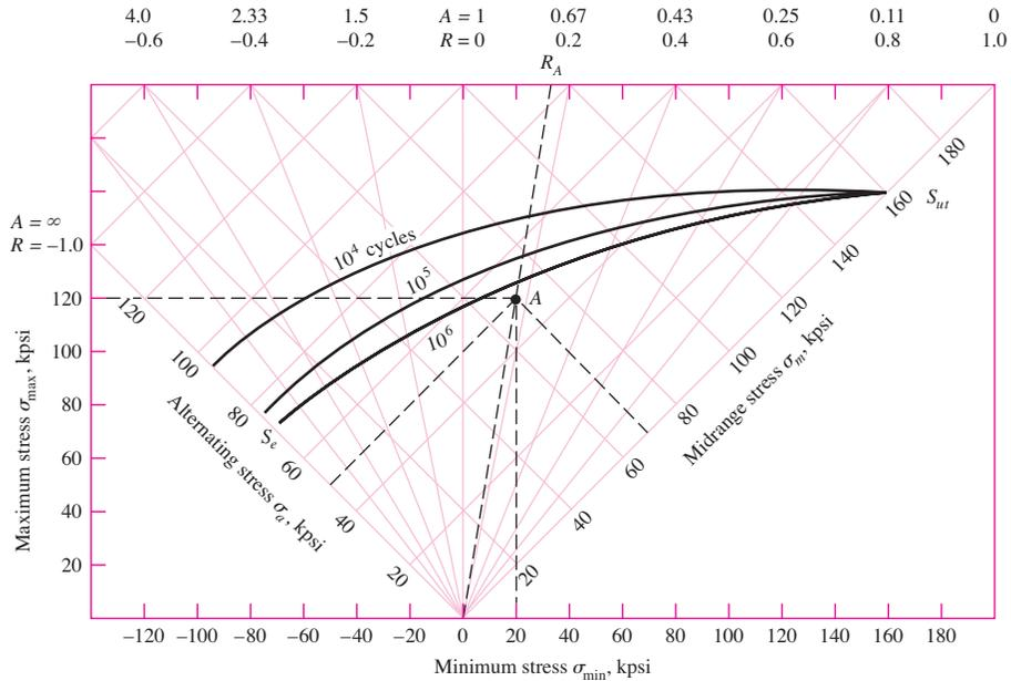
have been drawn too. Any stress state, such as the one at A, can be described by the minimum and maximum components, or by the midrange and alternating components. And safety is indicated whenever the point described by the stress components lies below the constant-life line.
