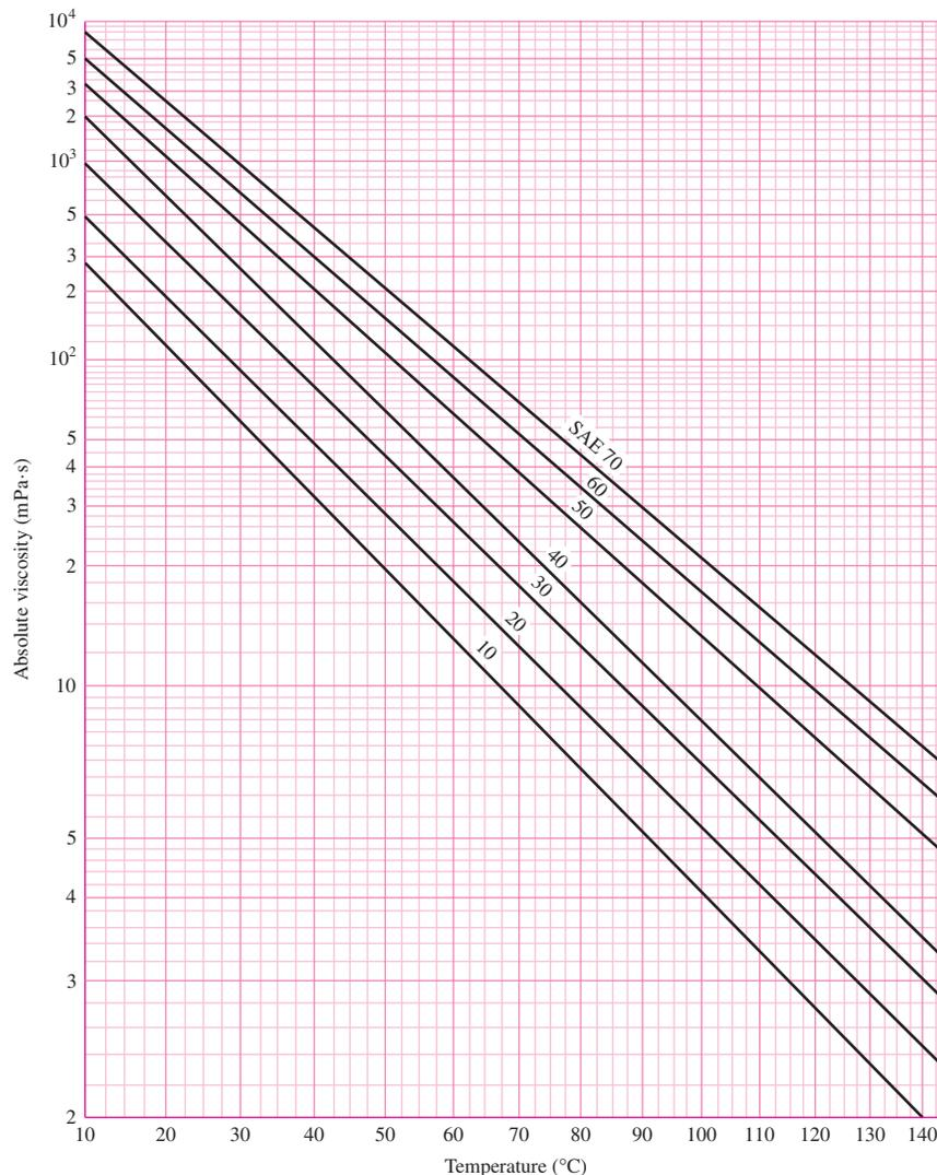
This corresponds to point *A* on Fig. 12-12, which is above the SAE 30 line and indicates that the viscosity used in the analysis was too high.
