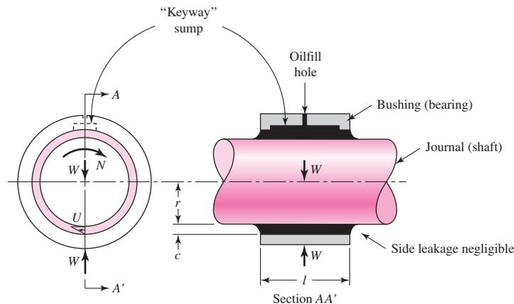
the radial clearance by  $c$ , and the length of the bearing by  $l$ , all dimensions being in inches. If the shaft rotates at  $N$  rev/s, then its surface velocity is  $U = 2\pi rN$  in/s. Since the shearing stress in the lubricant is equal to the velocity gradient times the viscosity, from Eq. (12-2) we have
