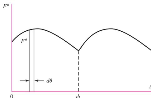
An example of this would be a cam whose bearings rotate with the cam through the angle  $d\theta$ . The total damage during a complete cam rotation is given by
