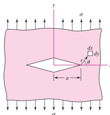
The stress  $\sigma_y$  near the tip, with  $\theta = 0$ , is
