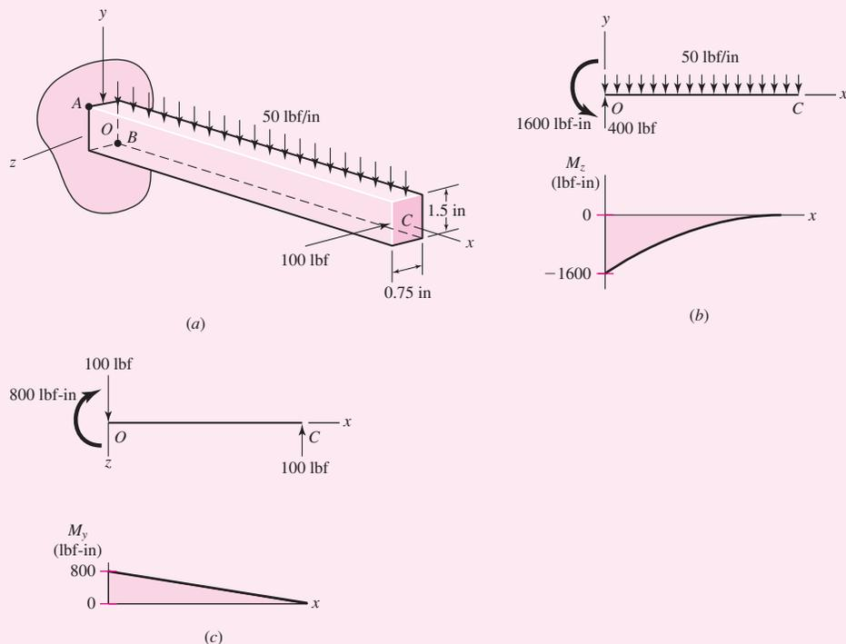
(a) For the cross section shown determine the maximum tensile and compressive bending stresses and where they act.
