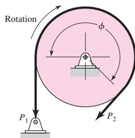
**16-12** The drum for the band brake in Prob. 16-11 is 300 mm in diameter. The band selected has a mean coefficient of friction of 0.28 and a width of 80 mm. It can safely support a tension of 7.6 kN. If the angle of wrap is  $270^\circ$ , find the lining pressure and the torque capacity.
