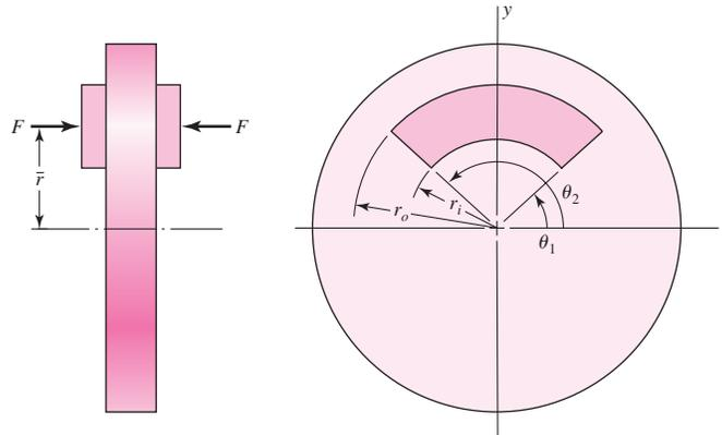
of a rotating disk. Depicted in Fig. 16–19 is the geometry of an annular-pad brake contact area. The governing axial wear equation is Eq. (12–27), p. 643,
