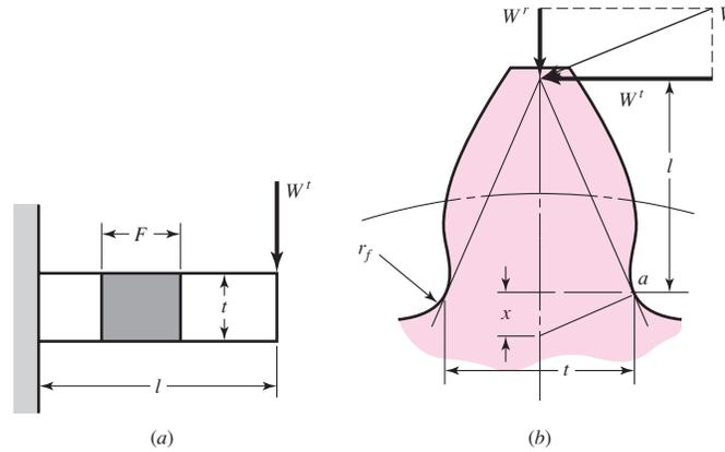
Referring now to Fig. 14-1b, we assume that the maximum stress in a gear tooth occurs at point  $a$ . By similar triangles, you can write
