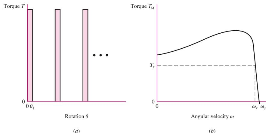
continuously, creating a punching rhythm, or it can be connected on command through a clutch that allows one punch and a disconnect. The motor and flywheel must be sized for the most demanding service, which is steady punching. The work done is given by
