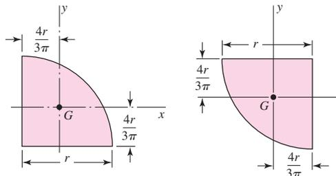
$$A = \frac{\pi r^2}{4} \quad I_x = I_y = r^4 \left( \frac{\pi}{16} - \frac{4}{9\pi} \right) \quad I_{xy} = r^4 \left( \frac{1}{8} - \frac{4}{9\pi} \right)$$
