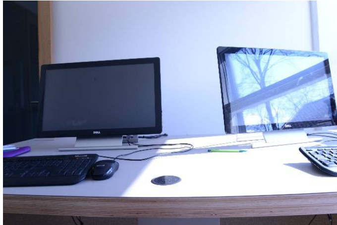
Figure 6.9 Veiling reflection caused by sun beams entering the room. The picture refers to room R5209 but the same phenomenon occurs in each room.
