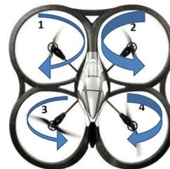
**Fig5. Move towards low speed motors**
