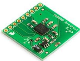
Image.3.2. Gyro breakout board
