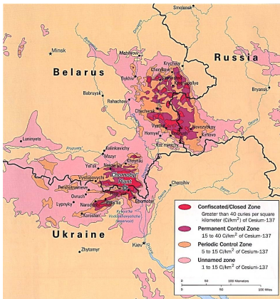
w/ A map showing levels of radiation near the site of the Chernobyl disaster. At the boundary of the most highly contaminated (bright red) areas, people would be exposed to about 1300 millirem per year, or about four times the natural background level. In the pink areas, which are still densely populated, the exposure is comparable to the natural level found in a high-altitude city such as Denver.
